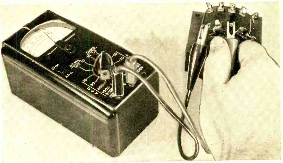
Fig. 1. The correct way to use an ohmmeter to identify transformer terminal connections.
