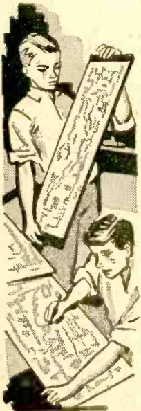
This printed circuit section represents approximately 50 per-cent of the complete chassis and is produced by automatic machines. Result is lower cost TV set.
