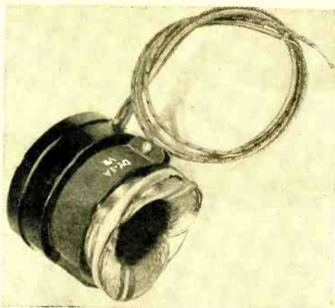
Fig. 5. The photograph shows a typical deflection yoke of a modern TV receiver.
