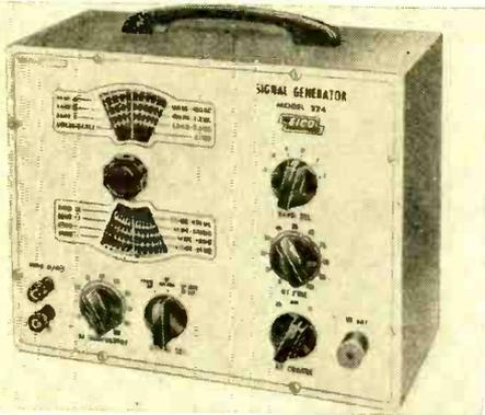
It can be used for i.f.-r.f. alignment; signal tracing; troubleshooting of AM, FM, and TV receivers; as a marker generator for alignment of new high frequency as well as older low frequency TV i.f.'s; and for 400-cycle sine wave audio testing.
