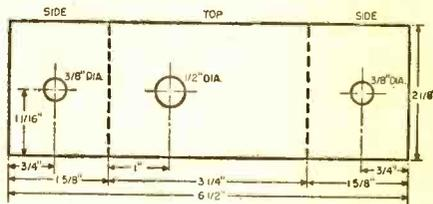
Dimensional diagram of the Bud "Minibox" showing the holes for the a.c. line, battery leads, and the "on-off" toggle switch.
