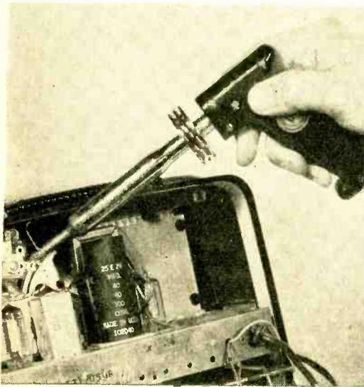
← If components fastened to the cabinet prevent the chassis from being taken out, they must be removed. If unsoldering is necessary, perform the operation very carefully to avoid damaging components. Here two wires are unsoldered from an adjustable capacitor across a built-in loop antenna.
