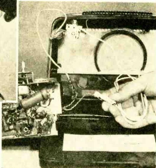
After chassis has been removed from → the cabinet, use a pair of flexible wire leads to connect the radio lead-in wires temporarily to built-in loop antenna. The chassis may be "hot" to ground, depending upon power plug polarity. Before attempting any repairs, check for presence of a.c. voltage between chassis and ground. If any voltage is detected, reverse the power plug.
