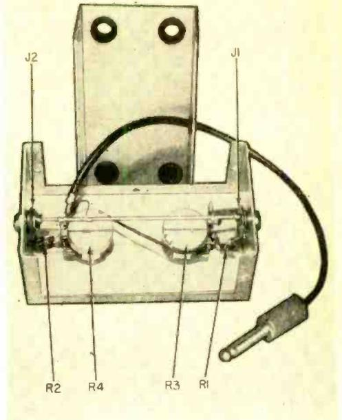
Underchassis view of mixer (above, right). Exact position of the two potentiometers is not critical. The author's potentiometers are equally spaced along one side with the input jacks at the ends. The cable to the recorder passes through a grommet in the side of the box. Use the proper plug for the tape recorder or amplifier at the end of this cable.
