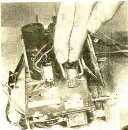
Other parts, such as capacitors and resistors, may be roughly checked with an ohmmeter by disconnecting one terminal. Try a few new components to learn about what to expect of good equipment so that you can recognize a faulty component when it turns up in your portable. —30—
