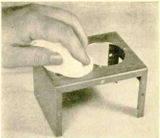
**2** Using a soft cloth dampened with clean water, wash the front panel thoroughly. Be sure you remove all grease, finger marks, and dirt before applying decals.
