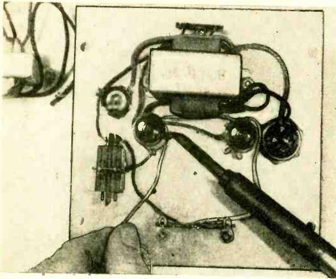
Do as much wiring as possible before installing the output transformer, T2. When looking down on the tube socket, the numbering is counterclockwise.
