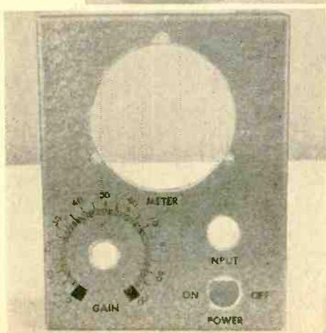
**8** A completed front panel. After the plastic covering thoroughly hardens, mount controls and other parts. Compare with Fig. 1.
