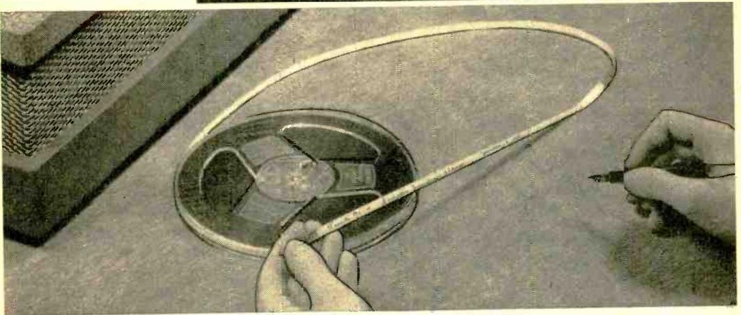
The smooth writing surface of No. 43 tape accommodates pen or pencil marking. Using it for labeling programs recorded on tape helps identify their contents. It also facilitates locating individual selections when several are recorded on one reel.
