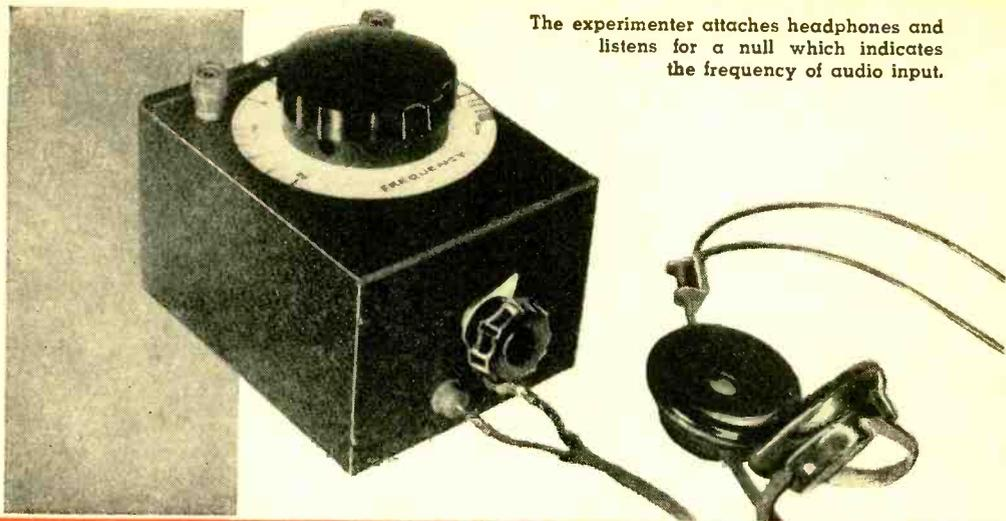
The experimenter attaches headphones and listens for a null which indicates the frequency of audio input.
