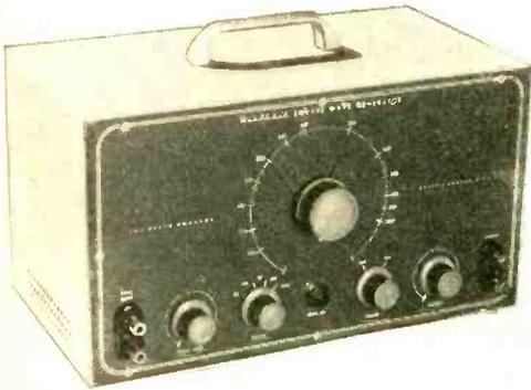
These two instruments are readily available kits for the experimenter and technician. Above is the HEATHKIT square wave generator Model SQ-1. At right is the EICO generator for both square and sine waves, Model 377. Both are reasonably priced and may be assembled in a few evenings of soldering and wiring.
