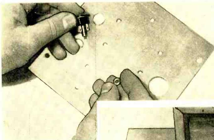
Tube sockets are flush-mounted on metal spacers which may be purchased from a local jobber or cut from copper tubing.
