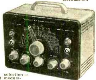
Output selection — internal modulation, pure r.f., or audio output.
