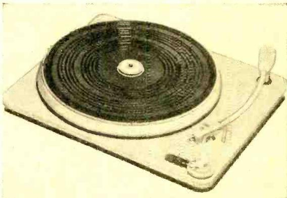
Components Corporation Model PBT gets maximum flywheel effect from 25-lb. cast-iron turntable. Nylon sleeve bearing, in which it rotates, reduces metal-to-metal contact. Motor is double-shock-mounted at maximum distance from turntable to reduce magnetic hum pickup. Reported performance data: 0.25% speed accuracy; 0.05% wow and flutter; -70 db rumble. Special spindle centers record on turntable and prevents slipping. Net, \$99.50. Components Corp., Denville, N. J.
