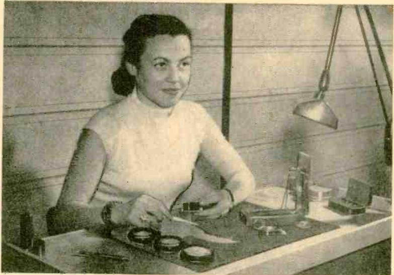
Inspection of the raw unfinished diamonds and sorting according to size.
