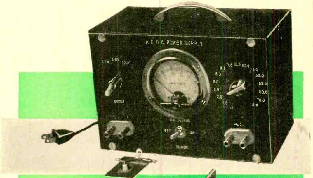
Front view (top) of the complete unit showing the engraving used on author's model. A G-E germanium power rectifier appears in the foreground. Rear view (right) with unit removed from cabinet shows location of major components and indicates how wiring may be cabled.
