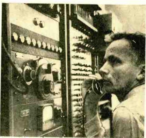
that determined which of ten numbers from 1 through 0 had been spoken into an ordinary telephone. It responded by flashing an appropriate light, as can be seen in the photo. At the time that the development of this device was announced, the Bell Labs people hoped to use it in conjunction with their telephone dialing operations.
