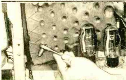
**Easy ratchet movement**—plus the offset angle of this tool—is a big help when you have to turn a screw or nut in a half-hidden corner. The rubber pad in background is used to protect TV tube from accidental slips.
