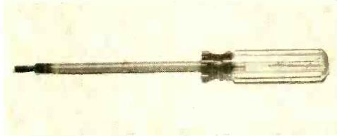
driver (15 cents). The screwdriver shown, as it came from the store, had a 4"-long shaft heavily covered with a break-resistant plastic tube of high dielectric strength. The outside diameter of the insulated shaft was  $\frac{3}{16}$ " (see top photo).
