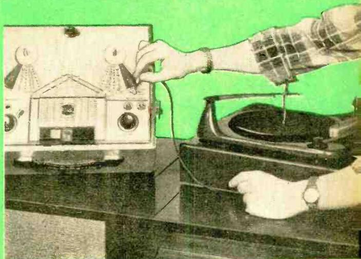
receive a signal that is strong enough to modulate the tape fully, so that even the lowest passages will be comfortably above the noise level. On the other hand, the signal must not be so high that it overloads either the circuits in the recorder or the tape itself. Either kind of overload means distortion.
