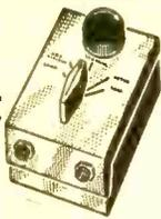
Yes, it's true! Order one at only 79¢ and get another for only 1¢. This handy Jack and Control Box is a genuine Signal Corps No. 1C-1366. A rare bargain for experimenters. A two piece cast aluminum box 3 1/4 x 4 1/2 x 2 1/2". Contains 2 phone jacks, a 5 position rotary switch with one spring return position, an eleven contact male and female contact board with silver plated terminals and 2 knobs. Shpg. wt. 2-2 lbs.
