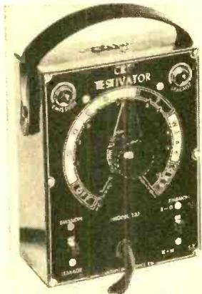
The "Testivator" checks cathode emission, indicates shorts and leakage between elements, tests for open elements, and estimates the probable useful life of the tube. It activates the CRT cathode by removing surface contamination, restores emission, and clears inter-element shorts and leakage. Price is given as \$14.95. (Century Electronics Co., 111 Roosevelt Ave., Mineola, N. Y.)
