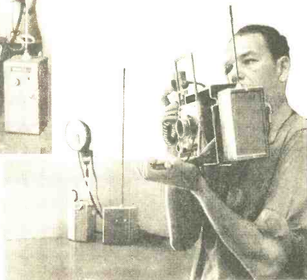
Complete outfit includes receiver, camera and transmitter. Lyle Byland, who developed units, looks at flash in top photo.
