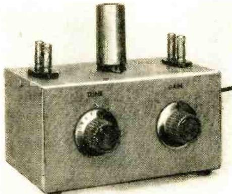
Placing the preselector stage in the receiver is usually an impossible task, but it can be conveniently made up on a small box and mounted atop the receiver. In this case, it is constructed on a 3" x 4" x 6" aluminum box, as shown above.
