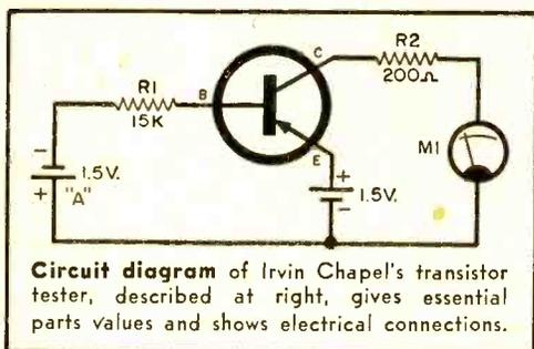
**Circuit diagram** of Irvin Chapel's transistor tester, described at right, gives essential parts values and shows electrical connections.
