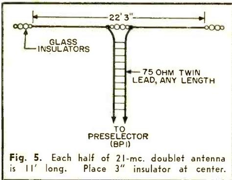
**Fig. 5.** Each half of 21-mc. doublet antenna is 11' long. Place 3" insulator at center.
