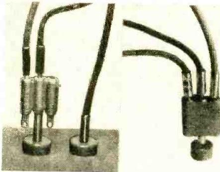
by-side. Then solder the lugs on the center jack into the sleeve of a phone-tip. Note how you can plug in one or two wire leads without interfering with the earphone connections. To dress up the adapter, clip off the lugs on the two outside jacks and wrap some wide Mystik tape around them.
