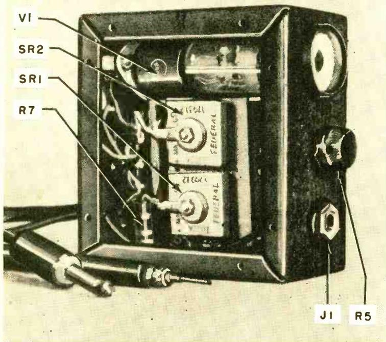
With the "magic-eye" tester, you can probe any point in a radio, television set or other electronic device from less than 0.5 to 500 volts. The "magic-eye" indicates whether voltage is positive or negative d.c. or a.c. and differentiates between low and high d.c. voltages. At left, the unit is shown with power supply installed and major components identified. Capacitors are mounted on the other side of the Micarta insulating board.
