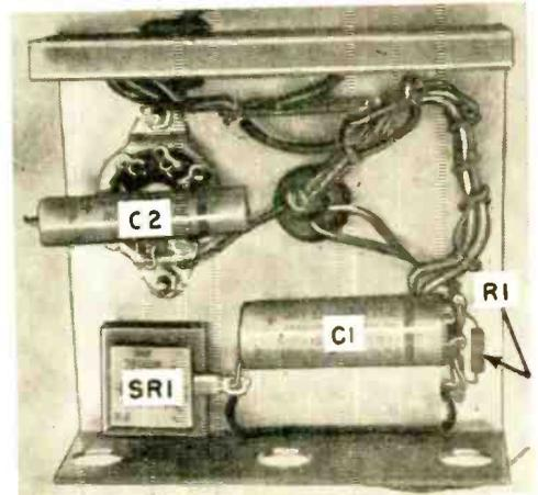
Two views of open-end chassis. Top view identifies enclosed-type relay RL1, isolation transformer T1, meter M1, and potentiometers R2 and R3. Underchassis view shows placement of selenium rectifier SRI, resistor R1, and capacitors C1 and C2.
