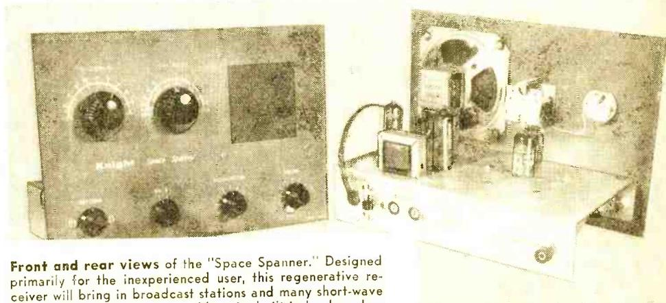
Front and rear views of the "Space Spanner." Designed primarily for the inexperienced user, this regenerative receiver will bring in broadcast stations and many short-wave stations from all over the world on its built-in loudspeaker.
