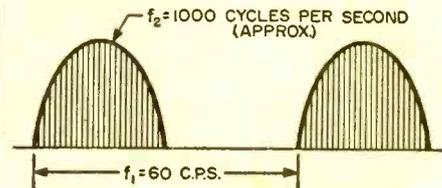
cycle fundamental results in a signal every 60 cycles from 60 cycles to over 10 megacycles.
