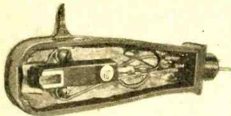
inated by lining the interior surface of the pickup end of the tone arm with heavy household aluminum foil, and then grounding the foil and the metal case or mounting of the cartridge to the braided shield of the pickup lead. —F.H.T.
