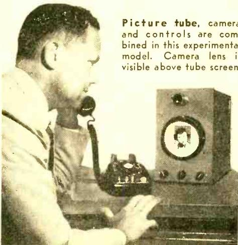
**Picture tube, camera and controls** are combined in this experimental model. Camera lens is visible above tube screen.
