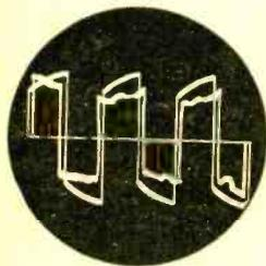
Two traces occurring one after the other are presented simultaneously for comparison on Memotron.
