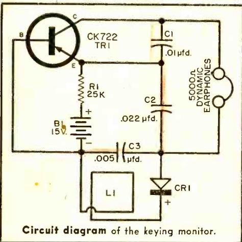
phone should be used . . . crystal earphones will *not* work in this circuit.
