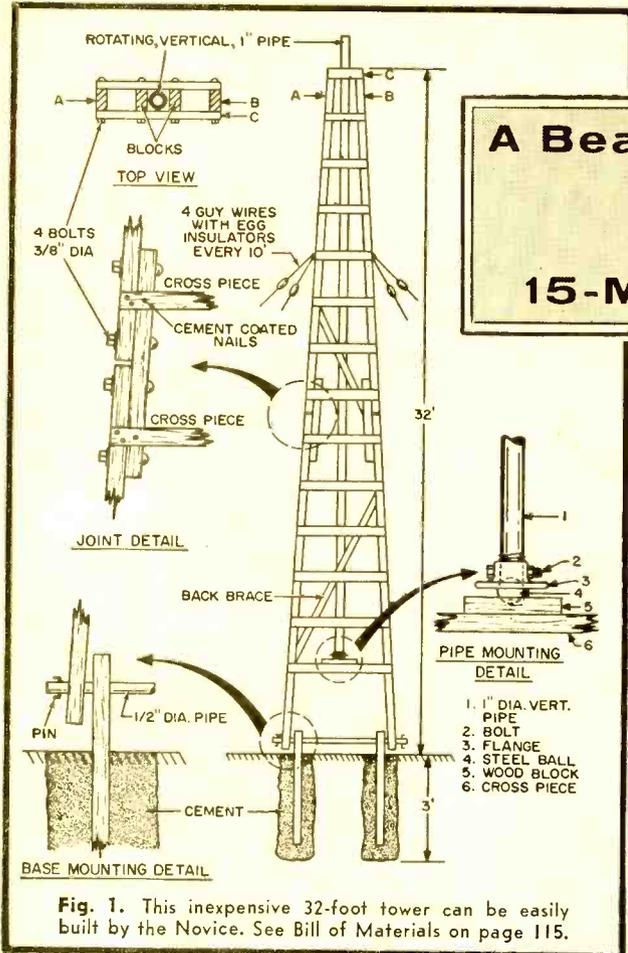
**Fig. 1.** This inexpensive 32-foot tower can be easily built by the Novice. See Bill of Materials on page 115.
