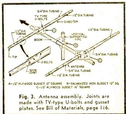
Fig. 3. Antenna assembly. Joints are made with TV-type U-bolts and gusset plates. See Bill of Materials, page 116.
