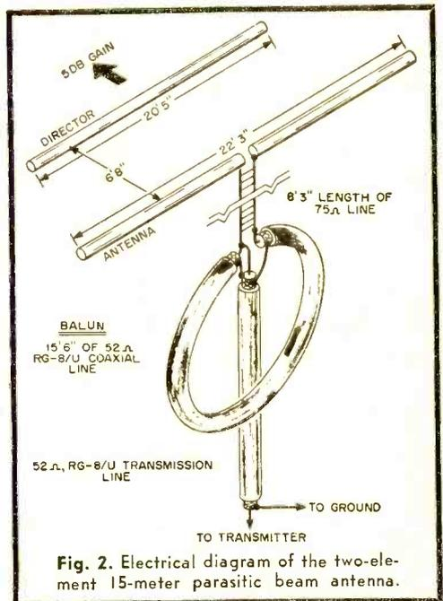
Fig. 2. Electrical diagram of the two-element 15-meter parasitic beam antenna.
