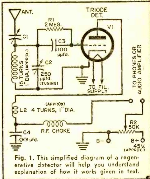
Fig. 1. This simplified diagram of a regenerative detector will help you understand explanation of how it works given in text.
