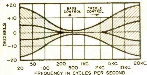
Ranges of control available with the circuits shown in (C) and (D) on page 55 are shown respectively in the two graphs above. Shaded areas indicate total range. Any combination of values between outer lines is possible. Note that the bottom graph shows that the point in the frequency spectrum, where tonal boost or cut begins, can be varied as well as the actual amount of boost or cut. For this reason, the circuit—the Baxandall system—is generally rated as best for hi-fi.
