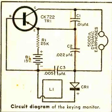
Circuit diagram of the keying monitor.
