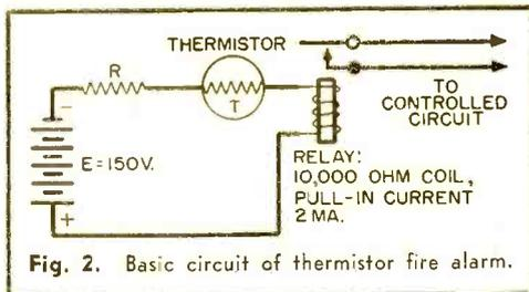
Fig. 2. Basic circuit of thermistor fire alarm.
