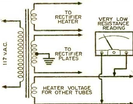
to the 117-volt winding. The small number of turns of heavy wire account for the very low resistance—which is often less than 1 ohm. —E.F.C.
