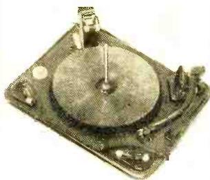
**Record changer**, Model RC-88, is improved version of Garrard RC-80. Unit plays at three speeds automatically or manually, as desired. Motor is 4-pole, shaded induction type. Weighted turntable, 1" high, turns on ball bearings, and is covered with rubber mat. Wow and rumble are said to be negligible. Tone arm, made of aluminum, uses plug-in shell which accepts most pickups. Stylus pressure and pickup height adjustments are provided. Unit is supplied with two spindles; mounting base is extra.
