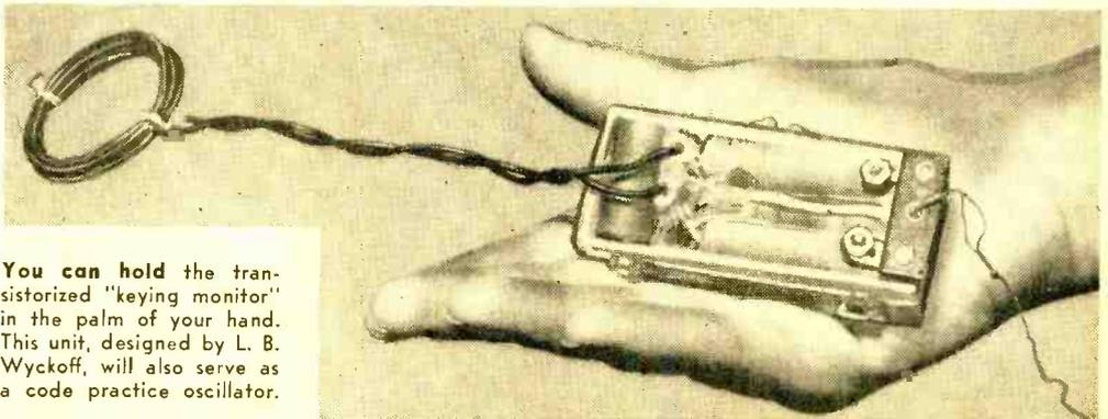
You can hold the transistorized "keying monitor" in the palm of your hand. This unit, designed by L. B. Wyckoff, will also serve as a code practice oscillator.
