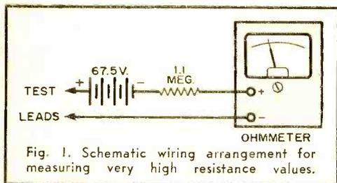
ternal hookup is awkward and inconvenient. The obvious need for a compact and convenient ohmmeter multiplier can be met with miniature transistor batteries. Such a probe can be made completely self-contained and as convenient to use as the conventional test lead.
