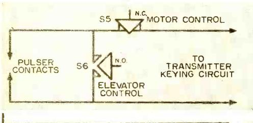
**Fig. 1.** Control switch hookup for proportional pulser. S5 and S6 (shown on top of unit at right, which was built by the author) are normally closed for motor control and normally open for elevator control.
