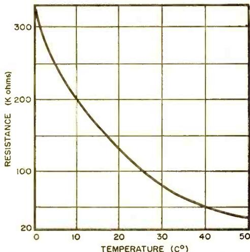
Fig. 3. Resistance-temperature curve for a 51R2.
