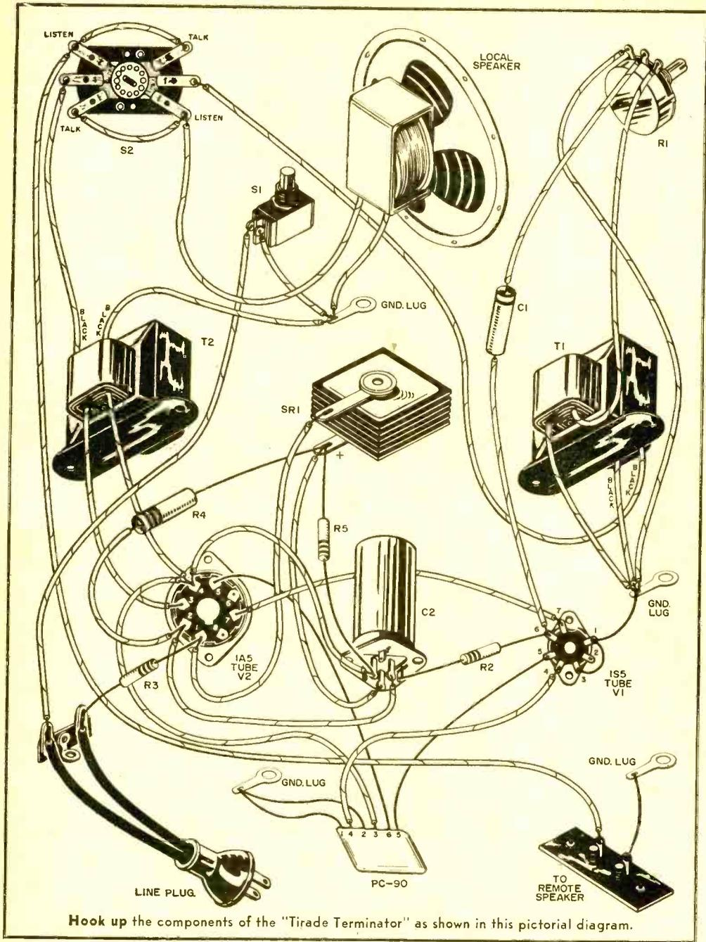
Hook up the components of the "Tirade Terminator" as shown in this pictorial diagram.
