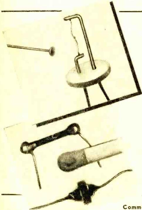
**Common shapes** in which thermistors are made. The head of a pin (top) is gigantic compared to tiny bead thermistor (A33 VECO) in center of fine wire. In the bottom square, a 51R2 VECO rod thermistor and a small disc thermistor are contrasted with ordinary paper match-head.
