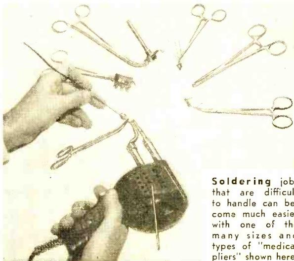
**Soldering jobs** that are difficult to handle can become much easier with one of the many sizes and types of "medical pliers" shown here.
