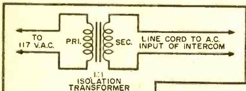
To eliminate any chance of shock, an isolating transformer having a 1:1 turns ratio could be connected as shown between the line and the a.c. input to the intercom—making precautions in text unnecessary.
