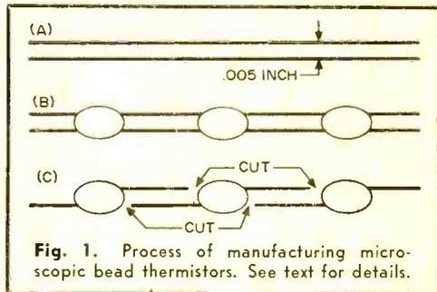
Fig. 1. Process of manufacturing microscopic bead thermistors. See text for details.
