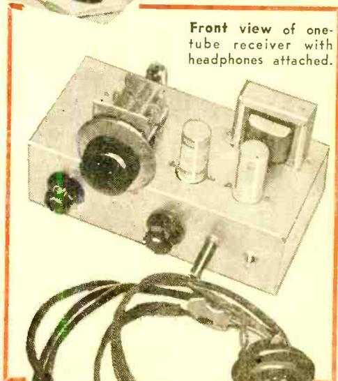
tered in the tickler when the latter is swung down over the tuning coil. You don't have to be especially precise about the coupling between the two coils.
