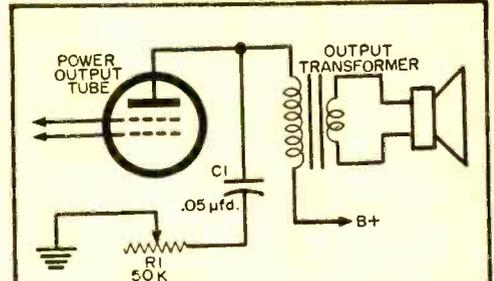
(A) Simple treble attenuation circuit.
