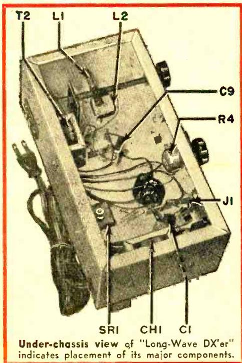
Under-chassis view of "Long-Wave DX'er" indicates placement of its major components.
