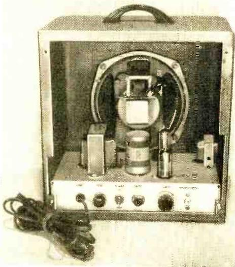
**Rear view** of amplifier case shows placement of the speaker and amplifier chassis. The gain control and jack for harmonica pickup are on the panel.
