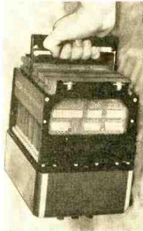
complete control unit. Cards are fitted into their holder in building block fashion. Known as "Transac," the device can add two numbers in 1.5 microseconds; it multiplies in 15 microseconds. This unit contains nearly 1000 tiny transistors, 300 resistors, and 12 capacitors permanently dip-soldered. It was developed by the Philco Corp., Philadelphia, Pa.
