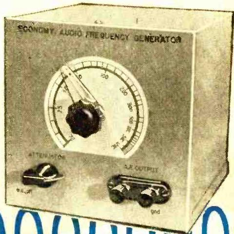
**It's inexpensive, uses only one tube, and will cover range from 22 to 12,000 cycles**
