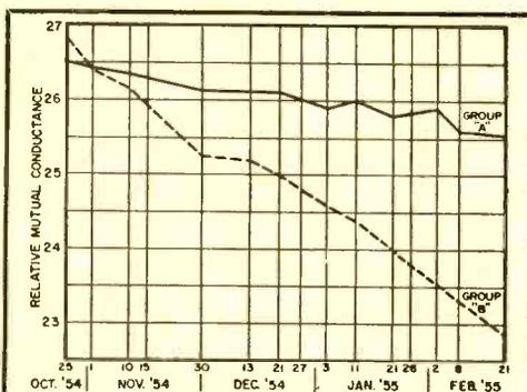
**Decay of tube efficiency** measured in terms of mutual conductance of two groups of tubes. Group A was used with Tube-Saver, Group B without. Group B deteriorated three times faster. Measurements were made by U.S. Testing Co.
