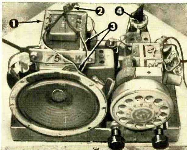
**Changes** which will improve sound in small, 5-tube a.m. receiver; ① new output transformer; ② leads connecting to external loudspeaker; ③ negative feedback connections; ④ added filter capacitor with unused terminals taped. Latter is clamped to i.f. can.
