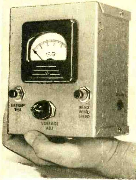
Front view of anemometer control box with meter which may either be calibrated directly to read wind velocity or may be used with a graph.
