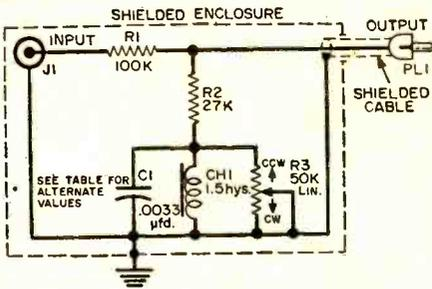
Schematic diagram and parts list are shown directly at left. Table below lists different "presence" frequencies that may be emphasized with different C1 values. Bottom diagram shows how to connect "outboard" presence control into circuit of complete amplifier.
