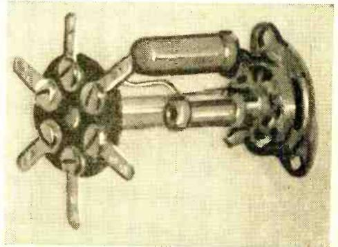
the connecting pillars. The method of attaching the pillar to the 9-pin socket is male to female, while for the 7-pin type it is female to male. Acrylic cement is useful in gluing these parts. Solder lugs are held to the turret with machine screws in tapped holes.
