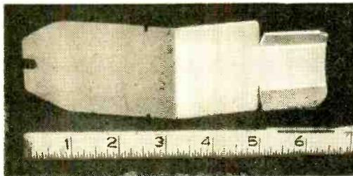
**2** Rocker arm (above) is fashioned from aluminum. Notches must fit snugly into narrower part of rocker cutout in aluminum mounting frame. The leaf spring is stainless steel strap and the switch bracket is aluminum. All dimensions are given in table on following page.
