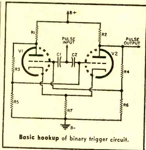
across  $R1$  again increases, making the plate of  $V1$  even more negative-going. Clearly, the effect is cumulative, with the grid of  $V2$  finally going negative enough to cut off the plate current. All this takes a tiny fraction of a second. At the time when  $V2$  is cut off, the grid of  $V1$  reaches approximately zero voltage and the system becomes stable, the plate current of  $V1$  being just about as large as it can become.
