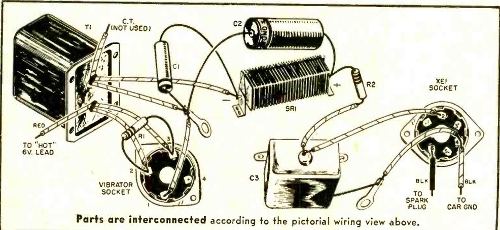
Parts are interconnected according to the pictorial wiring view above.
