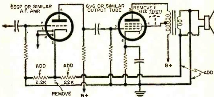
Simply reverse connections to secondary of output transformer to correct this situation. Some sets will operate best with a lower value resistor than 2200 ohms. Use lowest one that gives good results.
