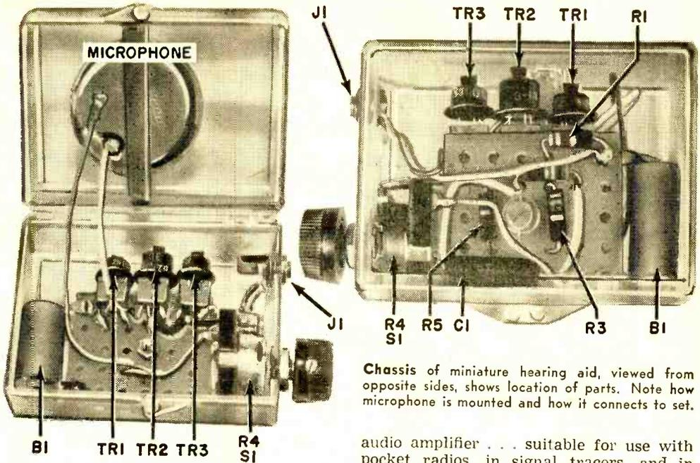
Chassis of miniature hearing aid, viewed from opposite sides, shows location of parts. Note how microphone is mounted and how it connects to set.
