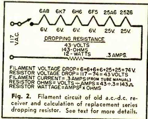
Fig. 2. Filament circuit of old a.c.-d.c. receiver and calculation of replacement series dropping resistor. See text for more details.
