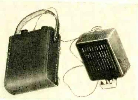
**The Lafayette KT-96 kit** (above, right) was designed to be used with Lafayette Radio's transistor superhet kit called the KT-94 (above, left).
