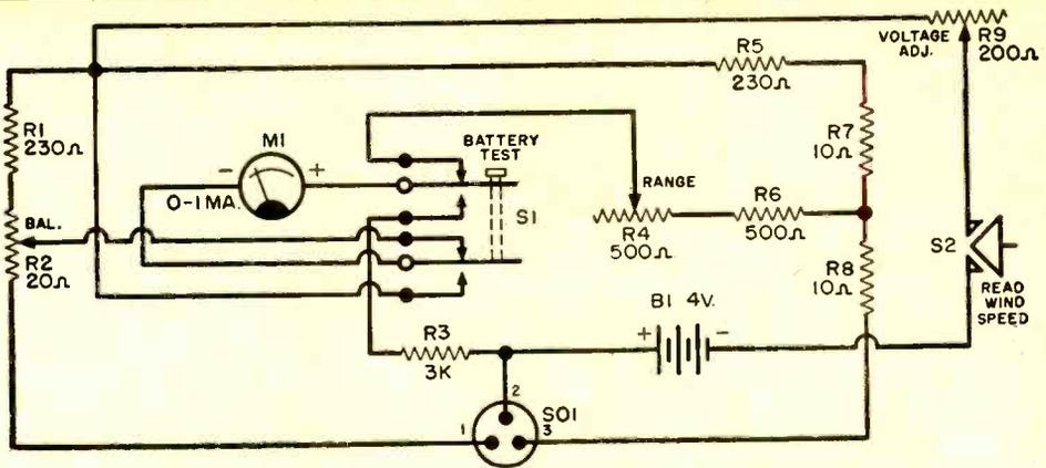
Diagrams and parts list for the electronic anemometer. The circuit above is contained in the control box; the thermistors diagrammed on the right are placed on a separate base and located out in the open. A three-wire cable connects the thermistor assembly to the control box containing the meter. Pictorial diagram showing method of connecting parts is at the left.
