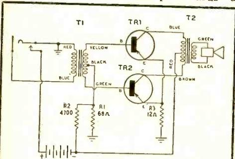
**Schematic diagram** of the KT-96 push-pull audio output speaker kit. Note in this wiring arrangement that the sleeve of the phone plug must be the signal lead and that the tip is the ground connection. The positions are reversed to permit the battery to be saved when the unit is not in operation. Simply plugging in the phone jack turns on the amplifier.
