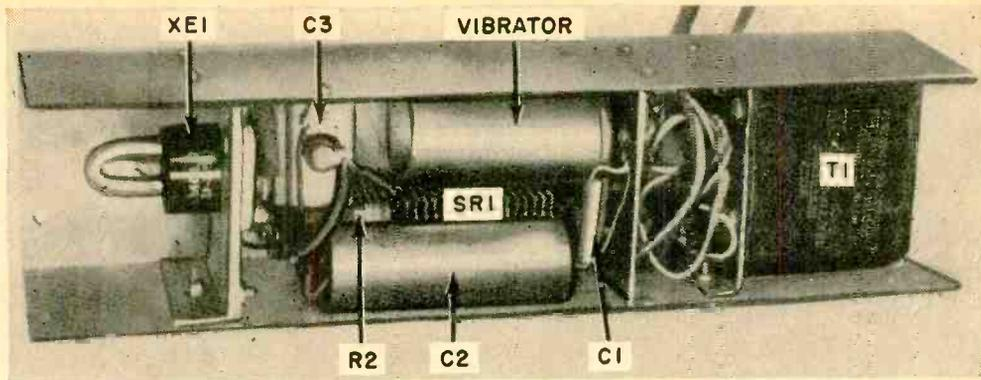
**Aluminum case** for the electronic timing strobe can be purchased at most radio parts jobbers. The transformer used by the author was one he obtained at a second-hand store. Note placement of major parts inside the case (above). The lens, which can be taken from a broken flashlight, is held in place by a simple bracket (below, left). All three leads enter the case through grommets (below, right); the heavy lead is the cable connection to the spark plug.
