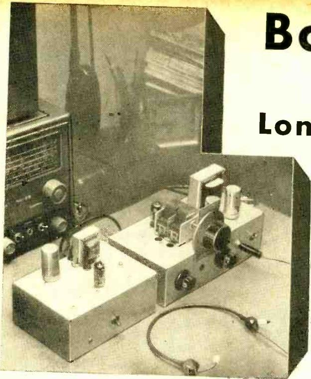
**I**F YOU ARE TUNING the long-wave band (100-500 kc.) and would like to fish for DX, or if you have been troubled by interference from broadcast stations leaking through your receiving setup, then this booster is for you. It requires no manual tuning. You merely connect it between your antenna and your receiver or converter, make one simple adjustment, and then tune your setup.
