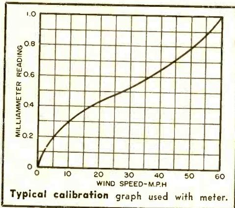
a full-scale reading on the meter. At this point, a reading of 1.0 ma. is equivalent to a wind speed of 60 m.p.h.\*
