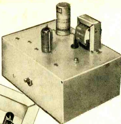
**Location** of parts is shown in these two photos. Above, top-chassis view shows (left to right) 6BA6 tube, the dual electrolytic capacitor, and the miniature power transformer. At left is under-chassis view. Parts designated by call-out numbers are detailed in parts list on page 87. Location and mounting of the three r.f. chokes is critical. See text for detailed explanation.
