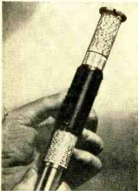
achieves graduations equal to those of a 66" slide rule. It is claimed to be more accurate than any slide rule currently on the market. The plastic-covered scales are fully resistant to wear and moisture, and since all parts
