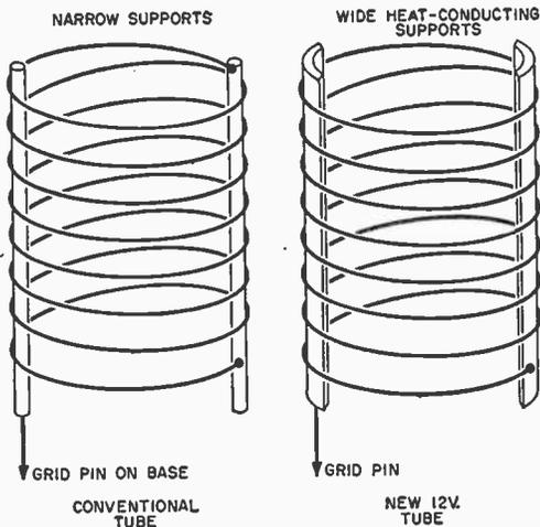
**Fig. 3.** Wide grid supports act as heat sinks for the 12-volt tubes—help cool the grids by conducting heat away quickly, minimizing grid emission. This is not as great a problem with the older tubes.
