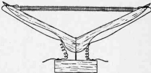
hanger and bring the ends through holes drilled in the hanger arms. The metal hook section can be straightened and cut off short to provide a rotary base. —L. T.
