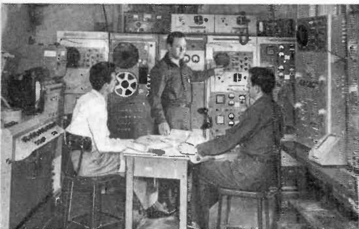
**Measuring** telemetered data from rockets in flight at an installation in Manitoba, Canada. At the far left is a telemetry recorder which takes data from airborne rockets; in the center is the main recorder which puts data on tape; the ballistic camera master control is at the right.
