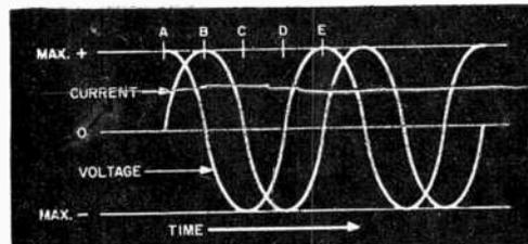
through the inductor in that direction. But, as soon as the current tries to reverse direction, the magnetic field generated by the current flowing in the original direction starts to collapse, and its energy is converted back into an electromotive force that tends to keep the current flowing in the original direction.
