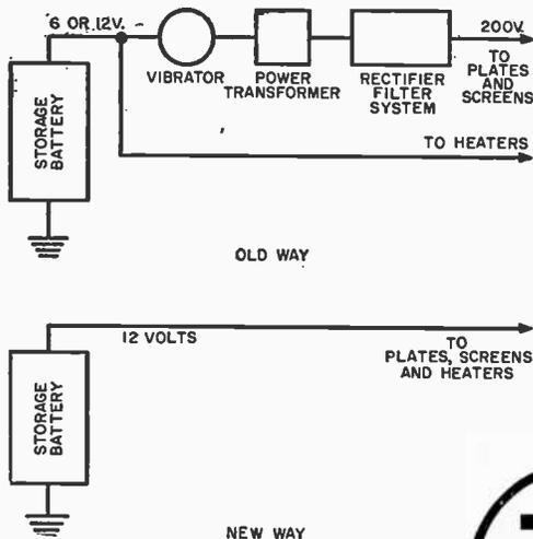
Fig. 1. The new low-voltage tubes make vibrator power packs virtually obsolete.
