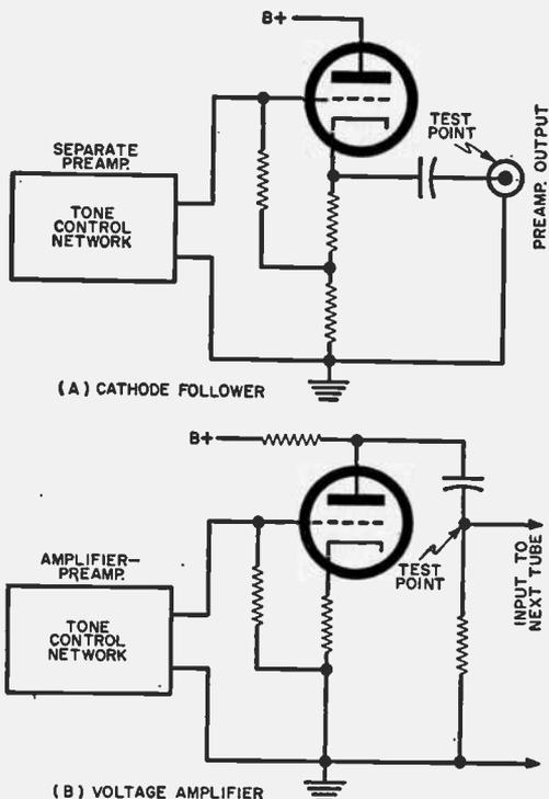
**Fig. 3.** The points indicated in (A) and (B) will provide the most reliable take-off points for your oscilloscope.
