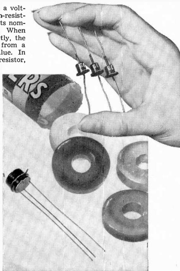
**Semiconductor devices** currently being produced by General Electric Co. include low-current silicon rectifiers (above, right), and a silicon double-based diode (right, compared in size with Life Savers). The tab protruding from the cap of the diode serves as a ground for shielding purposes.
