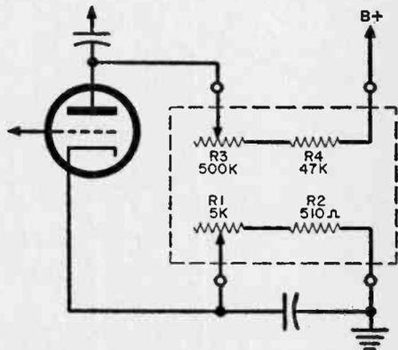
Fig. 2. How to determine plate load and cathode resistors needed in a particular amplifier stage.
