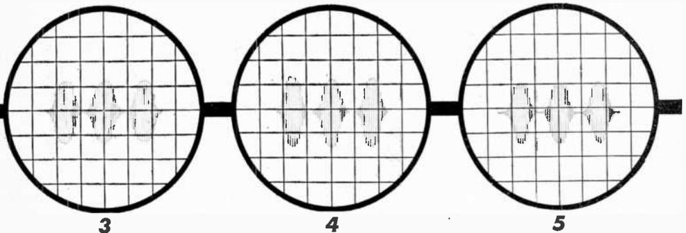
and adjust the sweep to give a good trace of the audio signal. The gain should be increased to the point where distortion begins to show on the signal.
