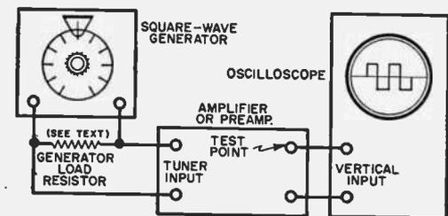
**Fig. 2.** Test setup used when running square waves through the amplifier.
