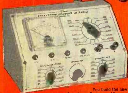
You build the new Sprayberry Tester... 18-range Volt-Ohm-Milliammeter readings.
