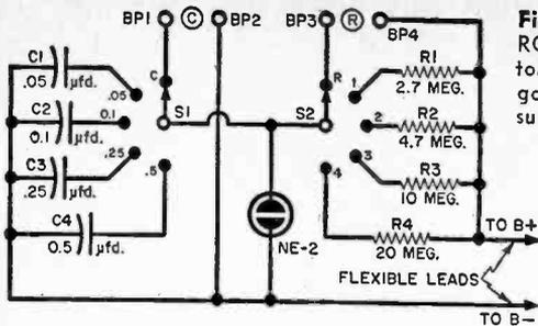
**Fig. 1.** Schematic diagram of the simple RC tester. Resistors should be of 5% tolerance and the capacitors should be in good-quality, low-leakage types to insure proper functioning of the instrument.
