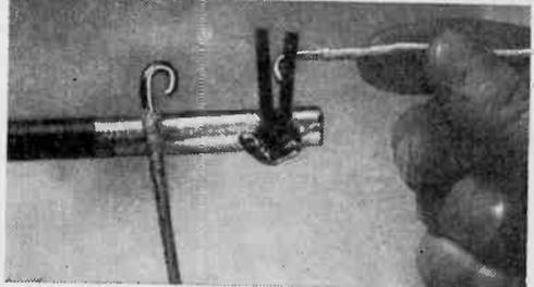
wire for making connections. Two 1½" headless bolts are welded at one end to a piece of bar or scrap iron which serves as a handle. Separate the free ends of the bolts to make a narrow "V." The stripped end of the wire to be looped is introduced from the rear and merely given a pull towards the front, forming a perfect loop. Spacing of the bolts allows the tool to handle wire
