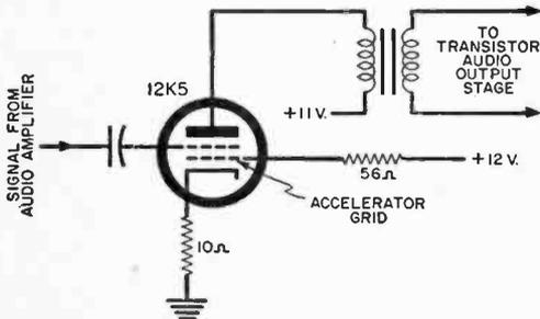
**Fig. 4.** Typical circuit using the 12K5 driver tube. An accelerator grid carrying a positive charge is located between the cathode and control grid.
