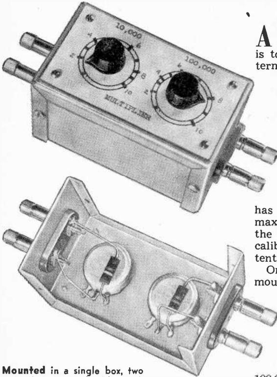
Mounted in a single box, two potentiometers should each have linear taper to insure uncrowded calibration scales. Dials can be calibrated by measuring the potentiometer resistance at various settings.
