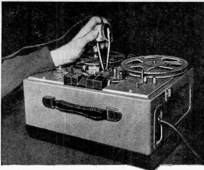
When you use a demagnetizer, withdraw it very slowly from head. Typical operation of Audio Devices Co. unit is shown above.
