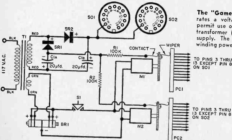
The "Gamester" circuit incorporates a voltage doubler circuit to permit use of an inexpensive power transformer (T1) as a high voltage supply. The transformer's filament winding powers the miniature motors.
