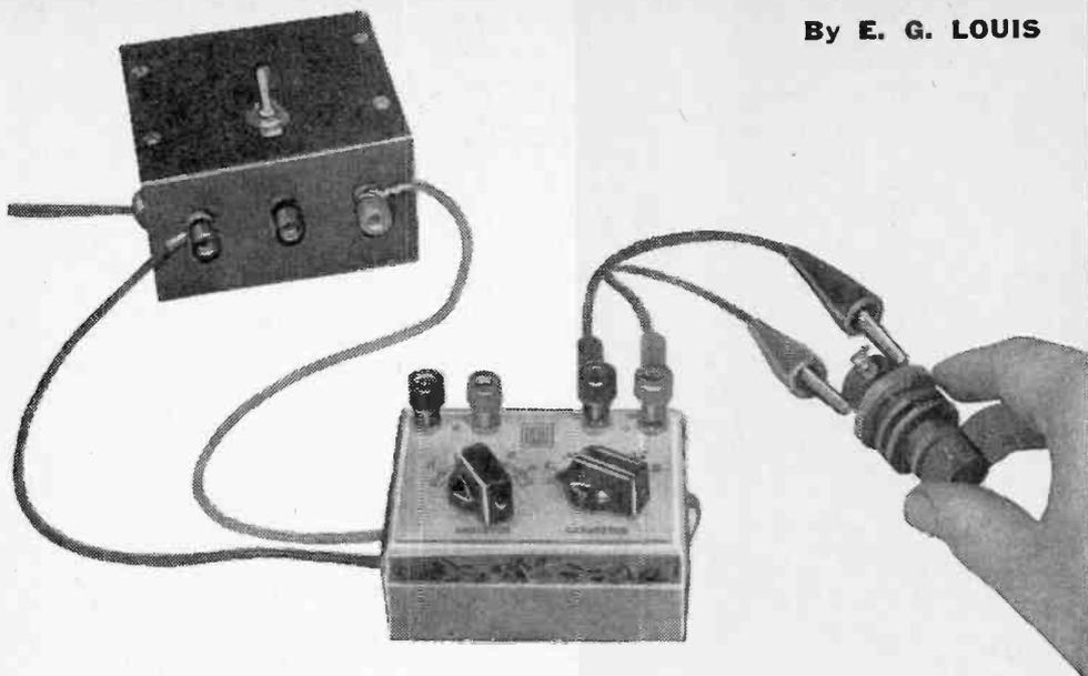
**A**S RESISTORS and capacitors make up the majority of electrical parts used in electronic equipment, it is important that both the home experimenter and service technician have adequate means for checking them. Resistors are usually checked with a standard ohmmeter which has a limited range, and few low-cost ohmmeters will give a usable reading at values above 500,000 ohms or 1 megohm. Yet 2 to 20 megohm resistors are encountered frequently in receivers and amplifiers.
