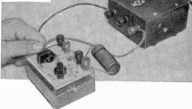
A capacitor is shown being tested in the photo below.
