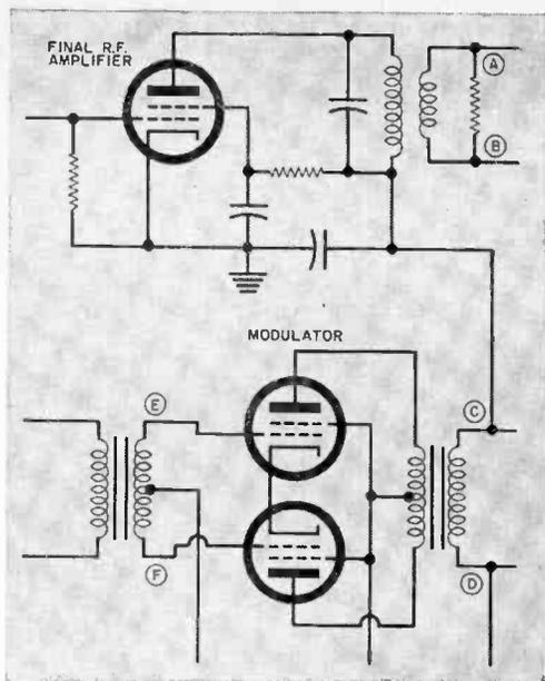
The circuit of a typical r.f. amplifier with push-pull modulator. Lettered test points indicate where the oscilloscope probe connection is made for each test trace. See text for complete details of modulation monitoring procedure.
