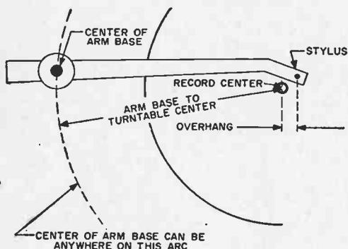
**Fig. 2.** These are the dimensions you must measure to find the right place for mounting your tone arm.
