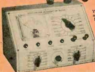
You build the new Sprayberry tester—a complete 18-range Vol.-Ohm-Milli-ammeter test meter.
