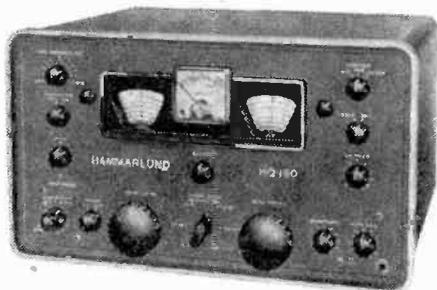
cuits in the i.f. to provide extremely clean side skirts. The second i.f. frequency is crystal controlled for optimum stability. A Q-multiplier is built into the unit.
