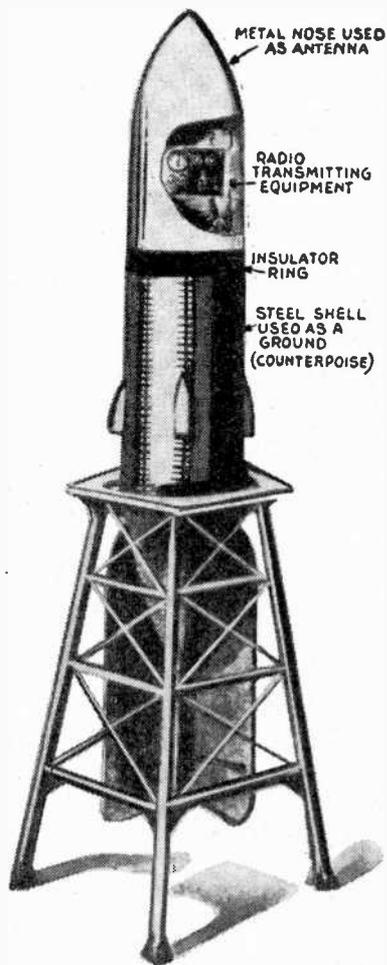
Proposed design of the Moon Rocket. A radio transmitter, in the nose, will send out waves continually on its course.
