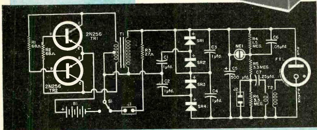
leaves only the four silicon rectifiers and the four capacitors (*C1*, *C2*, *C3* and *C4*) of the voltage quadrupler. They also are pre-wired, using a physical layout which corresponds with the placement shown in the schematic. Considerable space is saved by using pigtailed on the rectifiers instead of mountings clips.
