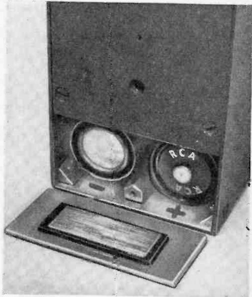
Battery installation; note the polarity markings and insulated contact plate.
