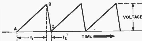
Fig. 5. Sawtooth waveform output of the generator which utilizes self-induction for voltage boost.
