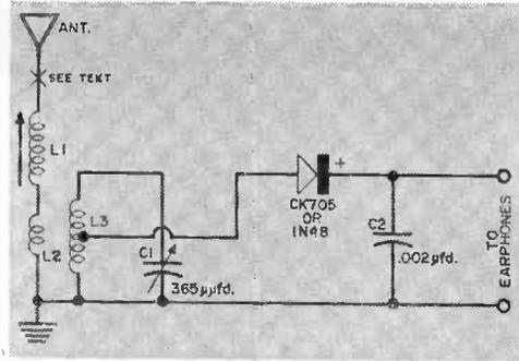
at 30 turns. Leave a ⅜" space between coils. If you use an antenna that is over 75' long, insert a 3-30 μfd. trimmer at point "X."
