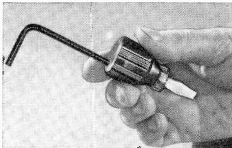
the outside and the center of the handle so that the wrench will be well separated from the embedded screwdriver shank. —K. M.
