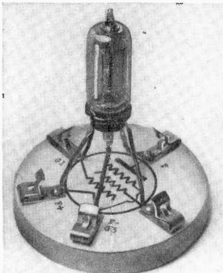
where the connections go. Radio students and experimenters can make up a number of these graphic tube mounts, one for each of the most commonly used tubes, and save much time and trouble when trying various hookups. —A. T.
