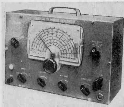
marker generator and vertical-horizontal bar generator. It has a frequency range of 3.5 mc. to 250 mc. in six bands with 1% accuracy. Calibration is checked by means of a 4.5-mc. crystal, accurate to 0.002%, mounted on the front panel.
