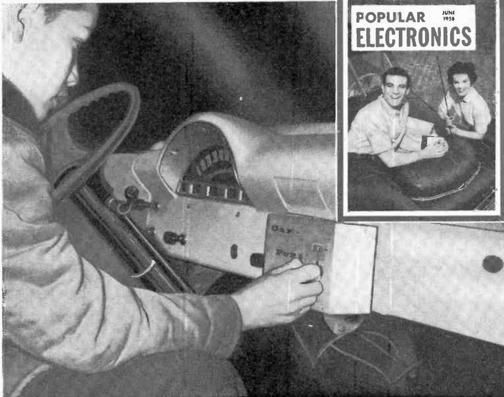
**M**ANY PEOPLE want to know if it is possible to purchase a portable radio and operate it in an automobile as well as take it on a picnic. It is possible. But the portable would have to be built in a metal case to shield it from the ignition system. And inasmuch as the metal car top and body would prevent the radio waves from reaching the built-in antenna of the set, an outside antenna must be installed.
