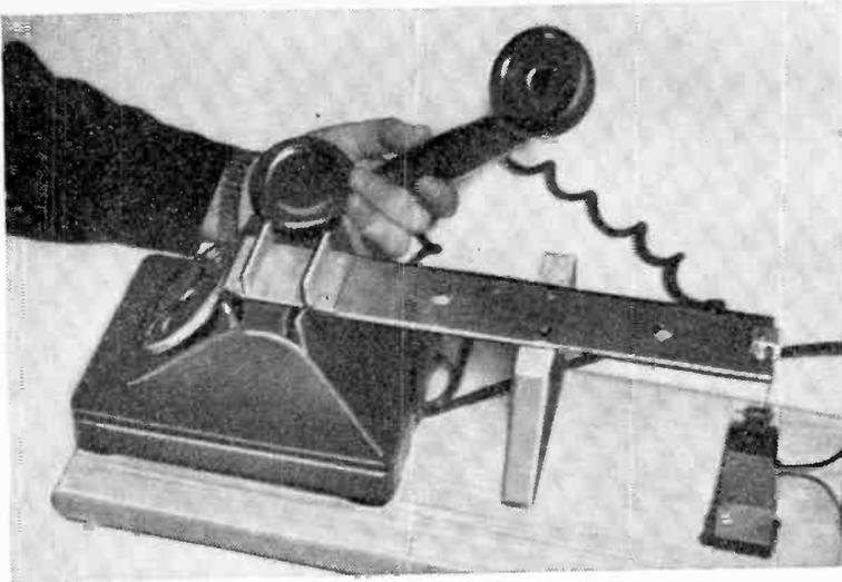
**Handset lifter** mechanism in place. Voice pickup coil is beneath the base, bell pickup is on the far side.
