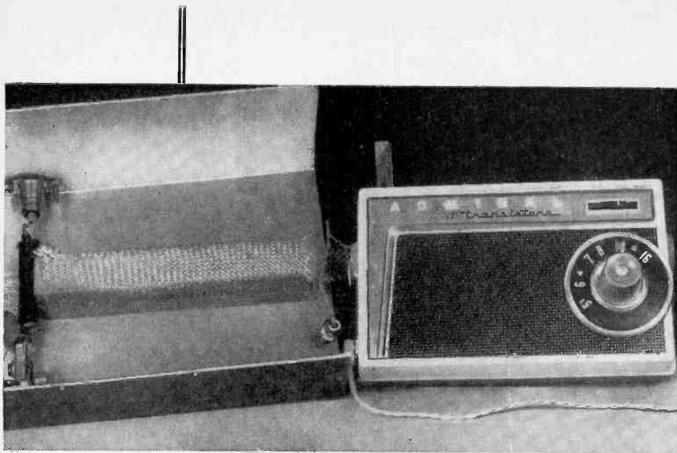
**Padded wooden blocks** can be used to hold receiver securely inside metal box. On some cars, there might be enough space behind the dashboard for mounting both the set and the speaker.
