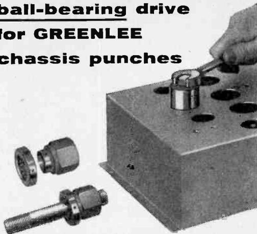
New GREENLEE Ball-Bearing Drive Nuts and Drive Screws reduce friction and make it easier than ever to cut smooth, accurate holes with GREENLEE No. 730 round Radio Chassis Punches. The new faster drives are available for all round-type GREENLEE Punches sizes 11/16" through 2-25/32". Operate with ordinary wrench for quick socket openings etc. in metal, bakelite, or hard rubber.
