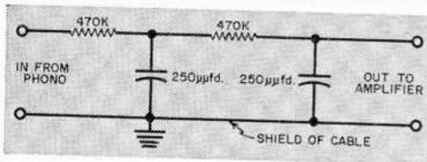
**The circuit** (at left) consists of a tandem, low-pass RC network.
