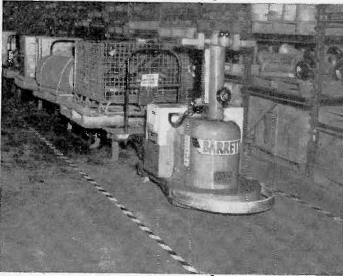
You don't need an engineer on this tractor-train, because the system at Esso's Baton Rouge refinery is electronically controlled. The train, which pulls five trailers at  $2\frac{1}{4}$  miles an hour, follows the electromagnetic field of a wire laid in the floor.
