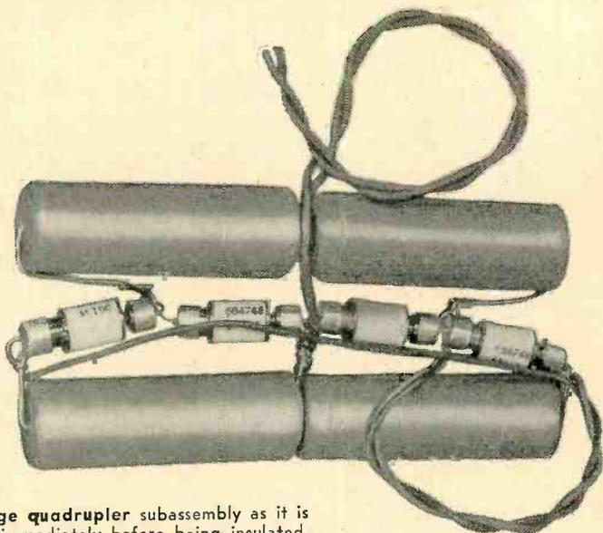
**Voltage quadrupler** subassembly as it is wired immediately before being insulated.
