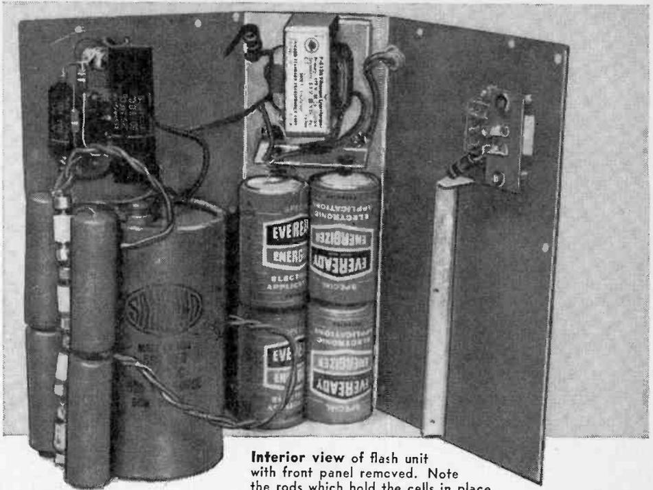
Interior view of flash unit with front panel removed. Note the rods which hold the cells in place.
