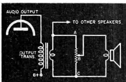
Fig. 1. Pot used as a speaker volume control (not recommended).
