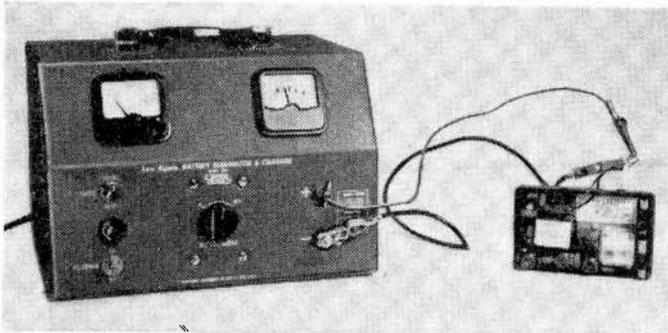
The 1060 is ideal for powering a transistor radio, as shown at left.
