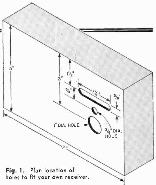
**Fig. 1.** Plan location of holes to fit your own receiver.
