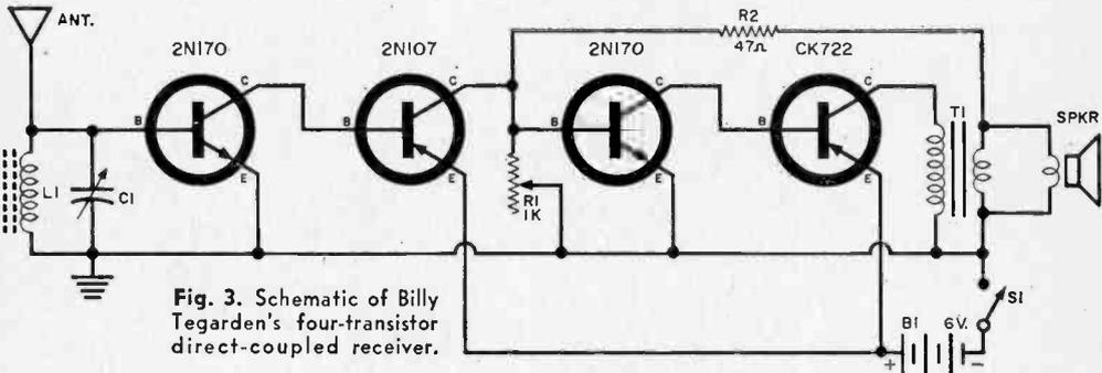
Fig. 3. Schematic of Billy Tegarden's four-transistor direct-coupled receiver.
