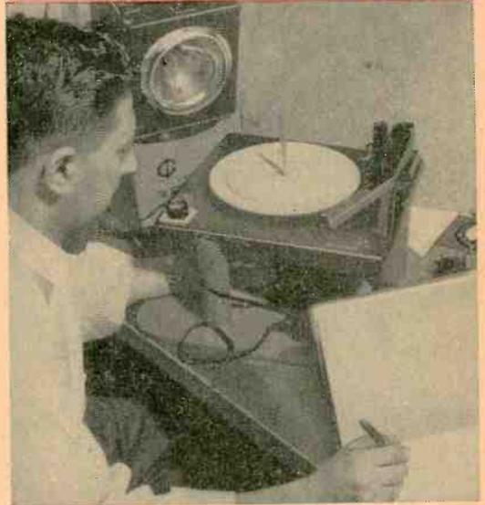
Development lab prepares stripped-down model for resonance and vibration tests. Pickup arm output is fed to vertical deflection plates of oscilloscope. Audio oscillator output fed to horizontal plates simultaneously will produce Lissajous pattern to determine frequency of any resonances. Later a vibration analyzer will be used to detect gross resonance. Results of such experimental work are compiled for future developmental use by the firm.
