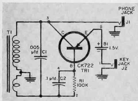
which it can be helpful. With the inexpensive transistors now available, it is easy to build a battery-operated oscillator tiny enough to fit in your pocket and have a battery life of a year or more.
