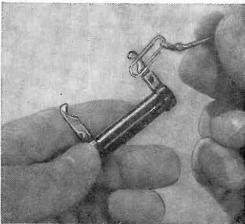
ample. One of these clips will connect the ends of several wires together instantly and is easily attached to the posts of resistors, capacitors, etc. A tug on a wire serves to disconnect it, so no time is wasted.—K.M.
