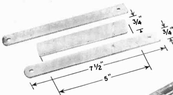
**Dimensions** for the parts of the handle are given at left. Battery mounting clamp is made of a length of angle iron as shown below.
