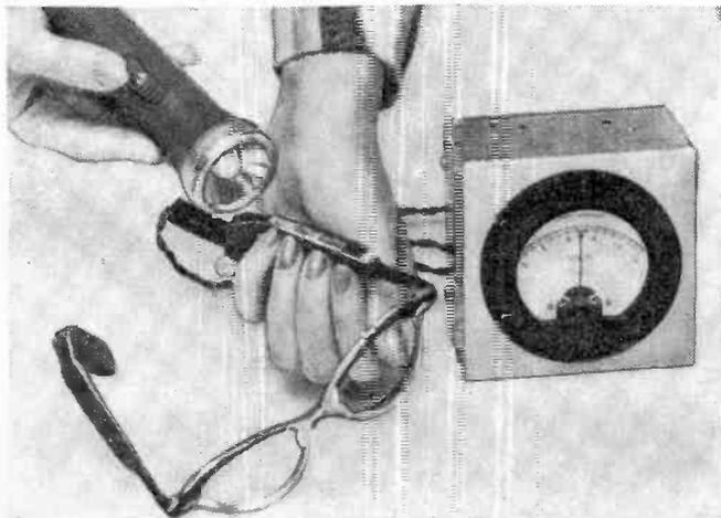
Hearing aids take on a new dimension with the debut of the new Zenith Solaris unit, which employs silicon solar cells (same type as used in the Vanguard satellite) to power its amplifier. The cells are so efficient that they can even use the weak light of a flashlight to register a voltage. Overcast sunlight will run the device properly. In darkness, it automatically switches to batteries. It uses four transistors.
