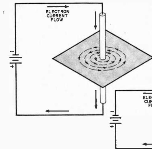
Fig. 1. The magnetic effect of a current passing down through a vertical wire. Iron filings sprinkled on cardboard sheet trace out the magnetic forces.
