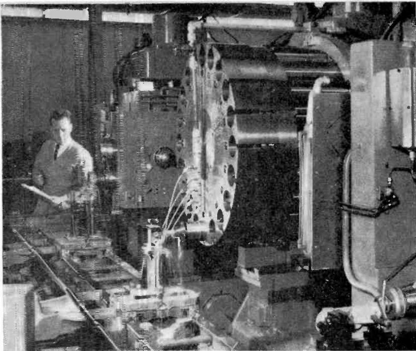
The nation's first all-electronically controlled line of machine tools is installed at Hughes Aircraft in Los Angeles. Working as a team, milling, drilling and boring machines pass parts along automatically after each machine operation. The line is operated by new Digitape electronic controls and was developed in cooperation with the Kearny & Trecker Corp., of Milwaukee.
