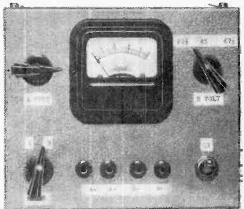
**Simple power supply replaces a wide variety of batteries in portable sets**
