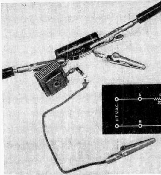
This simple circuit requires no chassis mounting. Lettered points in schematic of voltage source are explained in text.
