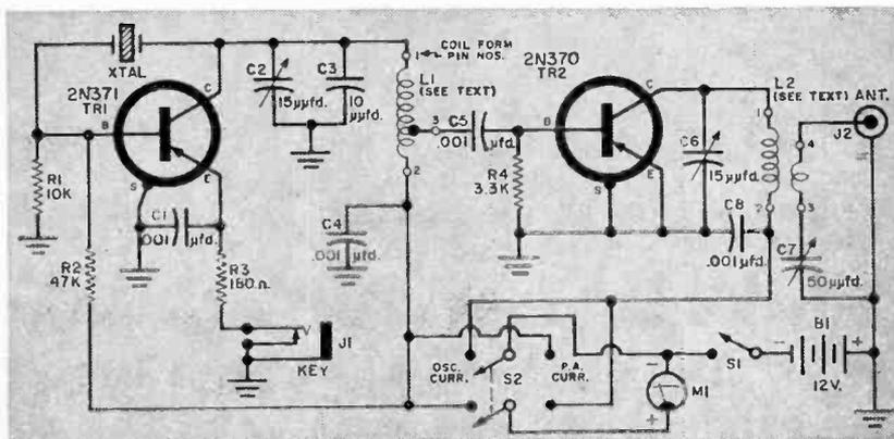
band and need only one set of coils. However, if you have General Class privileges, you can operate on either 10 or 15 meters. The coil data covers both bands.
