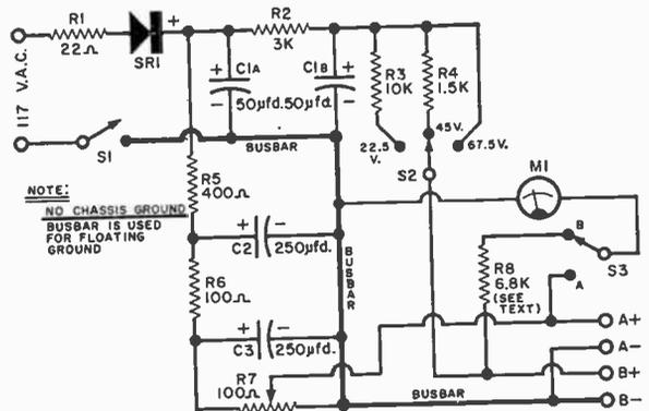
45, or 67½ volts for the "B" voltage. It has a built-in meter for reading either output *while in use*. A compact unit which can be built in a Bud Minibox cabinet, its total cost including the meter should be below \$15.00.
