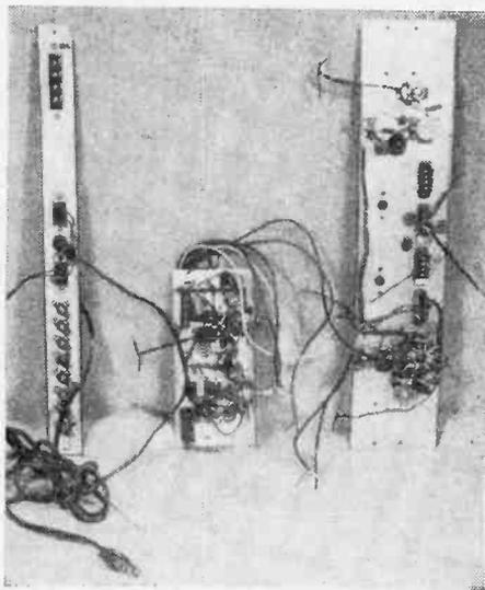
The four subassemblies of the SA-25 are shown above. Largest section, at top of page, includes the complete basic amplifier and power supply. The three smaller assemblies, directly above, are bolted onto the square end brackets and then interwired. Completed unit slides into the cabinet provided.
