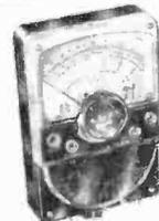
A terrific buy in a hand-held, compact, light, accurate, completely wired instrument. Has a 36  $\mu$ A movement, 1% precision resistors and simple selector switch with calibration markings protected against wear. Scales: Volts DC and AC; 0.5-25, 100, 500, 1000; Ohms: 0-6K-600K-6 Meg; DC Current: 0-50  $\mu$ A-5-50-500 MA; Decibels: -20 to +64 in 5 ranges. Size 4 3/8" x 2 7/8" x 1 1/4". Shpg. wt., 1 lb. Complete with batteries and test leads. Imported to save you money.
