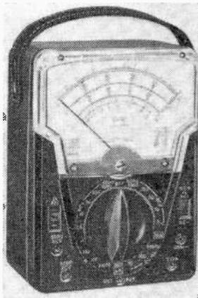
both circuit and range—minimizing wrong settings and burn-outs; and a.c. and d.c. voltage scales of 2.5, 10, 50, 250, 1000, 5000. (Triplet Electrical Instrument Co., Bluffton, Ohio.)
