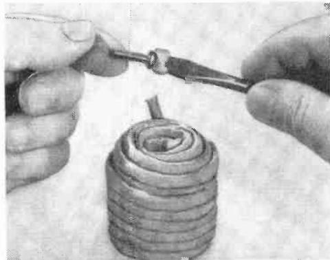
use the compound to hold a nut to the end of a screwdriver or even a piece of wood, such as a dowel, when the nut must be put into a location difficult to reach by hand. —K. M.
