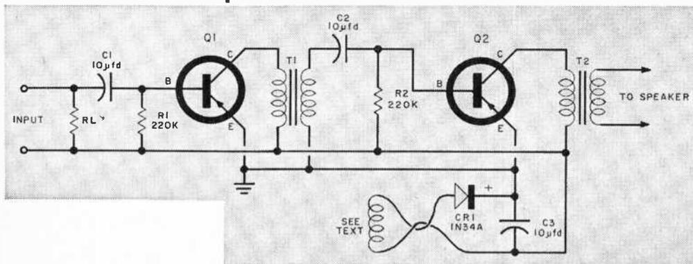
An extra winding (L1) added on a phono motor core will "steal" enough current to power a two-transistor amplifier. The same technique can be used with almost any small phono motor. The + lead of C2 should be shown connected to T1.
