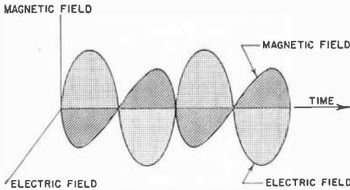
**Fig. 7.** An electromagnetic wave in space consists of two components lying in planes at right angles to each other.
