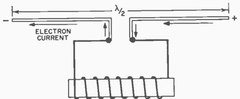
**Fig. 2.** A half-wave dipole energized by a transmitter tank coil. Each element of the dipole is a quarter-wave length, making a total length equal to a half-wave at  $\lambda/2$ . Arrows indicate direction of electron current at some arbitrarily chosen instant.
