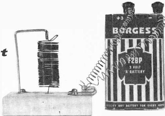
With a block of wood, about 10 feet of enameled wire, a small blob of mercury, and a three-volt dry cell, you
