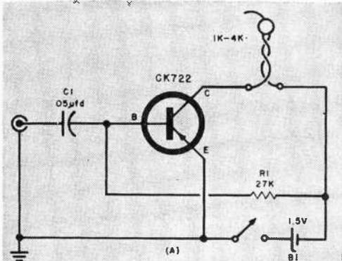
Fig. 1. Two useful transistorized audio amplifier circuits: Dave Harter's single-stage amplifier (A); and George Sollman's direct-coupled interphone amplifier (B).
