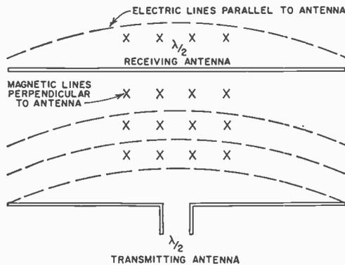
cal, the horizontal planes of the magnetic component can cut through the vertical receiving antenna *at right angles*. This condition, as we know from elementary magnetic induction principles, causes the maximum induced e.m.f.
