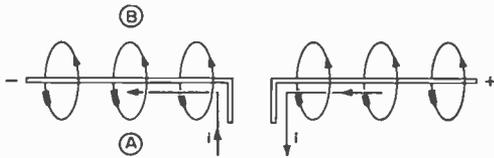
Fig. 3. Magnetic field surrounding the half-wave dipole takes the form of concentric circles lying in planes perpendicular to the conductor.
