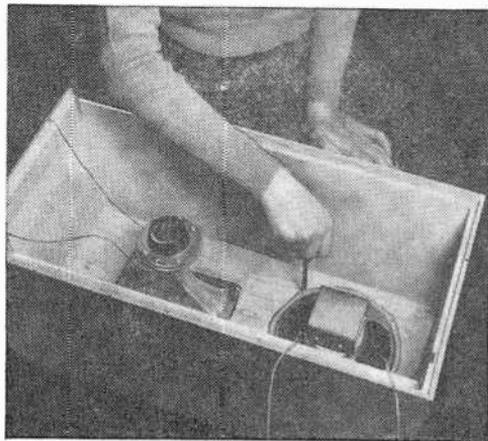
**Speaker installation** is quite simple. Tweeter is mounted on adapter and then is screwed down to the inside of the enclosure.
