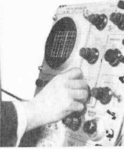
**Programing** a big computer is a tricky job, and it takes a specially trained technician to do it. While the Univac II is being warmed up, the electronic technician below is setting up "turn-on" instructions on the control panel.
