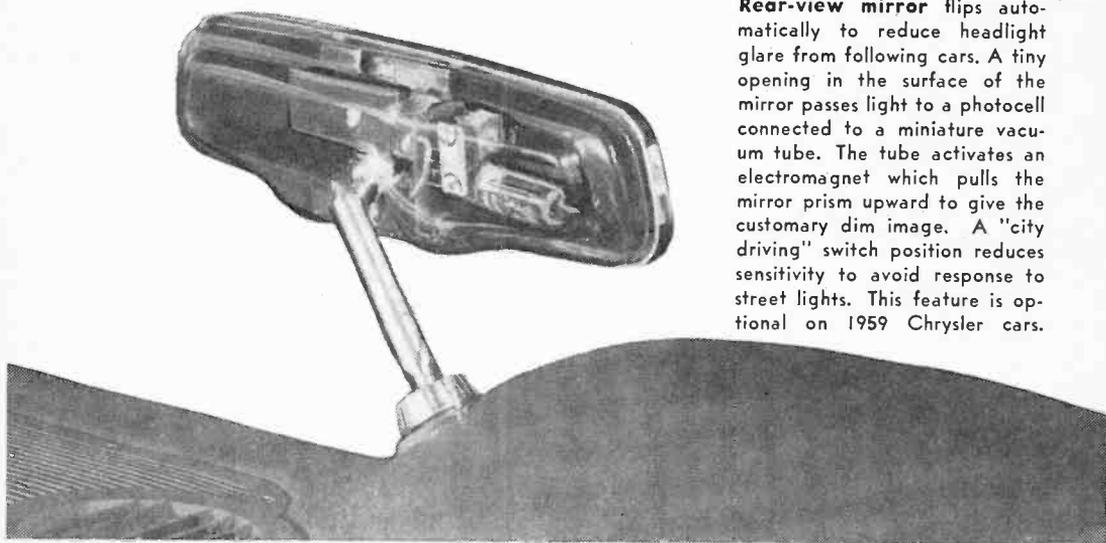
**Rear-view mirror** flips automatically to reduce headlight glare from following cars. A tiny opening in the surface of the mirror passes light to a photocell connected to a miniature vacuum tube. The tube activates an electromagnet which pulls the mirror prism upward to give the customary dim image. A "city driving" switch position reduces sensitivity to avoid response to street lights. This feature is optional on 1959 Chrysler cars.
