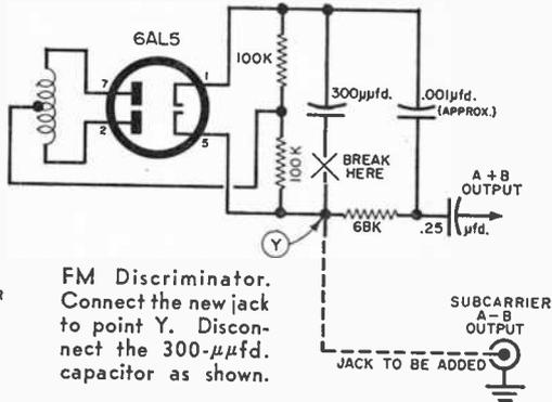
FM tuner circuit modifications which may be required for a multiplex output.
