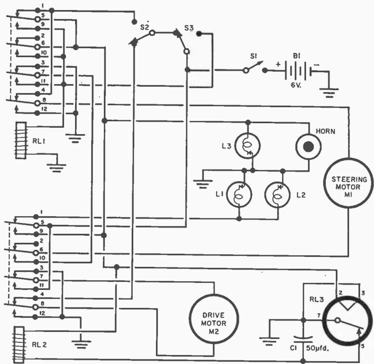
to contact 1 of  $RL2$ . The remaining lug of  $L3$  is connected to contact 9 of  $RL2$ .
