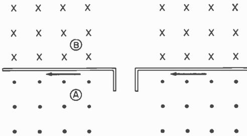
stands for the head of the emerging arrow and a cross for the tail feathers of a retreating arrow. This takes care of the instantaneous magnetic field due to the initial surge of electrons into the dipole (Fig. 4).
