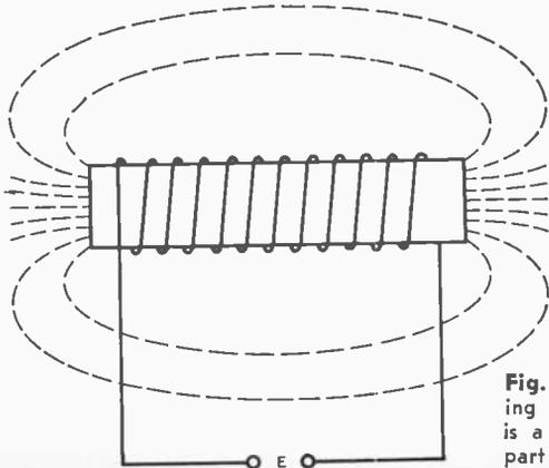
**Fig. 1.** The induction field surrounding a current-carrying coil. This is a short-range field which is not part of the electromagnetic wave.
