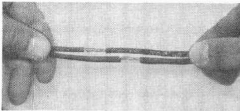
gether. This method staggers the connections, thus insulating them from one another. When soldered and taped, the joint is a slender, neat-appearing one. —P. B.
