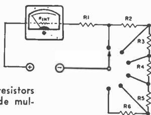
**Fig. 2.** Series resistors wired to provide multiple ranges.
