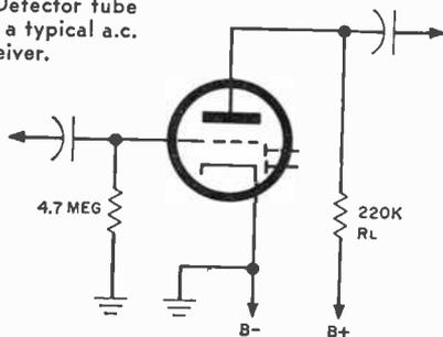
range and check the voltage on the tube's plate. What will the reading be? Oddly enough, the meter reading will depend on the sensitivity of the meter used. A 20,000-ohms/volt meter will read about 55 volts and a 1000-ohms/volt VOM will read about 42 volts. And if the 1000-ohms/volt VOM is switched to the 50-volt range, the reading will drop to about 17 volts.
