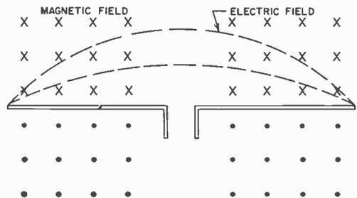
Fig. 6. Magnetic lines of force are always perpendicular to the accompanying electric lines of force.
