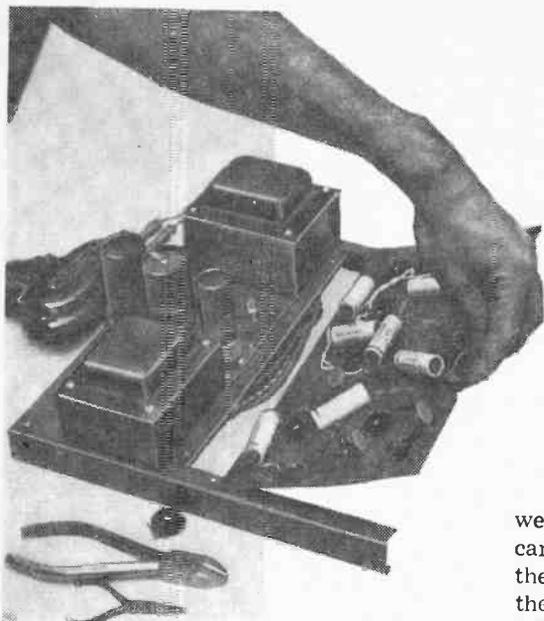
**Printed-circuit board** is wired as a unit and is installed on chassis when power supply has been completed.
