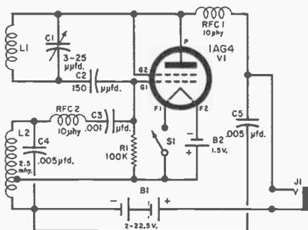
Antenna coil L1 is the only one requiring special winding. All others are commercially available. For longer battery life, a mercury cell can be used as B2 instead of standard penlight cell.
