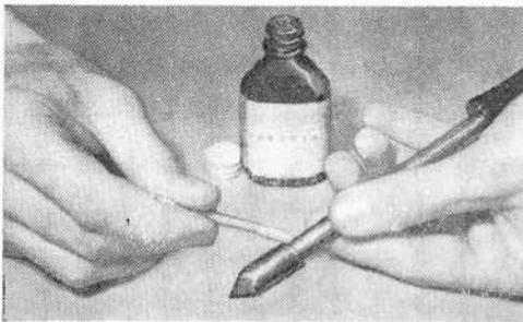
has, don't try to loosen it with pliers—you are liable to damage the tip. Instead, take a cotton swab or brush, dip it in ammonia, and apply it to the tip as shown. This will "unfreeze" the tip in a matter of minutes. —P. E. C.
