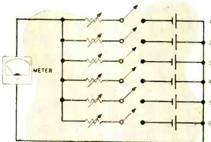
**3** Sam Addit made this simple computer to add any numbers from 1 to 6. The resistors were adjusted so that if battery #1 were switched in, the 0-15 voltmeter would read 1, switching in battery #2 would give a reading of 2, and so on. He figured that if a combination like 2 and 5 were used, the meter would read 7. What did it actually read?
