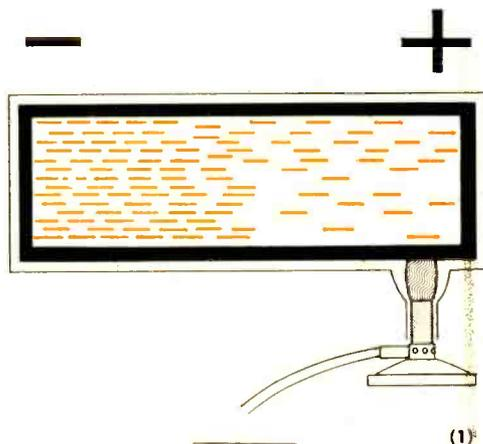
**Fig. 2.** Thermoelectric junction is between two materials which move electrons at different rates. When junction is heated and the circuit closed by a wire, current will flow.
