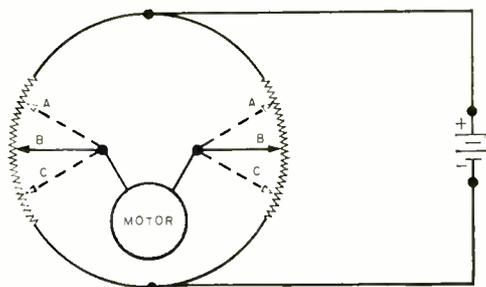
**Fig. 1.** Two potentiometers controlling a motor in this Wheatstone bridge circuit make for a continuous servo system. Whenever the two wiper arms are in different positions, the bridge is unbalanced and an error signal activates the motor.
