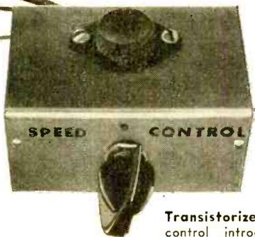
Transistorized speed control introduced as kit by Peck Products.
