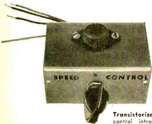
Transistorized speed control introduced as kit by Peck Products.
