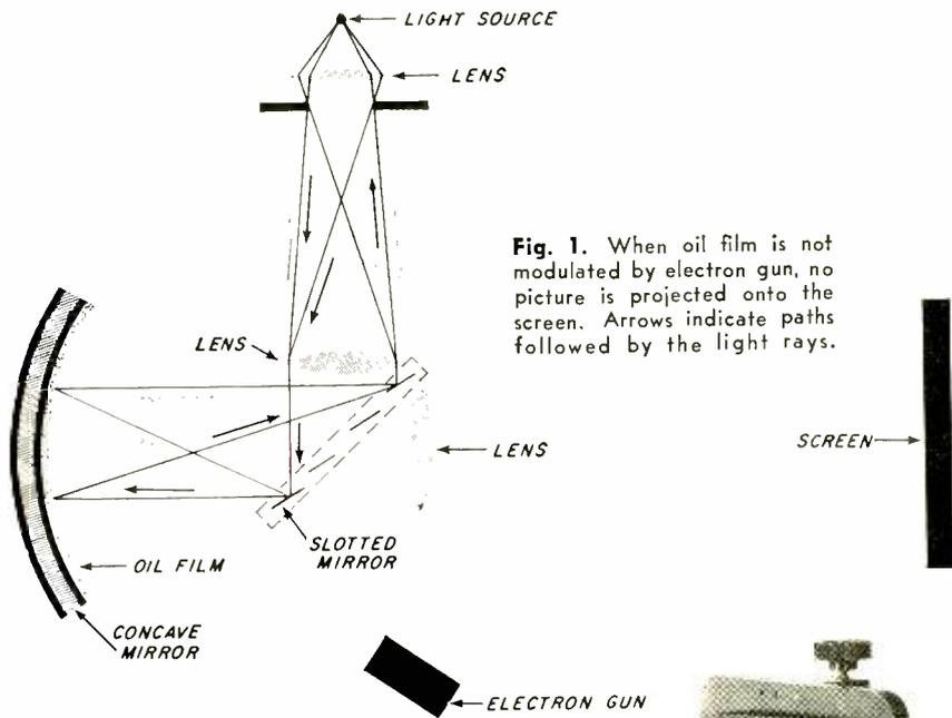
**Fig. 1.** When oil film is not modulated by electron gun, no picture is projected onto the screen. Arrows indicate paths followed by the light rays.
