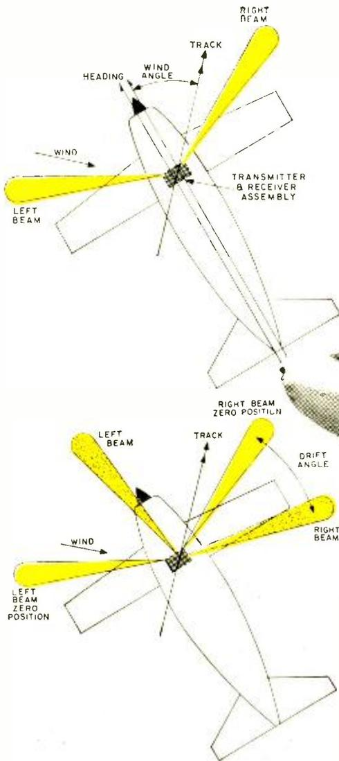
**DETERMINING DRIFT.** In zero position (diagram at left), twin radar beams straddle plane's nose, one aimed to the left and one to the right. When wind causes plane to move in direction different from heading (direction in which nose is pointed), Doppler frequency shift of right beam is greater than that of left beam and antenna swings until frequency shifts are equal again (diagram below, left).
