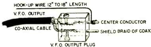
**To increase** the VFO output signal for frequency checking, add a 12" to 18" wire to the center conductor of the VFO output cable. The plug can be inserted into the crystal jack or the transmitter.
