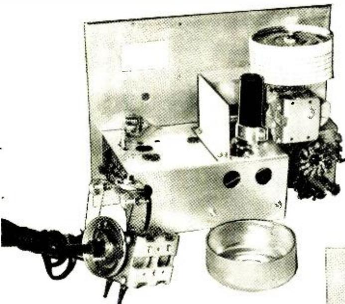
The r.f. assembly is shown mounted to the front panel, adjacent to the main chassis, in the above photo. The r.f. unit is at the right. The partially assembled a.f. tuning unit is in the left foreground, with the a.f. dial drum lying beside it.
