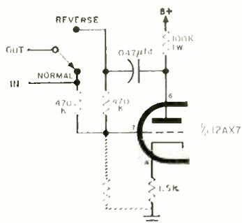
**Electronic phase reversal** can be accomplished by the circuit shown above. Switched output from grid and plate is  $180^\circ$  out of phase.
