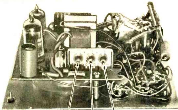
Completely wired unit is at left. Note the three internal adjustment potentiometers. Diagram below is from the construction sheet. Well planned illustrations reduce complex wiring to a simple task.
