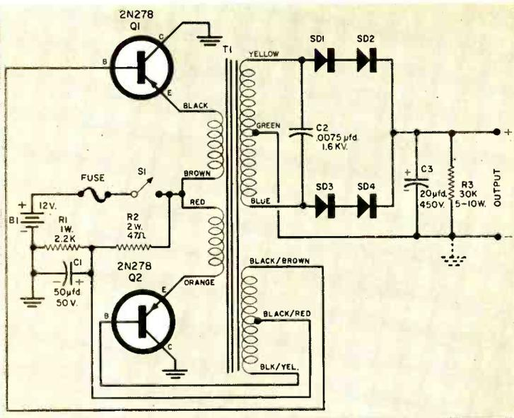
Fig. 2. Larry Edwins' transistorized B-voltage power supply for mobile transmitters, short-wave sets, p.a. systems, etc.
