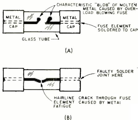
**Fig. 1.** Two types of fuse failure. The blown fuse (A) usually indicates excessive current drain due to momentary or permanent short circuit in the set. Fatigue failure of fuse (B) indicates only that a replacement is needed.
