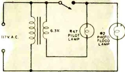
**1** Happy Snap, having only an s.p.s.t. switch, wanted to turn on a flood-light and a pilot light on the control board at the same time. Expecting no trouble, he wired his setup as shown. After double-checking his connections, he held his breath and inserted the wall plug. Things didn't quite work out. Do you have any idea why?
