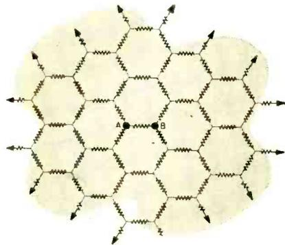
**4** Ned Work has a mesh of 1-ohm resistors connected as shown and extending across his living room floor. Some day he hopes to extend the mesh all the way to infinity—and maybe even beyond. Can you calculate what the resistance will be between points "A" and "B" when his "tangled web" is finished?
