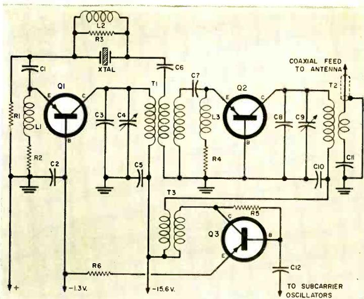
oscillator to the second stage.  $T1$ 's primary winding is tuned by  $C3$  and  $C4$ .  $C2$  and  $C5$  are bypass capacitors.
