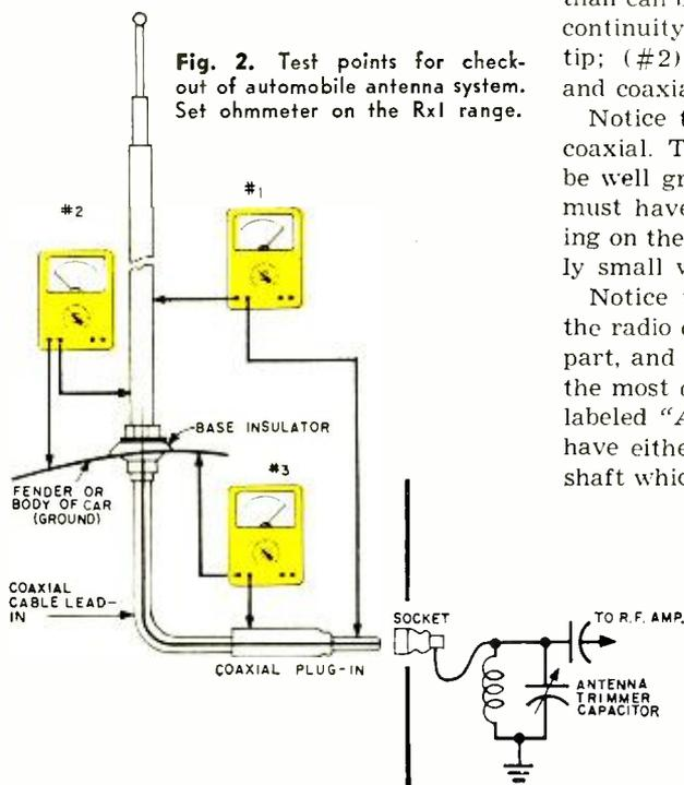
**Fig. 2.** Test points for check-out of automobile antenna system. Set ohmmeter on the Rx1 range.
