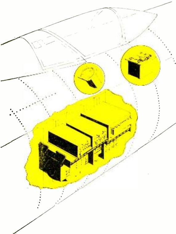
**SAMPLE LAYOUT.** Arrangement of assembly designed by Laboratory for Electronics, Inc., for use in a jet plane. Combined antenna-transceiver-computer package is mounted in plane's belly, while ground-speed and drift-angle indicator (circular dial) and control panel are in cockpit. Control panel indicates plane's exact longitude and latitude.
