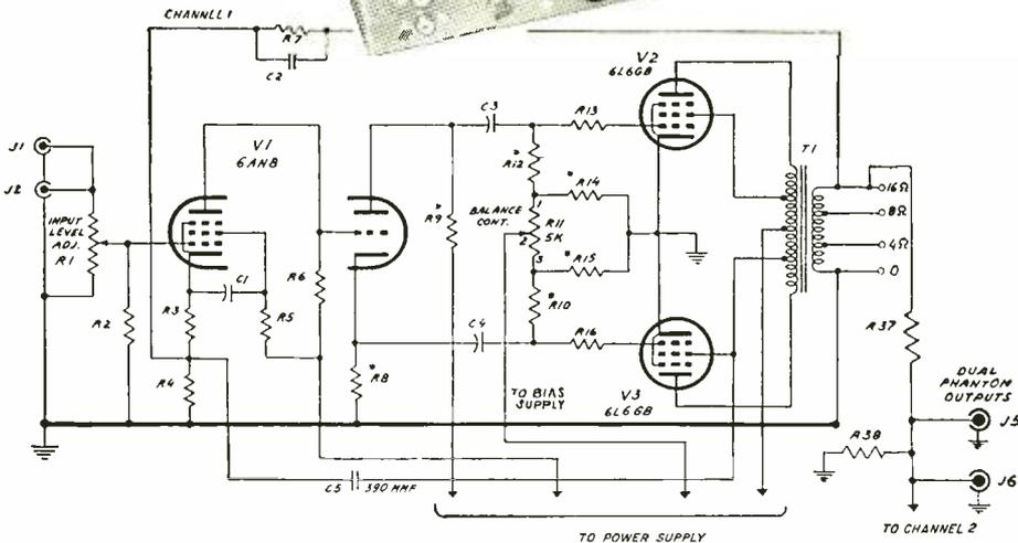
**H**ERE is a fine dual power amplifier for your hi-fi stereo setup. The SPA-55, made by Arkay Radio Kits, Inc., 88-06 Van Wyck Expressway, Richmond Hill, N. Y., offers the hi-fi beginner a top-notch 60-watt monophonic amplifier. And when transition to stereo is desired, dual 30-watt identical amplifiers are available.
