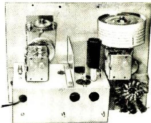
The a.f. unit minus the dial drum is mounted on the main chassis in this photo. Wiring has been completed. All that remains is final assembly.
