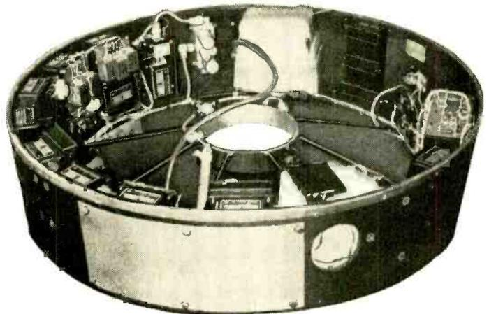
**Instrumented payload** of "Pioneer" moon rocket includes devices for measuring magnetic fields and the temperature of the vehicle's interior.
