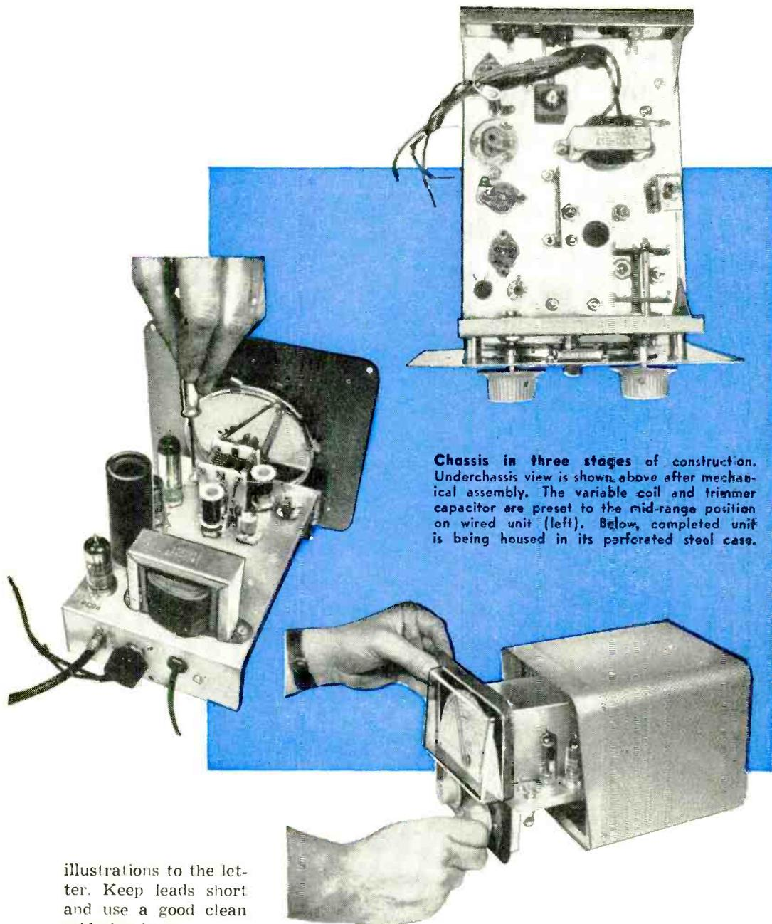
**Chassis in three stages of construction.** Underchassis view is shown above after mechanical assembly. The variable coil and trimmer capacitor are preset to the mid-range position on wired unit (left). Below, completed unit is being housed in its perforated steel case.
