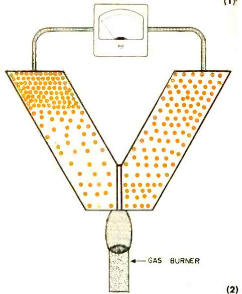
the highest thermoelectric voltage, definitely a desirable trait for power generation.
