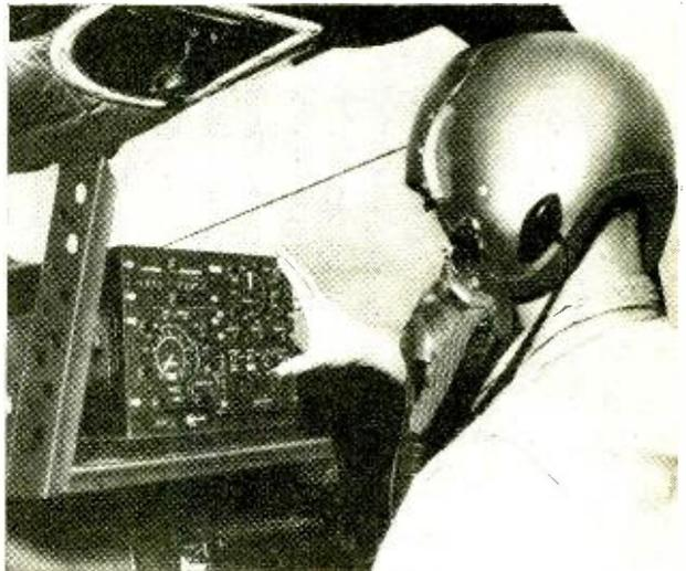
**HOMING PIGEON.** Thanks to Doppler radar, Navy flyers find their way home to their carrier. Here, pilot of A3D bomber adjusts Ryan Aeronautical unit. Instruments show latitude, longitude, ground speed, drift, etc.
