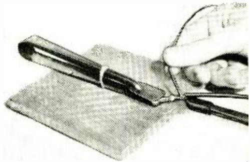
tongs. Simply fasten the tongs to a scrap of wood and wrap a rubber band tightly around the tongs as shown in the photograph.—*Jerome Cunningham, Chicago, Ill.*
