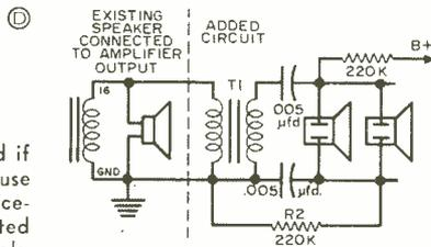
**Alternate circuit** to be used if the circuits of (B) and (C) cause the amplifier to oscillate. Voice-coil leads of T1 are connected to amplifier output terminals.
