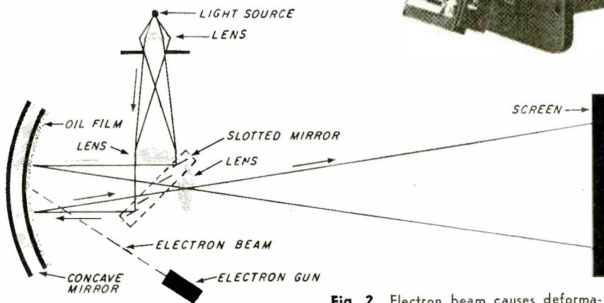
**Fig. 2.** Electron beam causes deformation of the oil film's surface, thus changing reflection angle of light from the light source. Picture is projected between the elements of the "Venetian blind" mirror.
