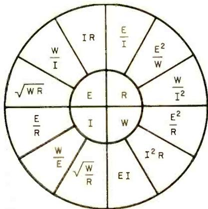
Has Ohm's law got you going around in circles? Take a look at the wheel at left and rotate no more. All of the Ohm's law equations are arranged in one simple, easy-to-read grouping. Simply select the desired unknown ( $E$ ,  $I$ ,  $R$  or  $W$ ) from the inner circle of the wheel, then scan its quarter of the outer circle for the one of the three available equations that applies.
