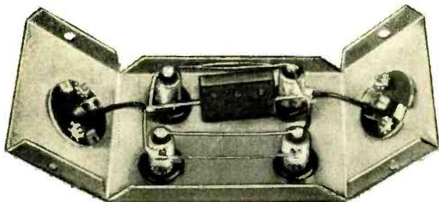
Side panels of cabinet have been folded down only to show internal wiring of Load Box. Note use of rubber grommets to hold pilot lamps and how the wires are soldered directly to the bulbs.
