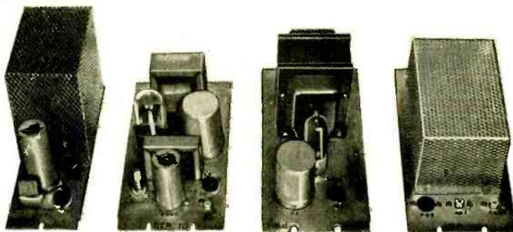
The four modular units in the order that they are installed in the chassis pan. Left to right: transmitter, modulator, power supply, and the converter.
