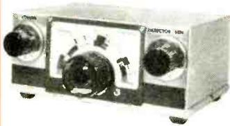
**SHORT-WAVE RECEIVER FOR THE 30-50 MC BAND**—Readers of POPULAR ELECTRONICS have been asking for this! Here are complete plans for an easy-to-build short-wave receiver in the most popular band for ham operators.
