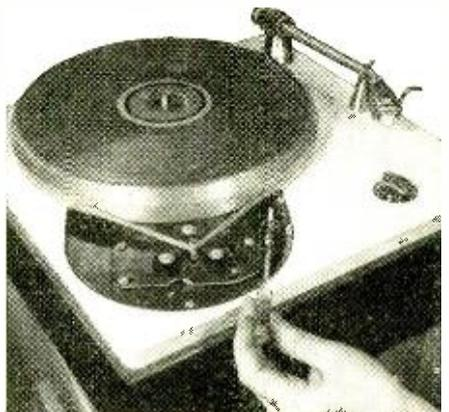
**Rek-O-Kut K-33H** provides a spring-loaded screw adjustment to increase or decrease tension on the belt which drives the platter.
