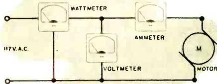
**2** Dewey Dubblecheck, who believes in making all measurements twice, connected a voltmeter and an ammeter to measure the power drawn in this circuit. Using the formula:  $W = E \times I$ , he found that the motor drew 40 watts. He made the measurement again, this time using a standard wattmeter, and read only 30 watts. Dewey is puzzled—are you?
