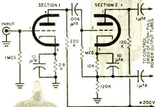
**I**NTENDED for low-level audio use, the new CBS-Hytron 7247 tube is a dual triode designed especially for the "front ends" of audio amplifiers. Special techniques are employed in its manufacture to minimize hum and microphonics.
