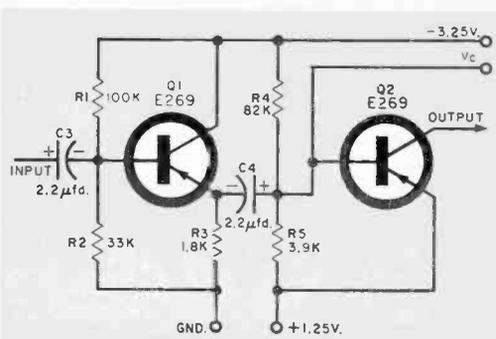
Fig. 1. Schematic of a micro-module audio amplifier. About 1/5" long by 1/3" square, the assembled unit weighs less than a tenth of an ounce, yet provides 32 db gain and 1 mw. power output.
