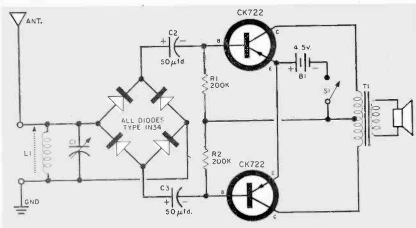
**Fig. 3.** Nurhan Seyhan's receiver circuit features push-pull detection and a push-pull amplifier.
