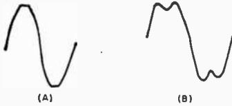
**Fig. 12.** Slight (A) and extreme (B) clipping which occurs when output stage of amplifier is overdriven.
