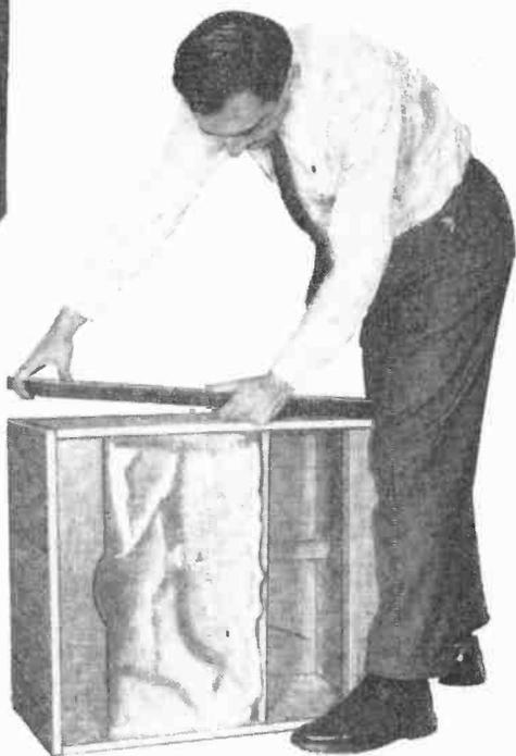
**5** Finishing panel, although not necessary, may be added for the sake of appearance. Four wood screws through cabinet hold 30" x 16" panel in place. Interior of top compartment should be loosely lined with Fiberglas, rock wool, or other acoustical damping material. Cabinet may be used upright as lowboy, finished or unfinished, as desired.
