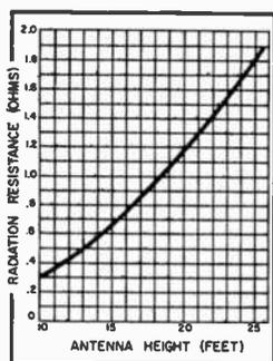
Fig. 1. Radiation resistance of Marconi antennas having heights that vary from 10 to 26 feet.
