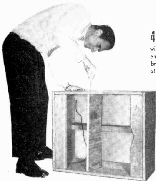
**4** Cabinet divider is fitted next. Exact angle is unimportant, but it should not be mounted parallel with top panel. Glue and two wood screws at each end hold it in place. Slight arc cut out of the top brace enables speaker to mount properly. Front edge of shelf should be flush with front edges of enclosure.
