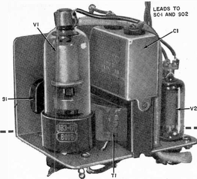
Values of C1 and R4 shown in schematic permit timing periods from five seconds to seven minutes. Capacitor and resistor in parallel with relay coil allows automatic recycling; typical values are 8  $\mu$ fd. and 680 ohms.
