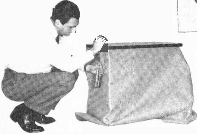
8 Plastic hi-fi grille cloth made by Mellotone is wrapped around cabinet and stapled into place. This material is recommended for speaker enclosures because it is strong, good-looking, and acoustically transparent. After the grille cloth is stapled, legs or a base can also be installed.
