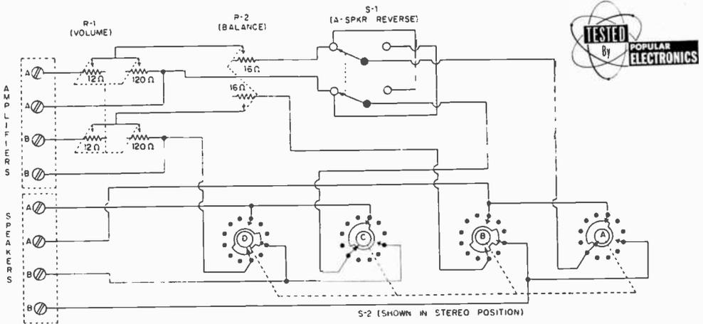
listening to either of the amplifiers on both speakers. The remaining positions provide switching on either channel A only or channel B only for balancing the stereo system.
