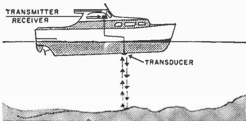
**Fig. 1.** Depth sounders operate on the principle of sound reflection from the sea bottom. A transducer mounted below the waterline alternately sends out a sound pulse and listens for the echo, with the elapsed time shown on some type of indicator.
