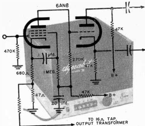
Fig. 4. Dyna "Mark III" power amplifier features a pentode voltage amplifier direct-coupled to a triode split-load inverter. Both functions are handled by one tube, a 6AN8.
