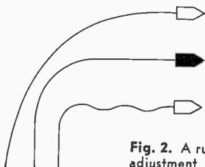
**Fig. 2.** A rudder amplitude adjustment determines how much the rudder will react to a change in course. Top wake shows too small a rudder angle, turn is too slow. Bottom wake shows too great a rudder angle, resulting in oversteering and a fishtail effect. Middle wake shows correct adjustment.
