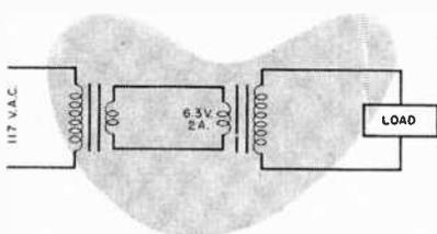
**3** Sam Aveapenny did not want to buy an isolation transformer, so he decided to hook up two filament transformers as shown above. He planned to use the transformers with a 200-watt load so he employed the formula:  $P = IE$ . Figuring that the voltage was about 120 volts, he arrived at:  $120x = 200$ ,  $x = 1.66$ . Since the transformers were rated at 2 amperes each, he went ahead with the job. To his surprise, the transformers burned out. Why?
