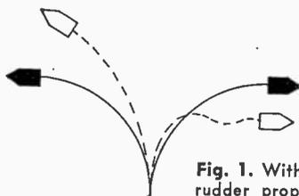
**Fig. 1.** With left and right rudder properly equalized, the autopilot should move the boat in identical turns to the left or to the right. Dotted lines show the effect of unequal rudder control.
