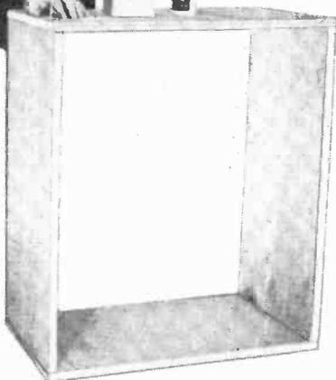
**1** Sides, top and bottom of enclosure are assembled using a good wood glue and 8d (penny) finishing nails. All joints are butted with five or six nails per joint. Design of cabinet makes use of cleats unnecessary.
