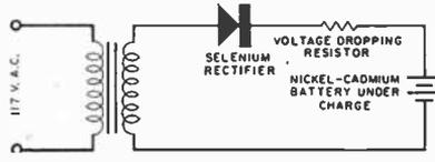
**Fig. 4.** Typical simple rectifier circuit employed to reactivate rechargeable batteries.
