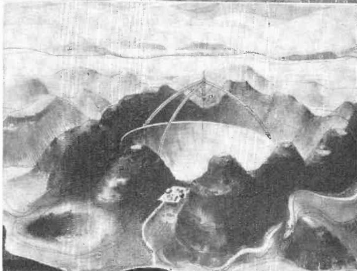
**This giant radio telescope** is being built for the U. S. Naval Research Laboratory in Sugar Grove, W. Va. The huge reflector will be 600' wide, twice the length of a football field. The entire 20,000-ton installation will rotate on rollers which ride circular tracks on the ground, allowing the dish to be aimed at any point in the sky above the horizon.
