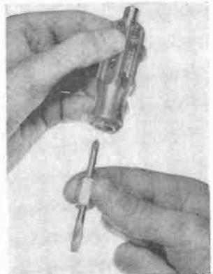
applied to the rear panels of TV sets. As a ⅜" nut driver, it can be used for fastening antenna fittings. Price, \$2.30.
