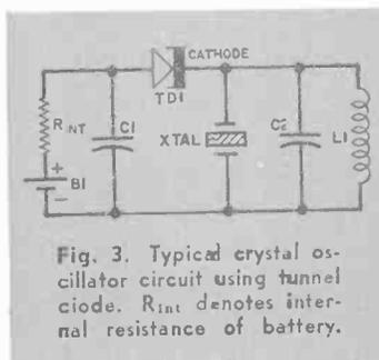
Fig. 3. Typical crystal oscillator circuit using tunnel diode.  $R_{INT}$  denotes internal resistance of battery.
