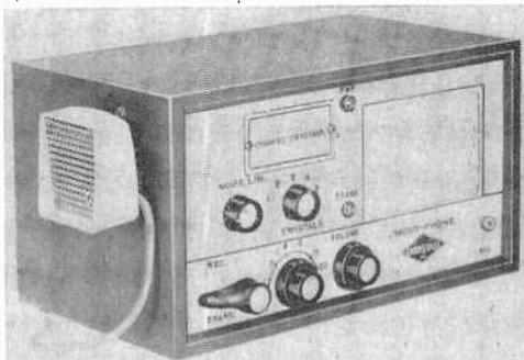
Island City 1, N. Y. Features of the "Radio-Phone" include a superhet variable-tuning receiver, a crystal-controlled transmitter, and a power pack for operation with either 6 or 12 volts d.c. The unit is furnished with one crystal, a microphone, mobile mounts, and a license application form. Price, \$99.95.
