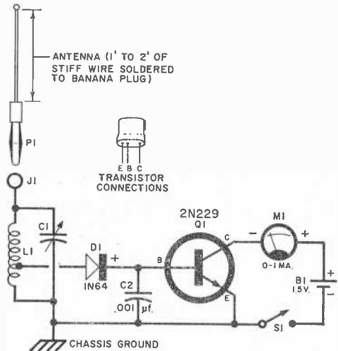
**Schematic diagram** of field strength meter. Exact values of *C1* and *M1* will depend on desired range and sensitivity of unit; switch *S1* can be omitted if antenna is unplugged whenever meter is not in use.
