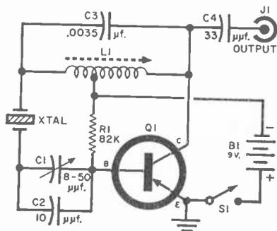
**Fig. 3.** Circuit of Heath Company's Type HD-20 crystal-controlled calibration kit. Device will check frequencies from 100 kc. to 54 mc.
