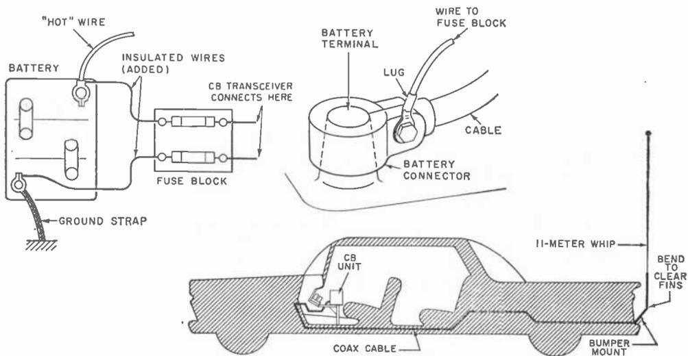
**Fig. 2.** Fuse block between battery and transceiver will protect the CB rig; one or two fuses can be used, depending on requirements. Use heavy insulated wire for all battery connections, and coaxial cable to connect the transceiver to the antenna.
