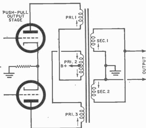
Fig. 4. Circuitry of Dyna hi-fi output transformer. Interleaved and counter-balanced windings help reduce leakage.
