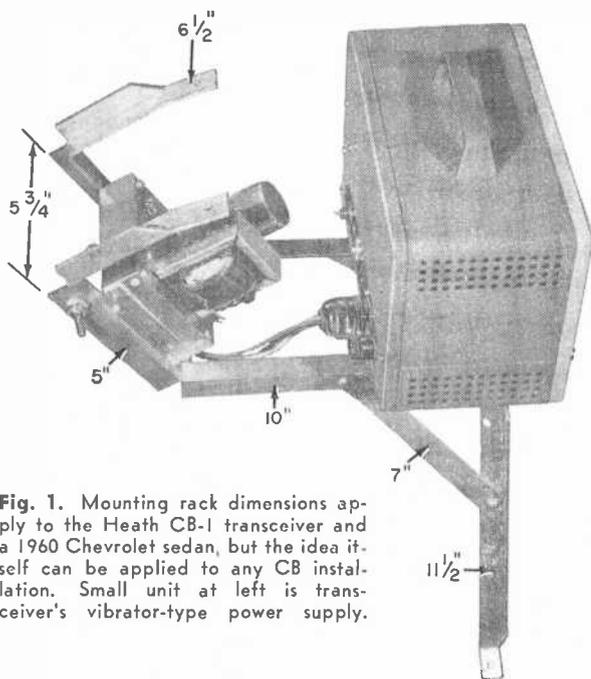
**Fig. 1.** Mounting rack dimensions apply to the Heath CB-1 transceiver and a 1960 Chevrolet sedan, but the idea itself can be applied to any CB installation. Small unit at left is transceiver's vibrator-type power supply.
