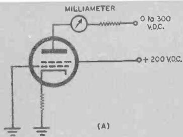
Fig. 1. Tetrode vacuum tube circuit (A) displays curves (B) somewhat like those of a tunnel diode. See text.
