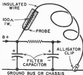
length of flexible, insulated wire; an alligator clip; a 100-ohm, 1-watt resistor; and a test probe. Attach the alligator clip to one end of the wire, and solder one
