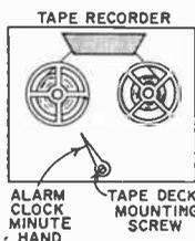
pointer loosely under a mounting screw on the tape deck as shown. Point the hand toward the take-up reel when you start recording, and point the pointer to the other reel when you start to tape the other way. You'll have no trouble recognizing the take-up reel even if you're in the middle of a reel of tape.—*Art Collins, Buffalo, N. Y.*
