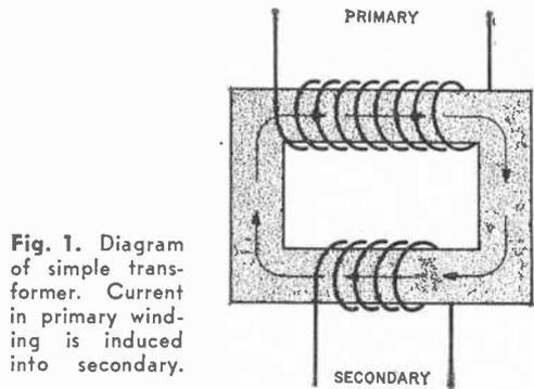
**Fig. 1.** Diagram of simple transformer. Current in primary winding is induced into secondary.
