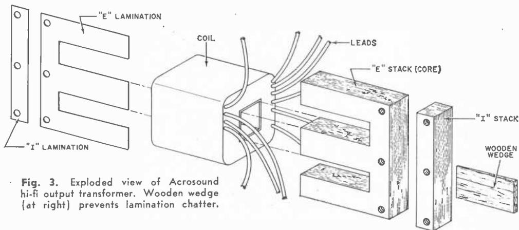
Fig. 3. Exploded view of Acrosound hi-fi output transformer. Wooden wedge (at right) prevents lamination chatter.
