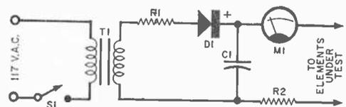
**Fig. 3.** Inter-electrode resistance measuring circuit in Heath TT-1 tester. Circuit functions as an ohmmeter to measure inter-electrode resistances to 20 megohms; external ohmmeter may be used instead.
