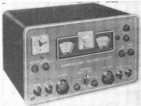
its own power supply, requiring only an external speaker or earphones. The HQ-180 features an 18-tube superheterodyne circuit with automatic noise limiter and
