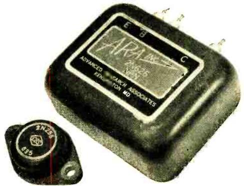
"Composite" transistors, introduced by Advanced Research Associates, have extremely high gain. Note size of unit at left compared with a conventional power transistor.
