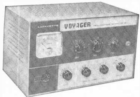
switching on 80 through 6 meters. The unit runs 120 watts c.w. input on 80 through 10 meters; 85 watts c.w. on 6 meters; and 70 watts phone on all bands. Its straight-through class C final assures highest efficiency. Priced at \$109.50, the HE-25 is
