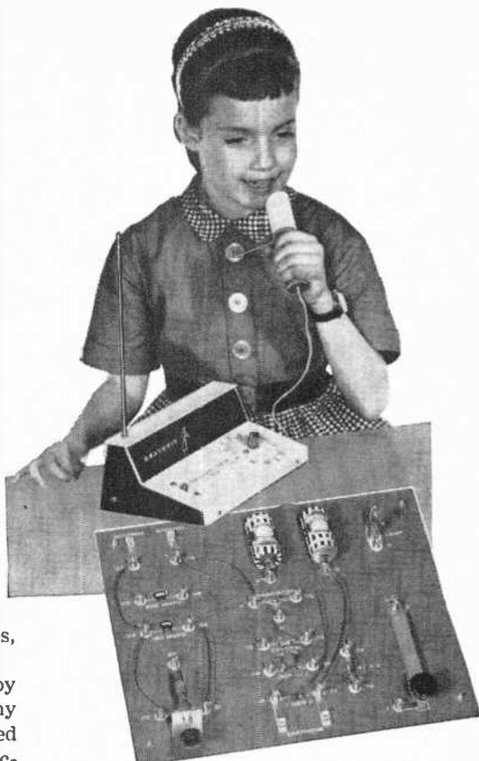
**Electronic toys** in easy-to-build kit form are now available from the Heath Company. Requiring no soldering, the kits feature pre-cut and pre-stripped wire for connection to screw terminals.
