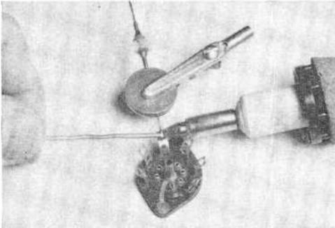
tect diodes and transistors from the heat of your soldering iron. The heat will not harm the coins either, but you can use a couple of scraps of copper instead if you wish. Small iron washers will also do the trick, but with reduced efficiency.
