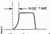
Fig. 2. Square-wave "rise time" is length of time required for wave to reach its maximum positive or negative peak. Diagram purposely shows exaggerated rise time.
