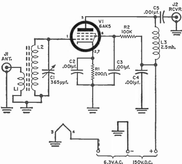
The DX booster uses a ferrite loopstick, tuned by capacitor C1, as its antenna coil. Capacitor C5 couples output to receiver.
