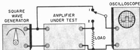
Basic circuit for square-wave testing is shown above. With the switch in position 1, check both generator and oscilloscope for good square-wave response. Then flip to position 2 to check the amplifier under test. The waveforms below cover most common amplifier troubles.
