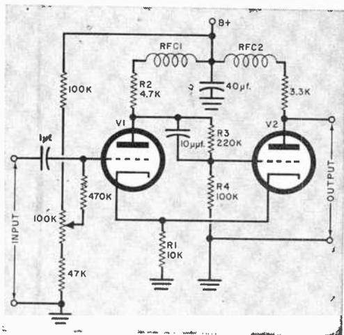
Fig. 3. Schmitt Trigger circuit employed in Heath AG-10 sine-/square-wave generator.
