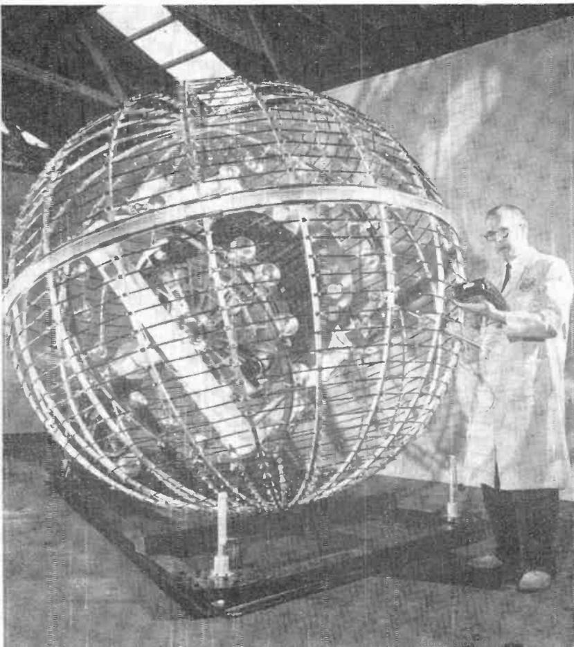
Spherical "cage" designed to produce magnetic fields resembling those of the earth was used in pre-launching tests of Tiros II. Here, Warren P. Manger, of the RCA Astro-Electronics Division, takes reading of magnetic effect within the wired "cage," preparatory to rotating the satellite on its mount for study of the orientation system.
