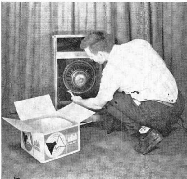
Check mounting surface before putting the speaker in place to be sure that the surface is not warped.
