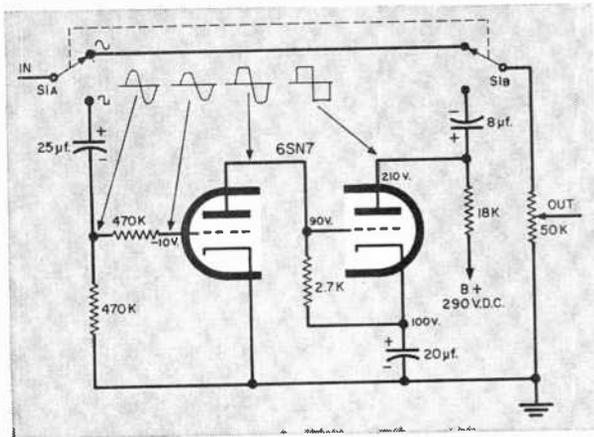
Fig. 1. Simplified clipper circuit in EICO 377 sine- and square-wave generator. Switch is shown in sine-wave position.
