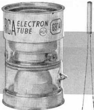
Image tube (far left) converts invisible infrared into visible light; the World War II "snooper-scope," which enabled troops to see in the dark, employed such a detector. Modern single-crystal infrared detector (left) is a byproduct of transistor development; unit produces output voltage in proportion to amount of infrared radiation falling upon it. Both devices are products of Radio Corporation of America.
