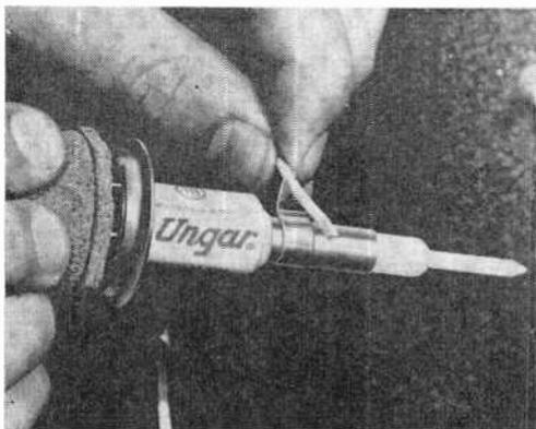
Ave., Los Angeles 66, Calif., you can strip insulation from wire while soldering. The stripping clip fits onto the barrel of a soldering tip, and will melt all rubber or plastic insulation from 8- to 24-gauge wire without nicking or scoring the strands. Clips are available in three different shapes at 75 cents each.
