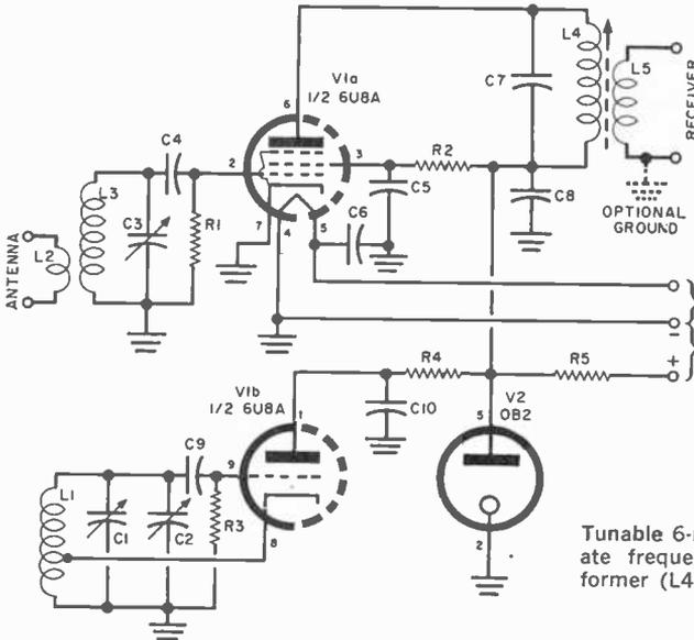
Tunable 6-meter converter operates with intermediate frequency near 7 mc. Slug-tuned i.f. transformer (L4-L5) is hidden behind tube V2 in photo.
