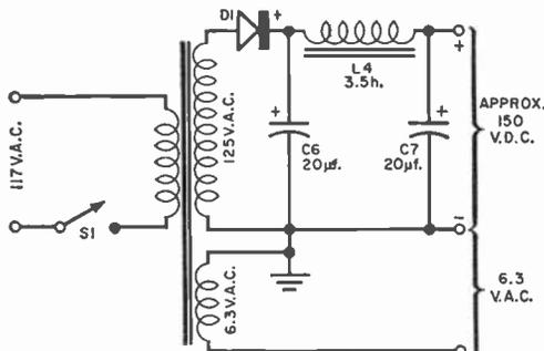
ground for B- and one of the 6.3-volt a.c. output terminals.
