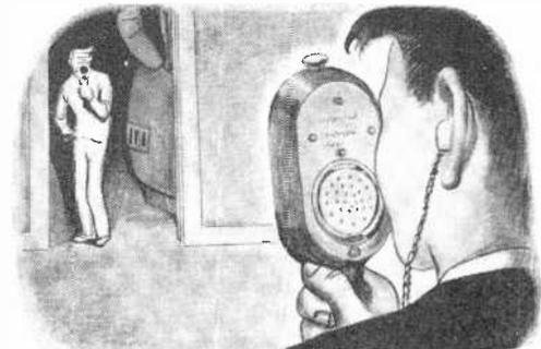
phones' were developed by the Infrared Industries of Waltham, Massachusetts. They permit talking over distances of several hundred feet by means of beams of infrared radiation.
