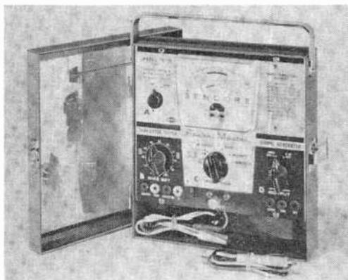
the tester is an r.f.-a.f. signal generator and voltmeter-milliammeter for troubleshooting purposes. The Transi Master is supplied with a test probe that connects
