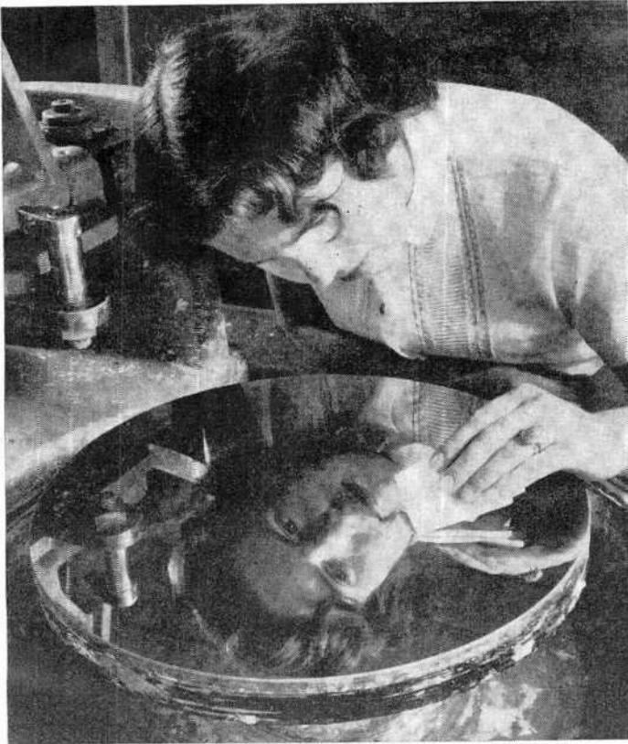
Infrared “picture window” produced by scientists at Hughes Aircraft is solid germanium casting 15” in diameter and ½” thick. Optically ground and polished, it is opaque to ordinary light but refracts infrared rays much as a glass lens collects and focuses rays from visible part of spectrum. Used in missile detection systems, the casting is made from 9½ pounds of germanium, and is valued at approximately six thousand dollars.
