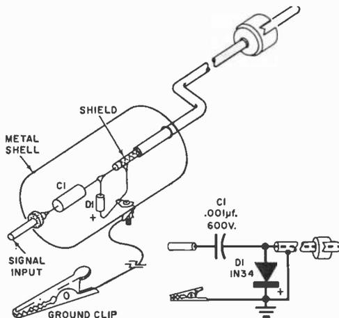
long or more; the ground lead connected to the alligator clip should be about a foot long. To use the probe, fasten the clip to the set being tested, connect the output cable to the input of any amplifier, and touch the signal input pin to the grid and plate of each stage until the inoperative stage is found. The quality of the signal may also be judged from the sound reproduced as the probe is moved from stage to stage.
