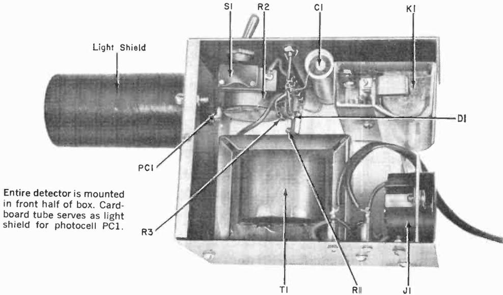
Entire detector is mounted in front half of box. Card-board tube serves as light shield for photocell PC1.
