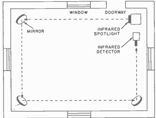
frared beam is focused on photocell *PCI*; you may have to put a larger lamp in the spotlight for long beam lengths or when mirrors are used.
