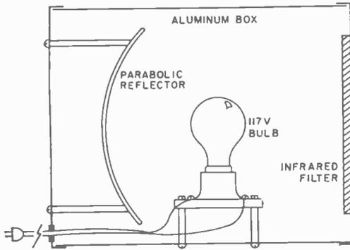
Infrared spotlight's box should have lightproof air vents. Use high-wattage lamp for long beam lengths.
