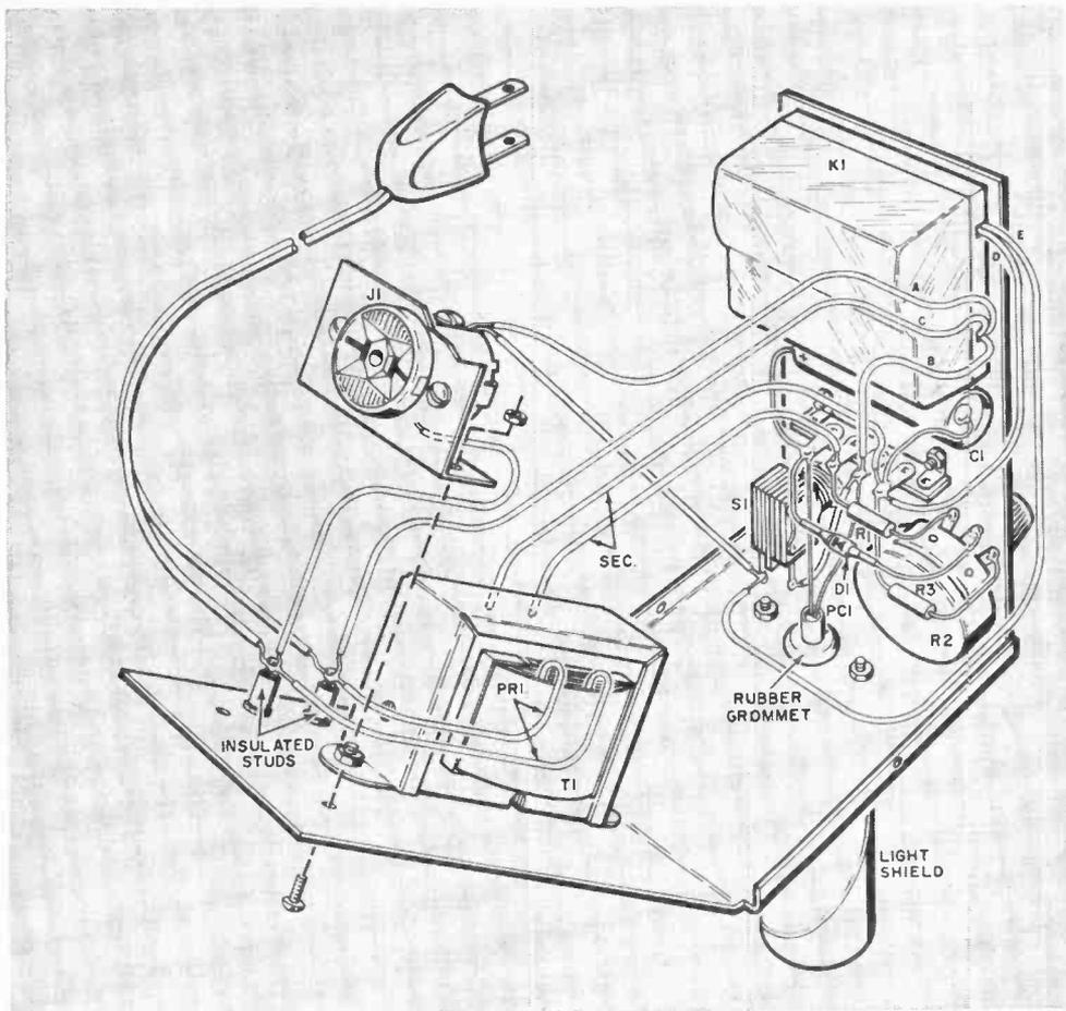
Infrared detector wiring is simple and straightforward, although photocell PC1 requires special consideration. See text for details.
