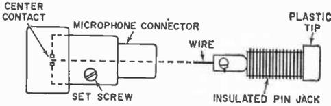
phone connector terminal hole. In any case, clip off the excess lead protruding through the hole and tighten the connector's setscrew on the pin jack's plastic body.
