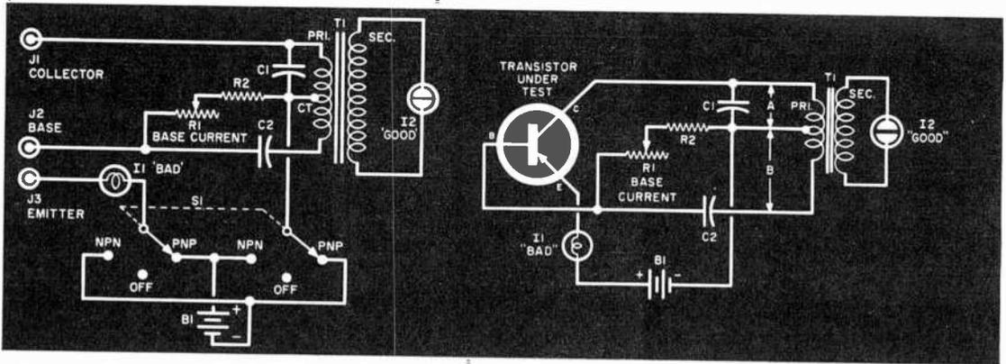
Actual schematic of the tester (above) and simplified schematic (right). See How It Works.
