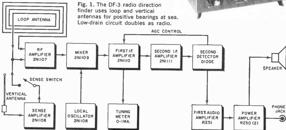
Fig. 1. The DF-3 radio direction finder uses loop and vertical antennas for positive bearings at sea. Low-drain circuit doubles as radio.
