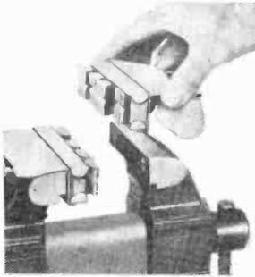
of adjustable jaws available from Mid-American Import Co., Inc., 1919 Champa St., Denver 2, Colo. Steel fingers in each jaw adjust to hold any shaped object firmly. The "Uni-Grips,"
