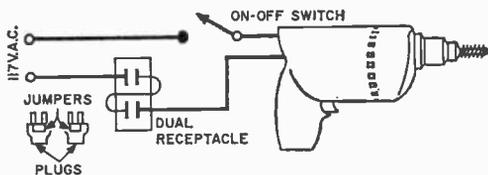
to a dual a.c. receptacle as shown in the schematic. To operate the interlock, make a couple of jumpers by connecting a wire across the terminals of two long-handled male plugs; when both plugs are inserted in the receptacle, the power tool is turned on. Hide the plugs when the tool is not in use for safety's sake. The on-off switch shown here can be left out of the circuit if your power tool already has a built-in switch.
