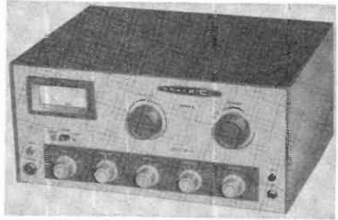
well as the General Class amateur. Power input is 90 watts peak, carrier-controlled phone or c.w., on amateur bands from 80 through 10 meters, but the unit can be run at reduced power for Novice operation. Other features include a built-in low-pass filter for harmonic suppression, a neutralized final for high stability, and grid-block keying. Price: \$82.95. (Heath Co., Benton Harbor, Mich.)
