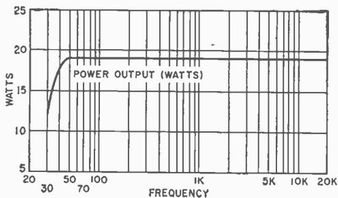
Power response of amplifier is shown above for a Harmonic distortion of 2%. Note that due to use of a special output transformer the output is flat from 48 to 20,000 cycles. Harmonic distortion at 18 watts output at 30 cycles is less than 3%.
