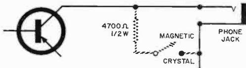
and either type of phone can be selected by flipping the switch. Open the switch when using magnetic phones, and close the switch when using crystal phones. The purpose of the resistor is to pass d.c. to the collector of the transistor
