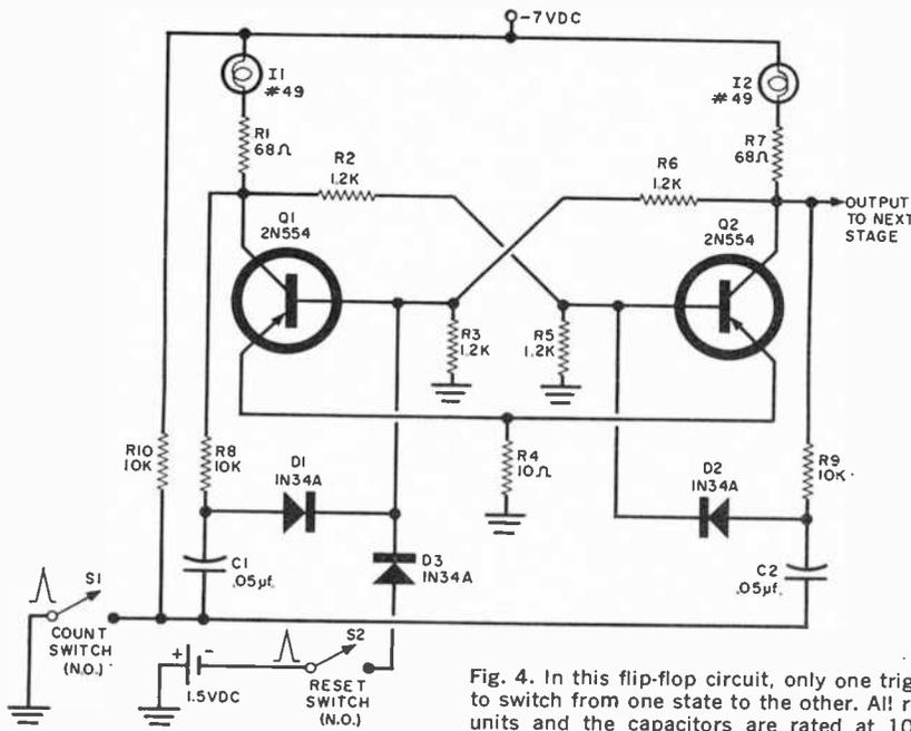
Fig. 4. In this flip-flop circuit, only one trigger input is needed to switch from one state to the other. All resistors are  $\frac{1}{2}$ -watt units and the capacitors are rated at 10-w.v.d.c. minimum.
