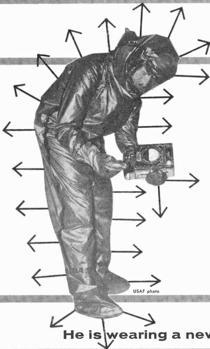
This four-layer suit consists of a neoprene-coated nylon coverall with attached mittens, boots, and headpiece to prevent arcing; two inner layers of silverized cloth to reflect radiation; and a cotton liner to protect the silverized cloth. It is designed to be worn by radar technicians at BMEWS radar stations.
