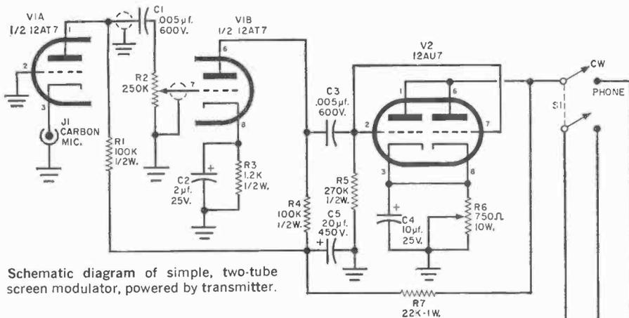
Schematic diagram of simple, two-tube screen modulator, powered by transmitter.
