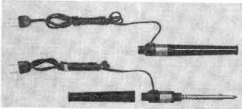
Broadway, Hewlett, N. Y.), has a removable handle that covers the tip when it's not in use. After a soldering job, you can switch the handle around and place the iron right in your tool box (or even
