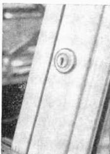
Mounting details of the alarm system are shown in these photographs. Door switch is mounted on frame just below dome-light switch (at left, above). Terminal strip for alarm and accessory wiring is mounted below the dash (center). Alarm siren (at right, above) is located behind the radiator under the hood. The key-operated switch that controls the system (below, left) fits neatly on the doorpost.
