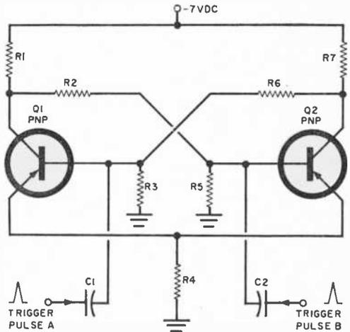
In many flip-flop circuit applications,  $R4$  is bypassed by a high-value electrolytic capacitor,  $C1$ , to insure constant voltage on the emitters of  $Q1$  and  $Q2$  during the flip or flop of the multivibrator.
