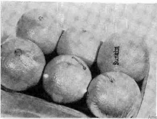
Packaging film made by electron-irradiating low-density polyethylene is clear, strong, and glossy. A blast of hot air shrinks the film to make an attractive, skin-tight wrap that prevents fruit from shifting or being bruised.
