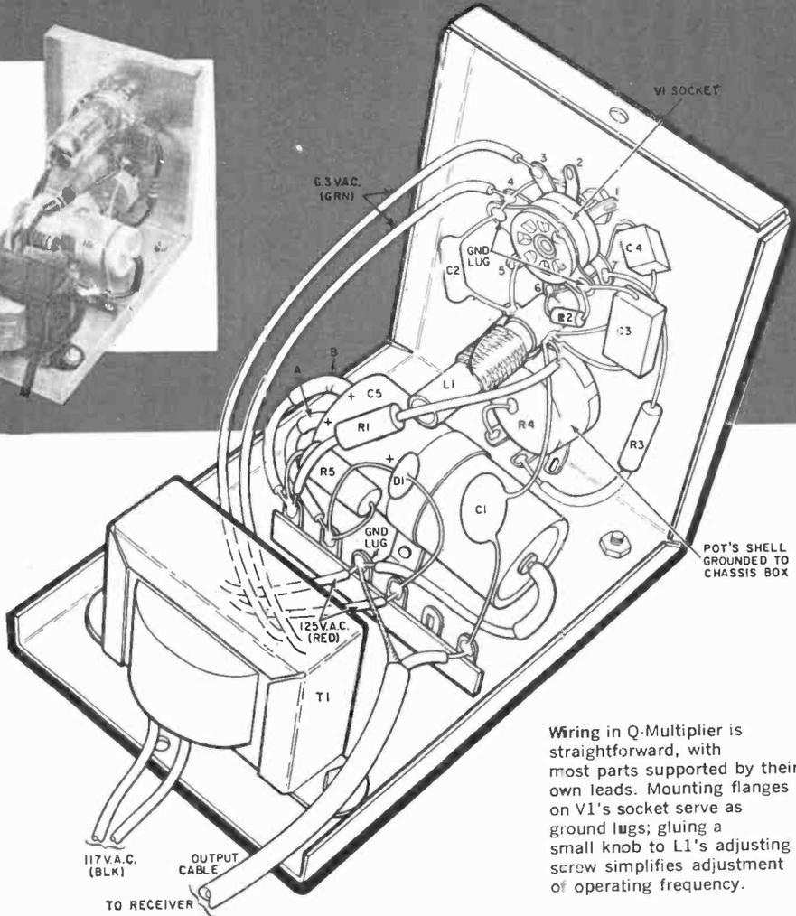
Wiring in Q-Multiplier is straightforward, with most parts supported by their own leads. Mounting flanges on V1's socket serve as ground lugs; gluing a small knob to L1's adjusting screw simplifies adjustment of operating frequency.
