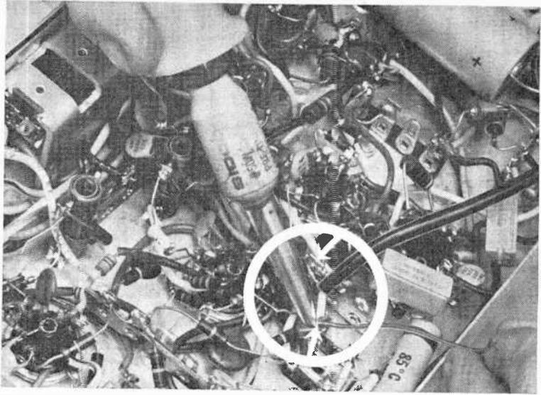
kc. i.f.'s, do not modify  $L1$ , but change capacitors  $C2$  and  $C3$  to  $680 \mu\text{f.}$  and  $.0025 \mu\text{f.}$ , respectively.
