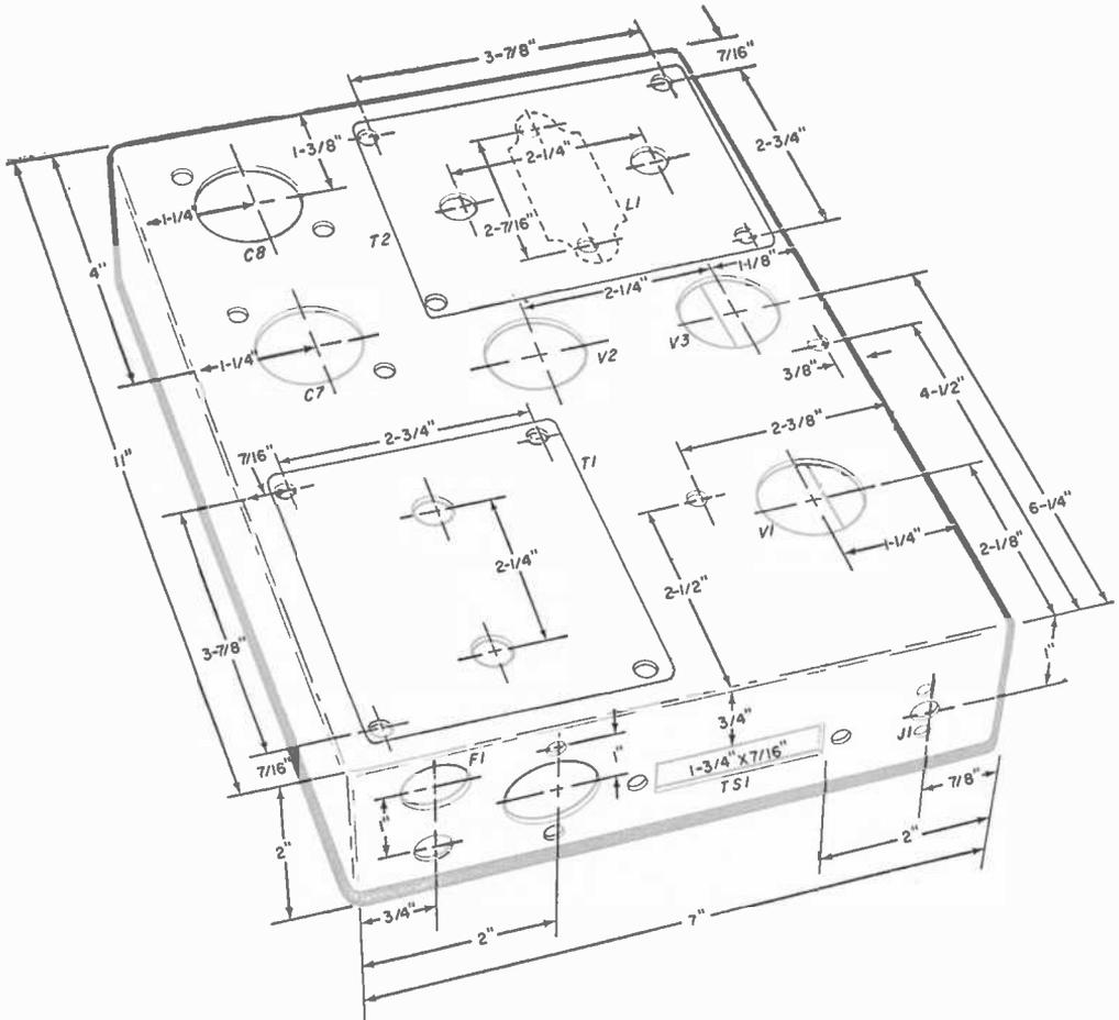
Drill and punch the amplifier's chassis before mounting any components. Filter choke L1 (dashed line) mounts under chassis below transformer T2.
