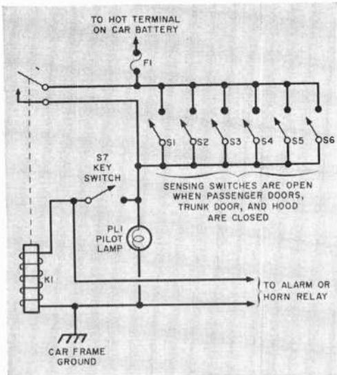
The alarm operates and relay K1 locks up when both key-operated switch S7 and any sensing switch (S1 to S6) are closed. Sketch at right, above, shows suggested spots for placing sensing switches.
