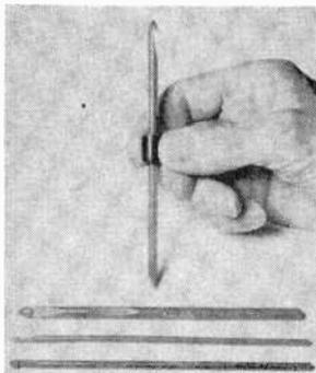
Use the hooked end of a needle to manipulate dial cords in tight corners; file the other end to fit tuning slugs and screws on i.f. transformers. A small "knob" can be formed in
