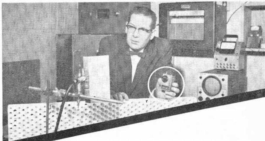
A dosimeter developed by Dr. A. W. Richardson of Saint Louis University is used to measure r.f. radiation. Worn by a maintenance technician, it sounds an audible tone when r.f. intensity becomes dangerous.
