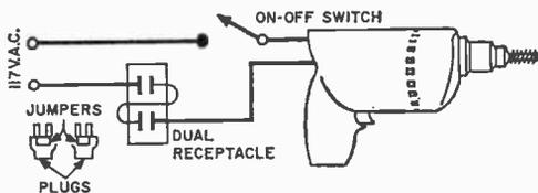
to a dual a.c. receptacle as shown in the schematic. To operate the interlock, make a couple of jumpers by connecting a wire across the terminals of two long-handled male plugs; when both plugs are inserted in the receptacle, the power tool is turned on. Hide the plugs when the tool is not in use for safety's sake. The on-off switch shown here can be left out of the circuit if your power tool already has a built-in switch.
