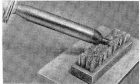
to a piece of plywood which can be screwed or nailed to an adjacent wall. To use the brush, simply wipe the iron's tip on the bristles; sludge and dirt will come off, and the tip will do a better soldering job.
