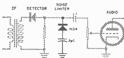
oped across the detector load resistor, and it conducts until the capacitor charges to the value of this voltage. At this point, the bias on the limiter diode drops to zero.
