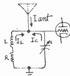
ain't so. The resistor,  $R$ , causes a phase shift in the coil leg of the tuned circuit. Since this resistance is small, the phase difference between the currents  $I_C$  and  $I_L$  is slightly less than 180 degrees, and summing up these two currents will not give us zero. A very small current will be left. Back to friend Kirchhoff . . ."
