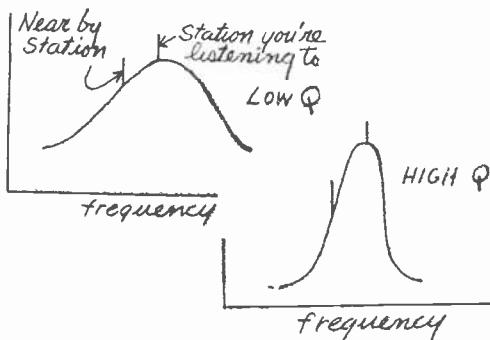
correctly, the station you want to listen to will be right on top of the curve. But note that a nearby station, which you don't want to hear, will have almost the same signal strength—the tuned circuit will not reject it. This shows poor selectivity." Pointing to the top drawing, Ken added, "That's your receiver!"
