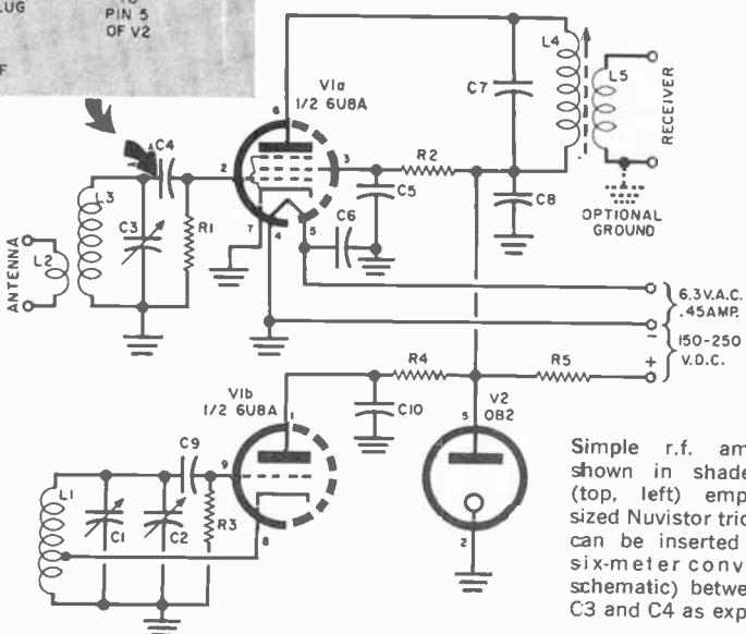
Simple r.f. amplifier stage shown in shaded schematic (top, left) employs peanut-sized Nuvistor triode. The stage can be inserted in circuit of six-meter converter (large schematic) between capacitors C3 and C4 as explained in text.
