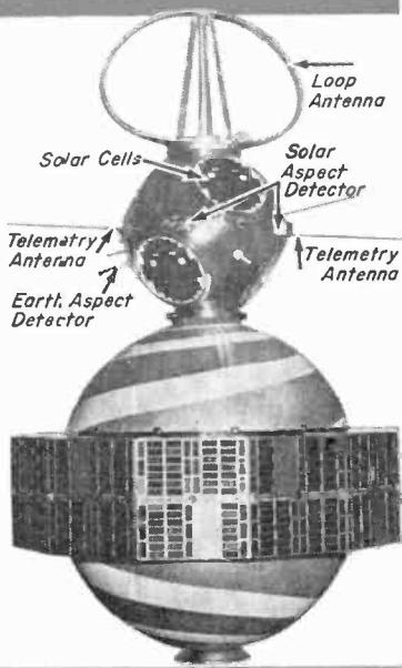
The "neck" joining Transit III-B and the NRL LOFTI satellite failed to separate after February 21 launch.
