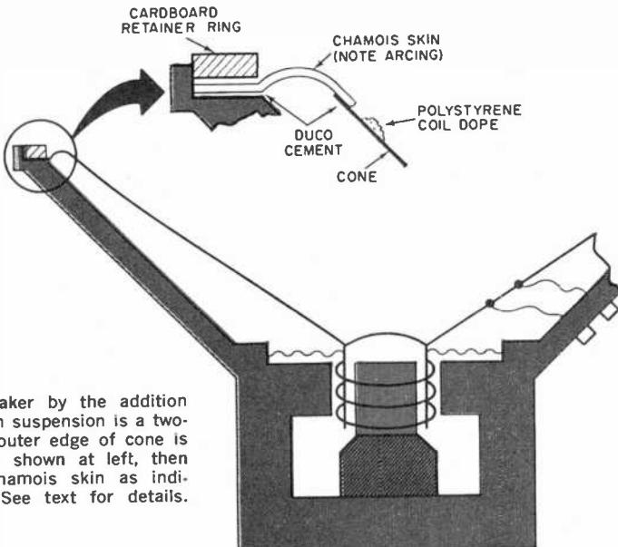
Modifying a speaker by the addition of a chamois-skin suspension is a two-step procedure; outer edge of cone is first removed as shown at left, then replaced with chamois skin as indicated at right. See text for details.
