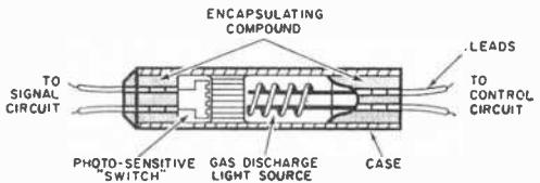
Fig. 1. Cross-sectional view of Raytheon's new Rayistor, a unique device which combines electro-optical techniques with a semiconductor element.
