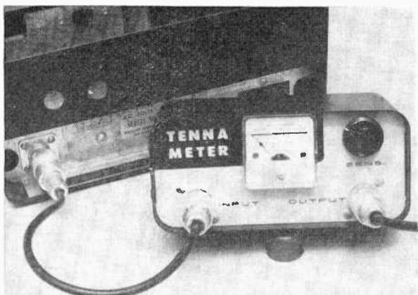
Globe output meter serves as monitor and modulation check. It is left in transmission line at all times.
