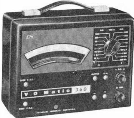
cise readings, and the meter is protected against extreme overload. Sensitivity is 20,000 ohms per volt d.c., 5000 ohms per volt a.c. The unit covers a.c. and d.c. volts, d.c. current, a.f. (output), and resistance in 25 ranges; 18 separate overlay meter scales are provided for supplementary ranges. Price, \$59.95; an optional leather carrying case sells for \$11.95.
