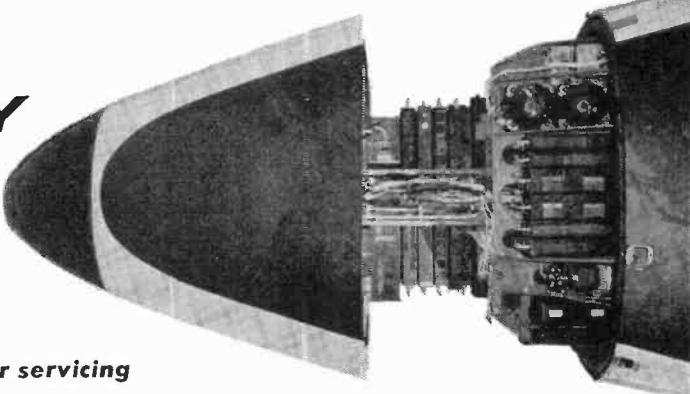
THE NEW four-engine "JetStar," Lockheed Aircraft's entry into the pint-sized jet transport field, has a nose for electronics.
