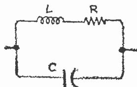
Larry studied the drawing for a moment. "So receiver tuned circuits are made up of coils, capacitors, and resistors?"
