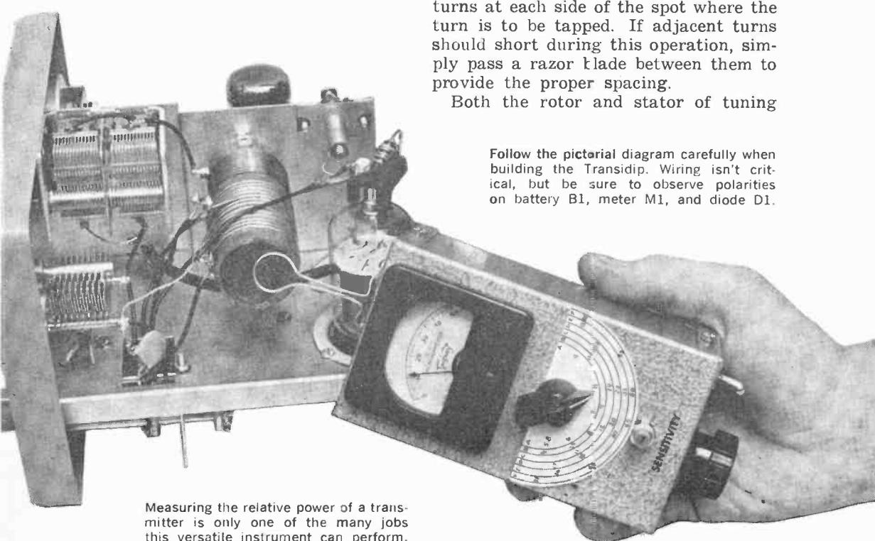
Measuring the relative power of a transmitter is only one of the many jobs this versatile instrument can perform.
