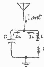
"Do you recall Kirchhoff's law about currents that enter and leave any point in a circuit adding up to zero? Well, at resonance, since the inductive and capacitive reactances are equal, the currents in L and C are also equal but opposite in phase; so they add up to zero. Now, if  $I_L$  and  $I_C$  add up to zero at resonance, what is the value for  $I_{ant}$ ?"
