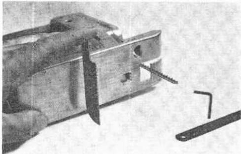
tute from a standard hacksaw blade. Break off a piece of the hacksaw blade and grind it down to fit into the power saw chuck. The blade's tip should also be rounded off to make cutting starts easier.
