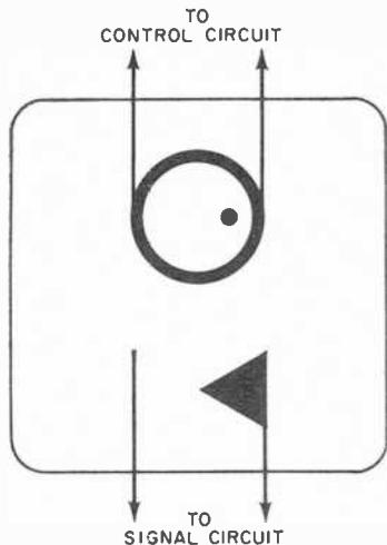
Fig. 2. Schematic symbol for the Rayistor. Note that there isn't any electrical connection between the control and signal circuits.
