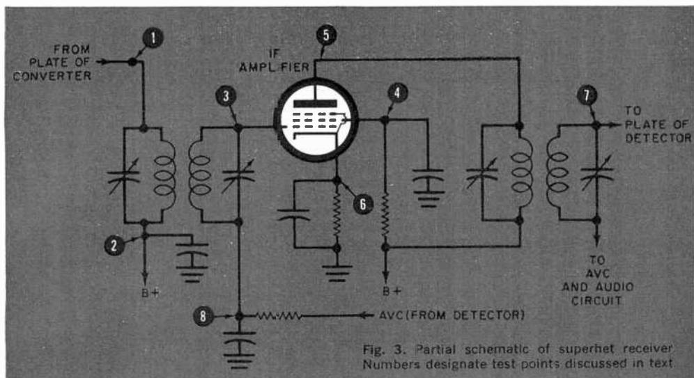
Fig. 3. Partial schematic of superhet receiver. Numbers designate test points discussed in text.
