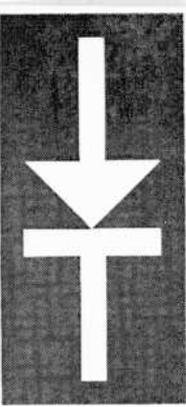
however, the nonlinear resistance also makes it difficult to specify any other diode characteristic. For instance, a vacuum diode can be rated for 300 milliamperes of current, and this will be true at any voltage. Before a semiconductor diode can be rated, however, you must specify the voltage.
