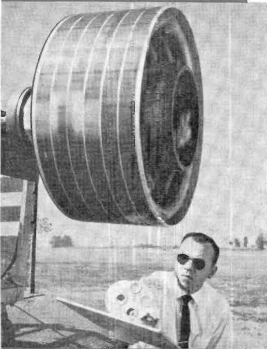
Spinning satellite, built by Hughes Aircraft, is an "active" repeater. It weighs 32 pounds and is powered by silicon cells.
