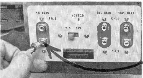
Hooking up is a simple matter with most decks - on the Sony 262-D, jacks are located on a convenient plate with a switch to select record or play-back functions.
