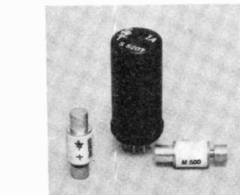
Packaging of diodes in tube shells permits replacement of 5U4, 5W4, 5Y3, 6X4 and other rectifiers. Cartridge-cased diodes are used in the newer TV sets.
