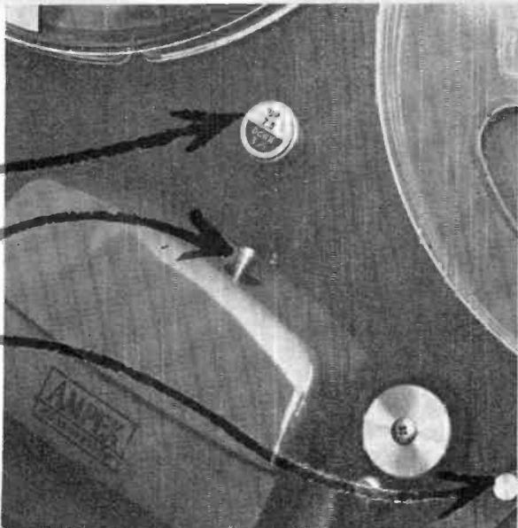
Screwdriver adjusts take-up tension on Heathkit AD-70
