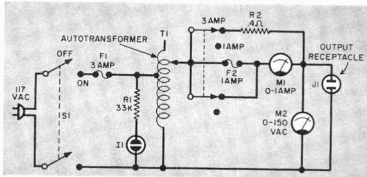
by making it fail immediately with a shot of extra-high line voltage. Want to know how much power a piece of apparatus draws? Plug it into the supply and multiply the voltage and current meter readings. You can even use the supply to reduce the power of a heavy-duty soldering iron (if it doesn't draw more than 3 amperes) to the 6 or 8 watts suitable for transistor work.
