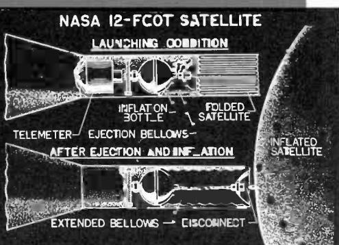
Explorer IX was carefully packed into nose of Scout I rocket and launched by NASA. Test was only partially successful.
