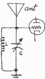
Ken continued with his explanation. "First off, let's see what happens at the resonant frequency. The tuned circuit behaves like a very high impedance or high-value grid resistor at this frequency, and very little of the signal picked up by the antenna passes to ground through the tuned circuit. Instead, the control grid of the vacuum-tube stage connected to the top of the tuned circuit sees nearly all of this signal and amplifies it."
