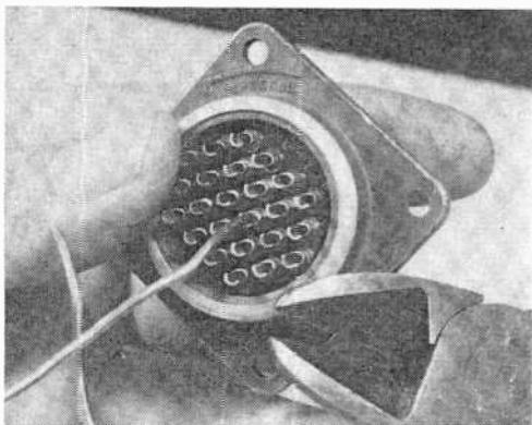
gently insert the wire (tinned) as the solder melts. A piece of spaghetti which has been slipped over the wire prior to soldering can be used to cover the joint.
