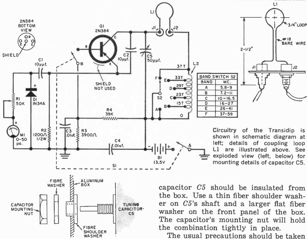
Circuitry of the Transidip is shown in schematic diagram at left; details of coupling loop  $L_1$  are illustrated above. See exploded view (left, below) for mounting details of capacitor  $C_5$ .
