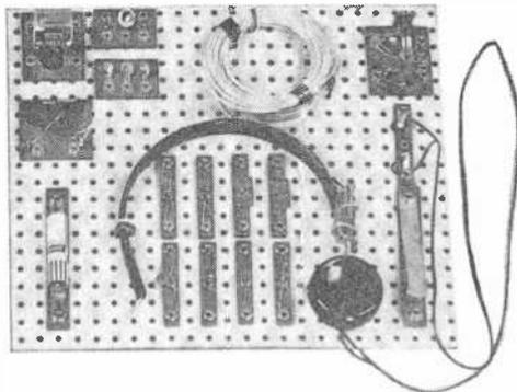
be built with the “Electronic Laboratory” manufactured by *Superex Electronics Corp.* (4 Radford Place, Yonkers, N. Y.). All the parts are provided—the only extra equipment you’ll need is a screwdriver, since the pre-mounted components are equipped with solderless screw connections and all connecting leads are pre-cut. Price, \$11.95.
