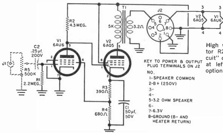
High value of plate load resistor R2 is key to "starved circuit" of V1. Shaded components at left in schematic comprise optional gain control circuit.
