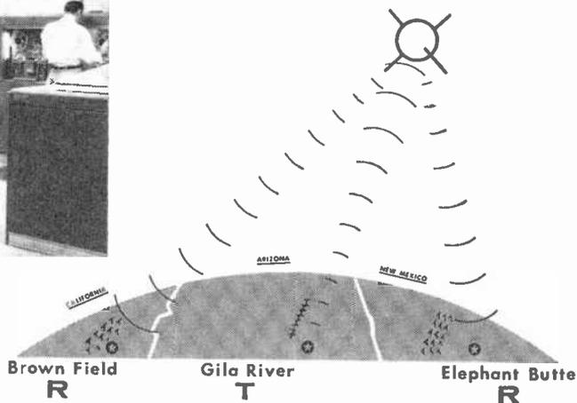
ground tracking station, a "command signal" activates the recorder, broadcasting the information on 107.97 megacycles. Rated at 125 milliwatts, the 107.97-mc. signal should be heard without difficulty on an average FM tuner.
