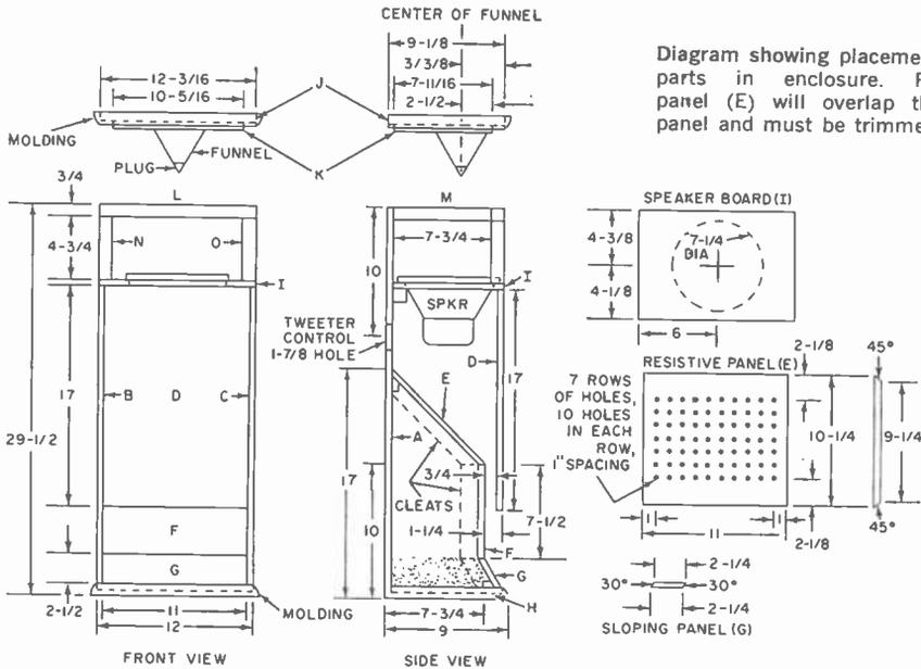
Diagram showing placement of all parts in enclosure. Resistive panel (E) will overlap the duct panel and must be trimmed to fit.
