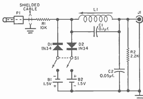
Placement of parts and wiring details for the "Ear Saver" are shown above. Capacitor *C2* can be increased to 0.1  $\mu$ f. to reduce high-frequency background noise on c.w. signals. Experiment with the value of resistor *R2*; with some headphones, this value should be changed, or the resistor eliminated.
