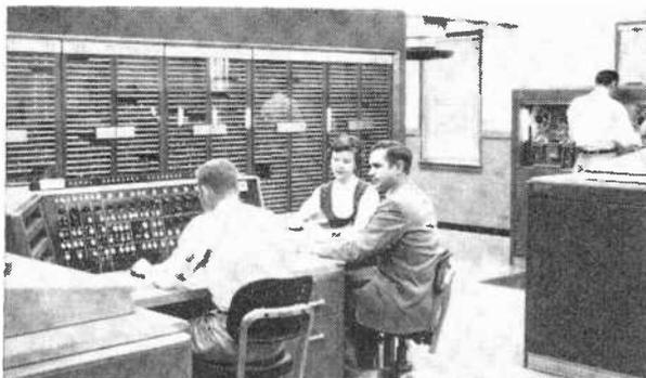
The U.S. Navy maintains a space surveillance system (NAVSPASUR) which has been in operation since 1959. It detects, tracks, identifies and determines the orbits of all non-transmitting space objects. Orbit computations are performed by the Naval Ordnance Research Calculator (NORC) at Dahlgren, Va.
