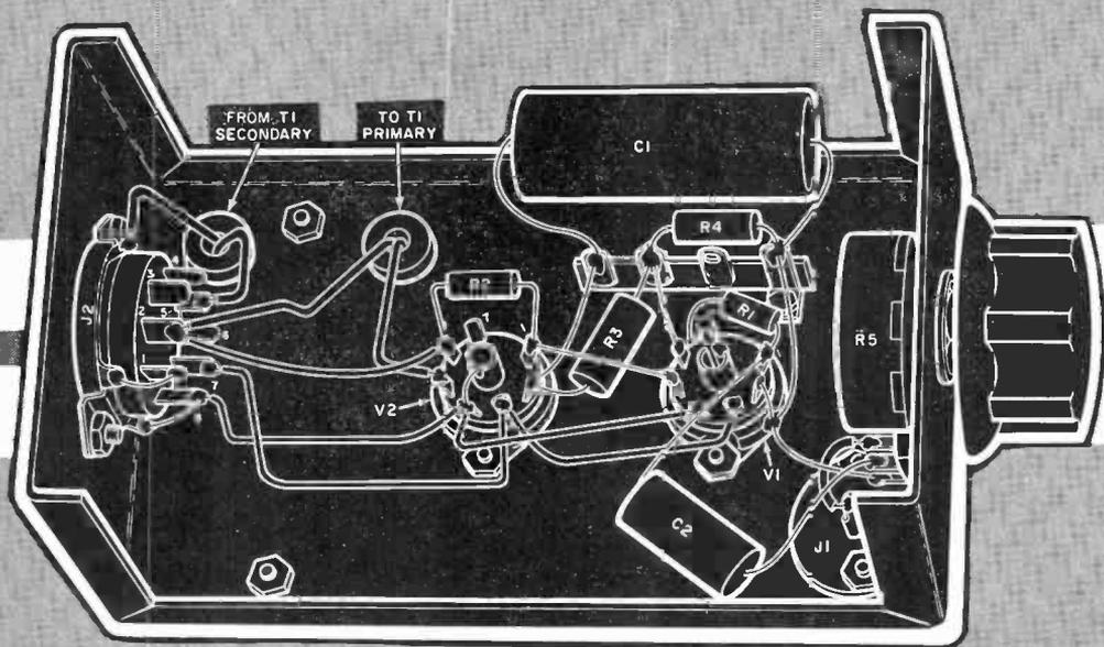
lifier. Almost any of the common tubes can be used if slight changes in circuit values are made; some tubes, of course, will give more gain than others. Two very common types are used here—the 6AU6 pentode (*V1*) and the 6AQ5 beam power audio tube (*V2*).
