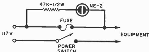
should blow, the current takes the alternate path through the indicator circuit, causing the neon lamp to glow. A 47,000-ohm, 1/2-watt unit, *R1* is a current-limiting resistor and is required for 117-volt operation of the NE-2.
