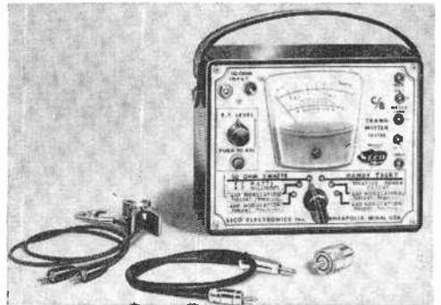
to 5 watts r.f. and has a 0-400-ma. scale. You can check to see how much power you are losing in your transmission line—read the meter and weep!
