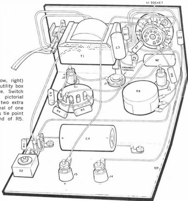
Completed unit (below, right) fits in 3" x 4" x 5" utility box with space to spare. Switch used for S1 (see pictorial diagram, right) has two extra positions. The terminal of one of these was used as tie point for the grounded end of R5.
