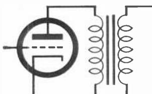
4 The gain of a transformer-coupled audio amplifier stage tends to increase at the low frequencies.
