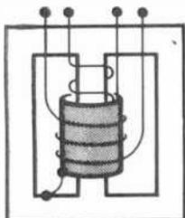
7 A "Faraday screen" is a copper sheet used to reduce inductive coupling between windings.
