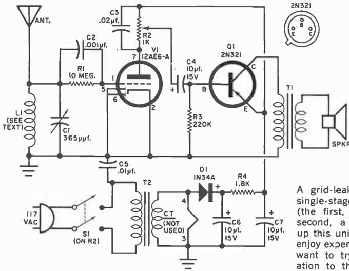
A grid-leak detector and a single-stage audio amplifier (the first, a tube; and the second, a transistor) make up this unique circuit. If you enjoy experimenting, you may want to try adding regeneration to the detector stage.
