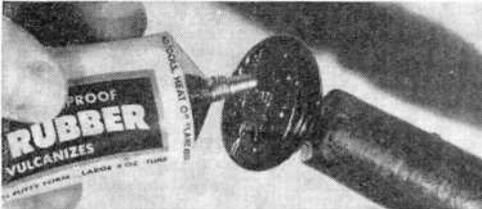
is applied in heavy dabs to the bottom of a portable radio, it will prevent the set from accidentally being pushed off a table. It cushions against shock and vibration, too.
