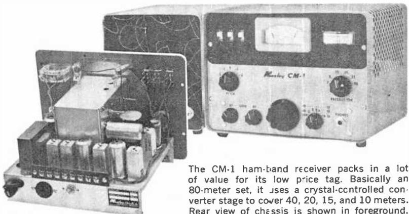
The CM-1 ham-band receiver packs in a lot of value for its low price tag. Basically an 80-meter set, it uses a crystal-controlled converter stage to cover 40, 20, 15, and 10 meters. Rear view of chassis is shown in foreground.
