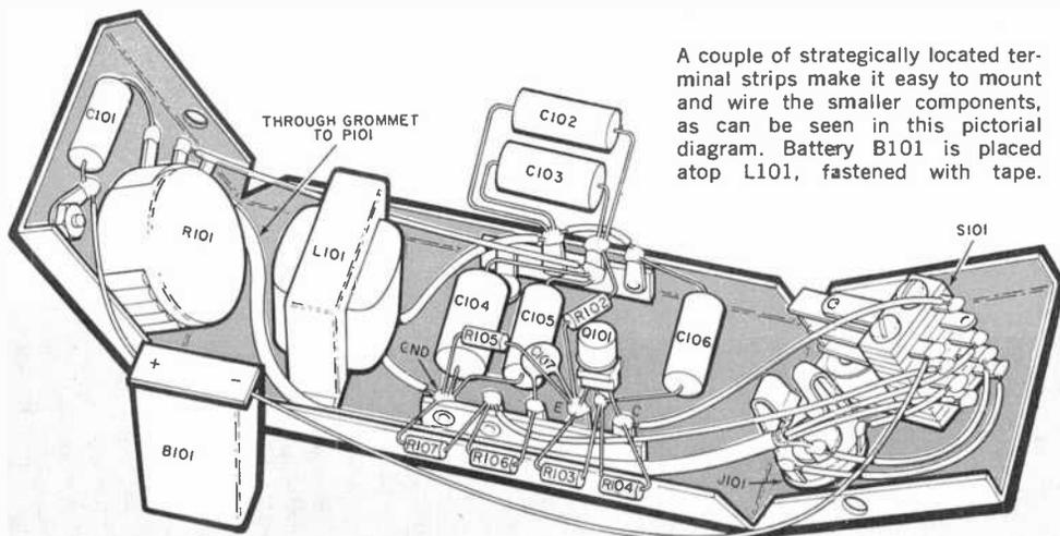
A couple of strategically located terminal strips make it easy to mount and wire the smaller components, as can be seen in this pictorial diagram. Battery B101 is placed atop L101, fastened with tape.
