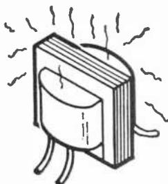
2 If a 50-cps transformer is operated at 60 cps, the transformer will overheat.
