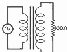
3 A 1:2 primary-to-secondary turns ratio will make 100 ohms across the secondary look like 25 ohms to the primary winding.
