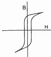
9 Power transformers are made with a laminated iron core material having a narrow hysteresis loop characteristic.
