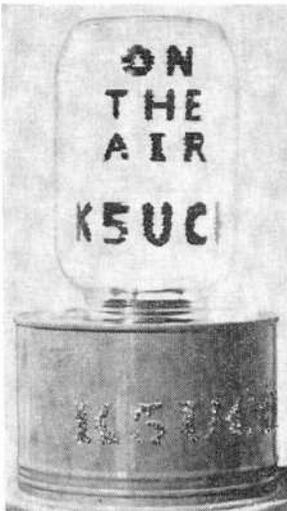
will illuminate the plastic—making the lettering stand out. The bulb can be wired to a manual switch or connected to your transmitter "send-receive" relay.
