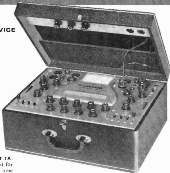
**MUTUAL CONDUCTANCE TUBE TESTER TT-1A:** Deluxe tube testing facilities! Includes adapter in lid for testing new compactron, nuvistor, novar and 10-pin tube types. Indicates Gm to 24,000 microhms. Constant current heater supplies. Ultra-sensitive grid current test. Direct reading ohmmeter leakage test. Built-in calibration circuit & roll chart. Professional quality throughout.
