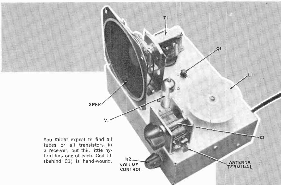
You might expect to find all tubes or all transistors in a receiver, but this little hybrid has one of each. Coil L1 (behind C1) is hand-wound.
