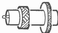
8 The windings of r.f. transformer coils are spiraled back and forth to reduce their distributed capacitance.
