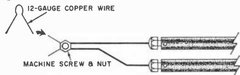
provide a two-point source of heat. Extra "keyholes" can be attached for components having multiple leads, and the prongs can be easily adjusted to any dimension.
