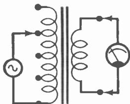
1 "Tapping down" the primary winding of any transformer increases the output voltage of the secondary winding of the transformer.
