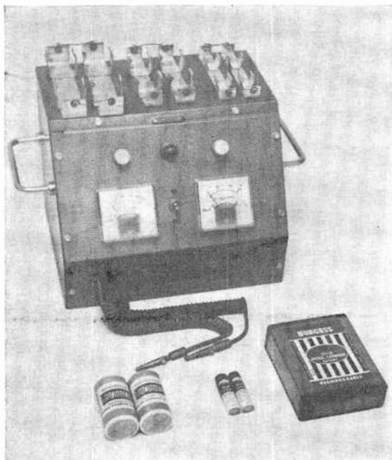
*De luxe heavy-duty charger provides two independent fully adjustable outputs, handles almost every type of nickel-cadmium battery*
