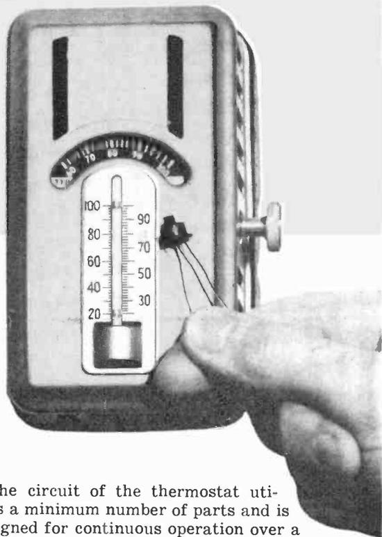
The circuit of the thermostat utilizes a minimum number of parts and is designed for continuous operation over a long period of time. No batteries are required, and the entire unit can be assembled for less than \$10.00—inexpensive indeed for such precise temperature control.
