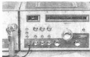
on CW, SSB (upper or lower side bands), FSK, and AM. It delivers 100 watts of r.f. into a 50-ohm load on CW and SSB, 25 watts on AM.
