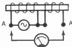
5 With two coils wound in the same direction on a core, as shown above, the voltage across A-A will be the sum of the voltages across each coil.
