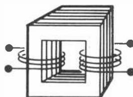
6 Transformer iron cores are laminated in order to reduce the heat generated by induced "eddy currents."
