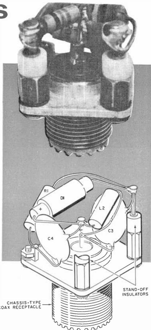
All parts for the sampling unit (see photo and pictorial diagram) are mounted on a coaxial receptacle.
