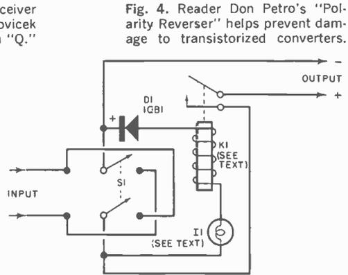
Fig. 4. Reader Don Petro's "Polarity Reverser" helps prevent damage to transistorized converters.
