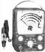
**V-70. VACUUM TUBE VOLTMETER KIT.** Uses stabilized bridge circuit to provide measurements on 7 DC and 12 AC voltage ranges, plus 7 decibel and 7 wide-spread electronic ohmmeter ranges. **Kit: \$31.95; Factory Wired, ready to operate: \$49.95.**
