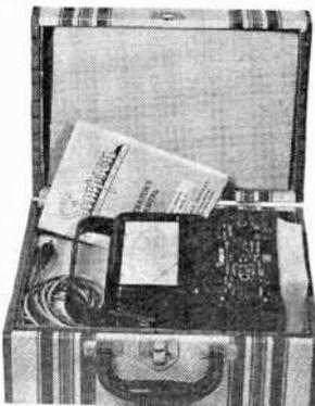
suitcases are available at most "5-and-10's" in a variety of sizes and need only be lined with appropriate padding. Foam rubber or plastic makes an ideal material for this purpose; just cut it to size with a scissors and
