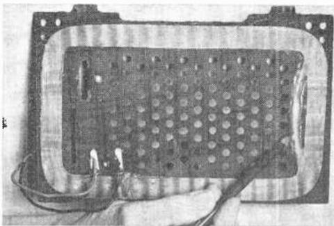
wire. Just melt the wax at one point on the loop and move the turns apart until the stations appear at the proper dial settings.
