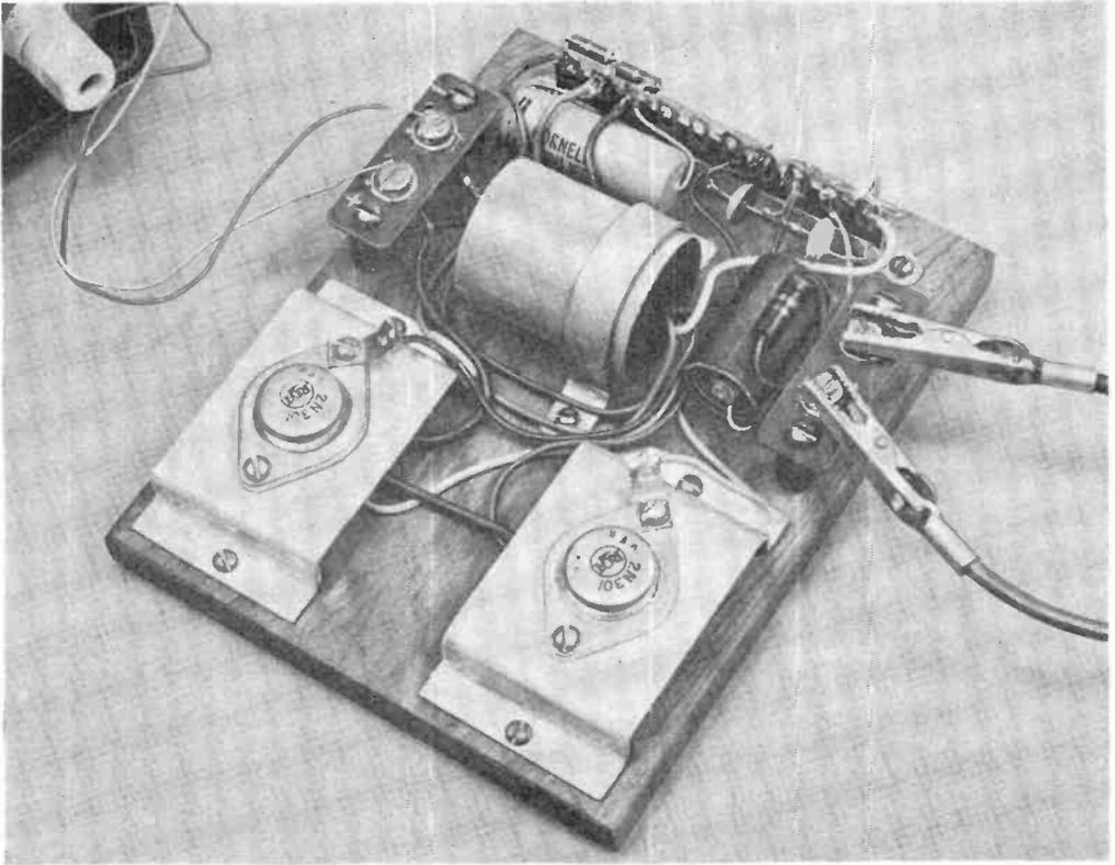
In this case, both the inverter and the filter can be built in a metal box. The leads to the battery should be kept as short as is practical and should be placed well away from antennas and other "inputs."
