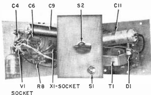
Most of the circuitry in the compactron frequency calibrator is mounted on the two covers of an aluminum utility box. The 6D10 compactron (VI) has been removed from its socket and placed in lower corner of cover shown at far left.
