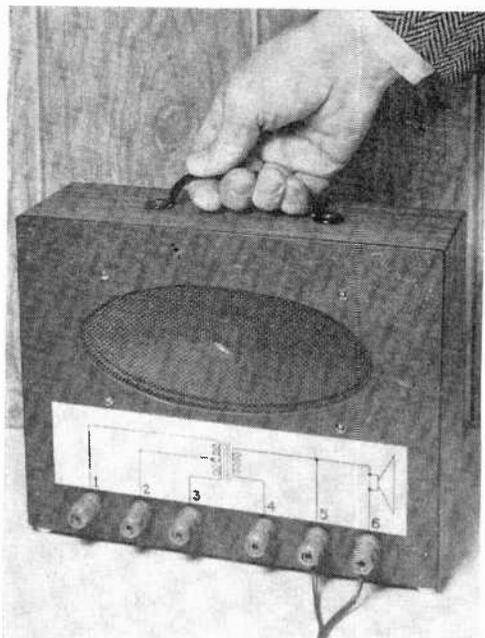
Designed for the serviceman, this Test Bench Squawk Box supplies for chassis under repair the missing audio circuit elements left behind in the customer's house.
