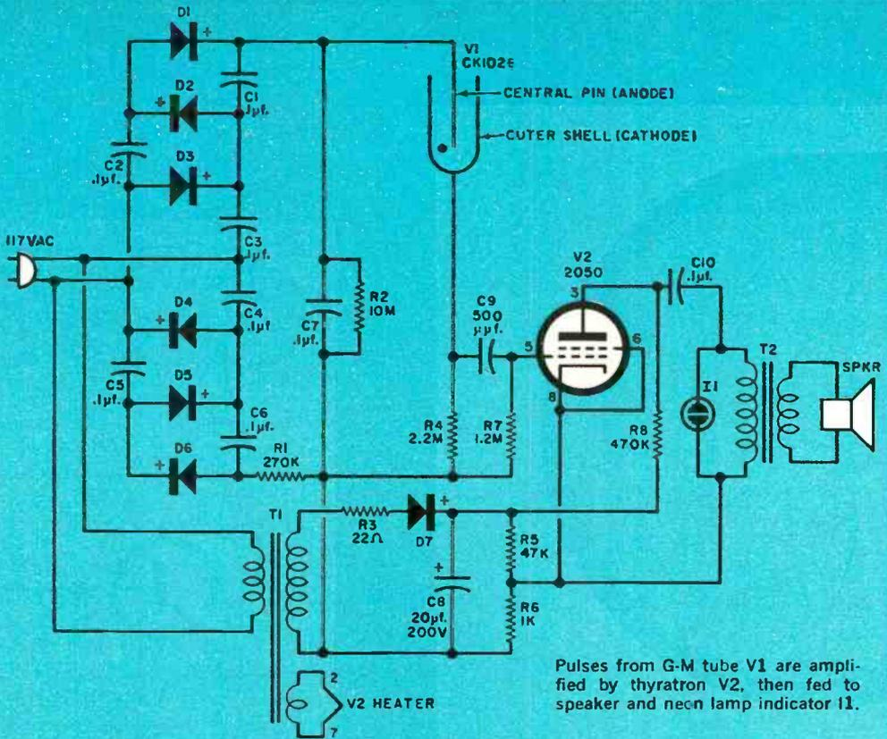
Pulses from G-M tube V1 are amplified by thyatron V2, then fed to speaker and neon lamp indicator I1.
