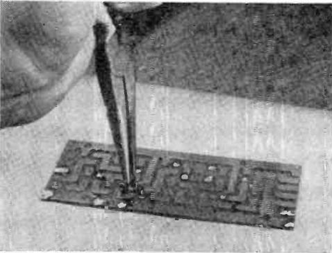
**CRUSHING.** Smash the rest of the resistor with a pair of pliers, and you're left with two bare leads.
