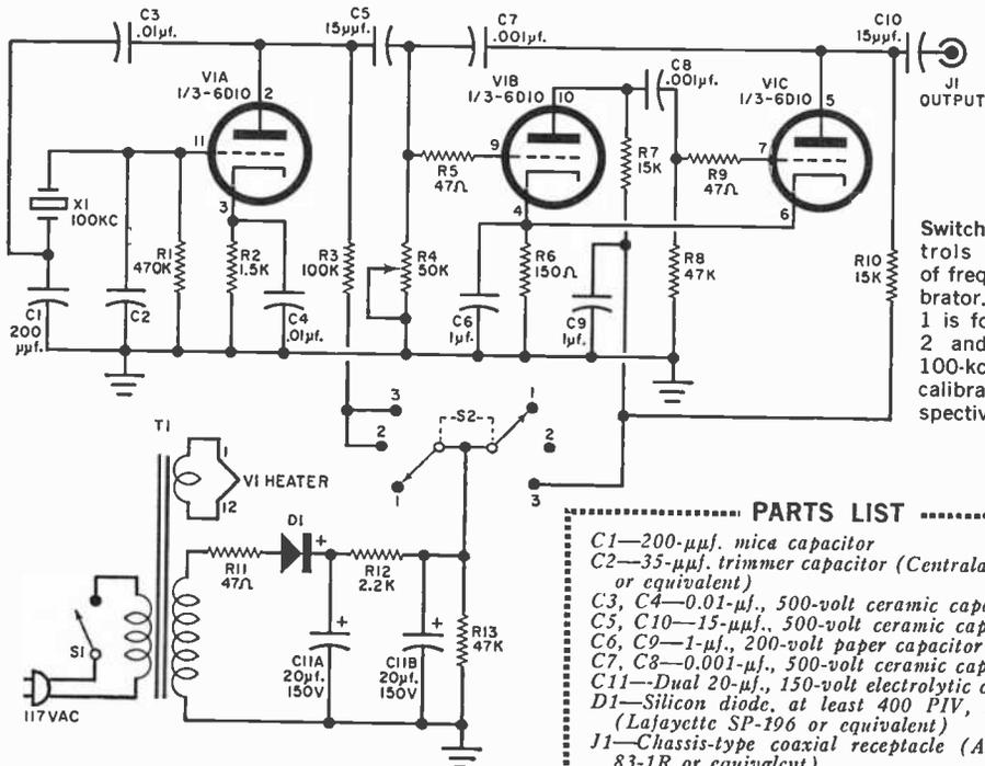
Switch S2 controls operation of frequency calibrator. Position 1 is for standby, 2 and 3 select 100-kc. or 10-kc. calibrations, respectively.
