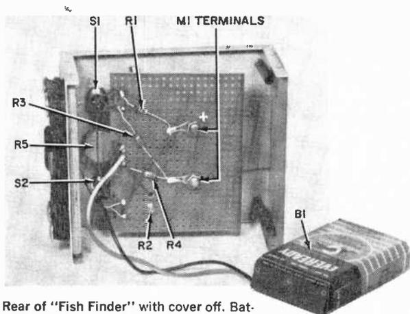
Rear of "Fish Finder" with cover off. Battery *B1* mounts in space behind perforated board.
