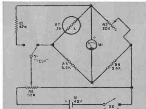
Thermistor ( $RT1$  on schematic) is used as one leg of a Wheatstone bridge indicator.
