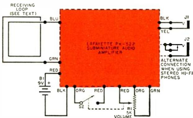
the miniature receiver in his pocket or place it on a table next to his chair. The amplifier or TV set "broadcasts" an audio signal that is inductively coupled to the listener's receiver through a loop antenna placed under the living-room rug. In this way, the listener has complete freedom of movement and trailing wires are eliminated.
