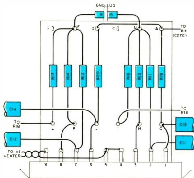
Fig. 6. Mounting turret detail at tube V2.
