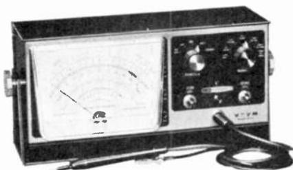
ranges, d.c. and a.c. (r.m.s.), include 0-1.5, 5, 15, 50, 150, 500, and 1500 volts. The unit features seven ohmmeter ranges, and measures up to 1000 megohms with internal battery. The d.c. accuracy is within  $\pm 3\%$  of full scale, a.c. accuracy  $\pm 5\%$  of full scale. Price, \$32.95. (Heath Company, Benton Harbor, Mich.)
