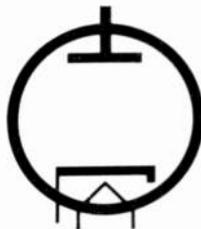
found to suffer from a serious disadvantage when used as a tuned r.f. amplifier. There is a fair amount of electrical capacity between the grid and plate. This permitted a percentage of the signal in the plate circuit to be coupled back to the grid, setting up the basic condition for oscillation.
