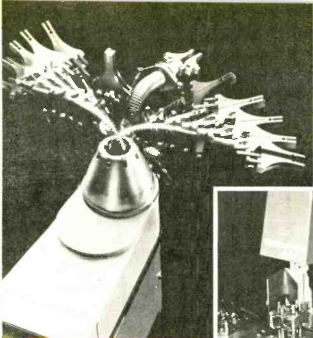
**CLUTCHING HAND** is actually a robot that can grasp 25 lb. or less at any point around it. This device, a "Fleximan" automatic manipulator, can be programmed.
