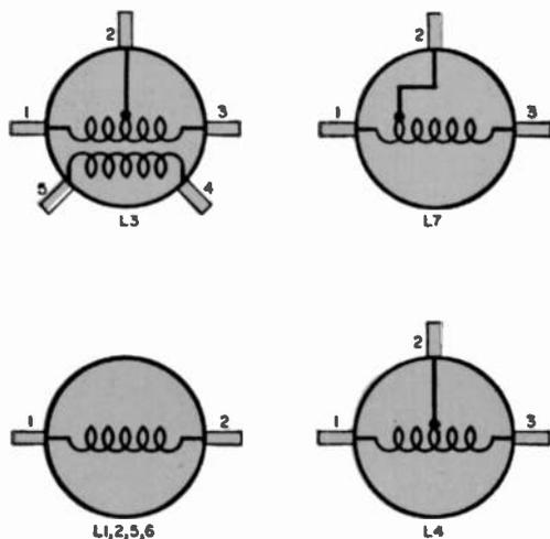
the entire coil in molten paraffin for several seconds. When the wax has dried, remove the Masonite ends and cover the end windings with a coating of cement. Slip on the collar, solder the leads, and cement the collar in place. Give the coil a second dipping in molten wax for about ten seconds, and then push on the mounting clip. This second coating is especially important for L3, since its two windings will be at a 250-volt differential.
