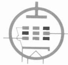
electrons back to the plate without appreciably affecting the normal cathode-to-plate electron flow. Today, the pentode is perhaps the most widely used basic tube type.
