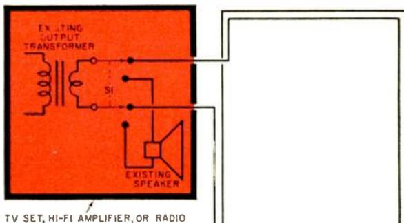
Fig. 2. Schematic diagram of the setup for the wireless earphone receiver. Parts are included in listing at right.
