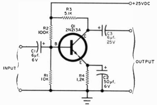
Plug-in module (far left) utilizes a mere handful of components connected to the pins of a defunct miniature tube. Schematic diagram (above) calls for 25 volts of B+, which can be tapped from most power supplies.
