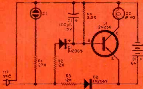
When charged, C1 keeps Q1 from conducting. If power fails, current flows, causing I2 to light.
