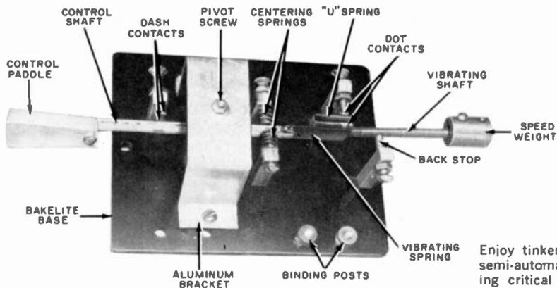
Enjoy tinkering? Try building this semi-automatic key. There's nothing critical about the parts—use what you have on hand. Properly built and adjusted, the key is capable of good c.w. from 10 wpm up.
