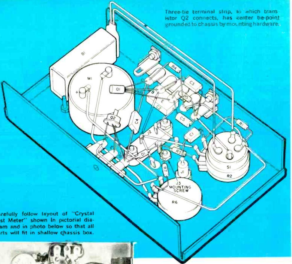
Carefully follow layout of "Crystal Test Meter" shown in pictorial diagram and in photo below so that all parts will fit in shallow chassis box.
