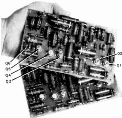
The tetrode transistor output stage provides constant voltage independent of load resistance and signal frequencies. The speaker impedance determines maximum power output. This also means that the user connects his speakers to the four speaker terminals and forgets tube-style matching problems.
