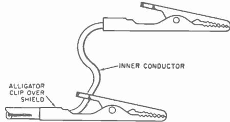
be applied where the two tabs meet. Attach the clip to the center conductor as you normally would.
