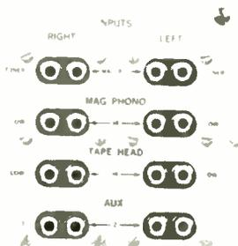
Input jacks are on the rear panel (photo at left); two tape out jacks at the front panel's right edge (far left) are paralleled with two others on the back panel. Large jack in lower right corner of panel is for stereo headset.
