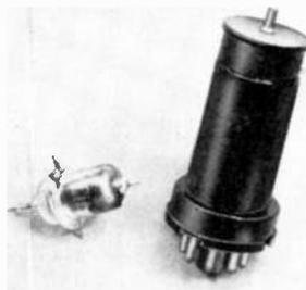
Gone but not forgotten are these three pioneers. The 200A (left) was one of the first mass-produced tubes. A 954 Acorn helped introduce VHF to communication services. At right is an 1851, a super-high-gain tube developed just before World War II.
