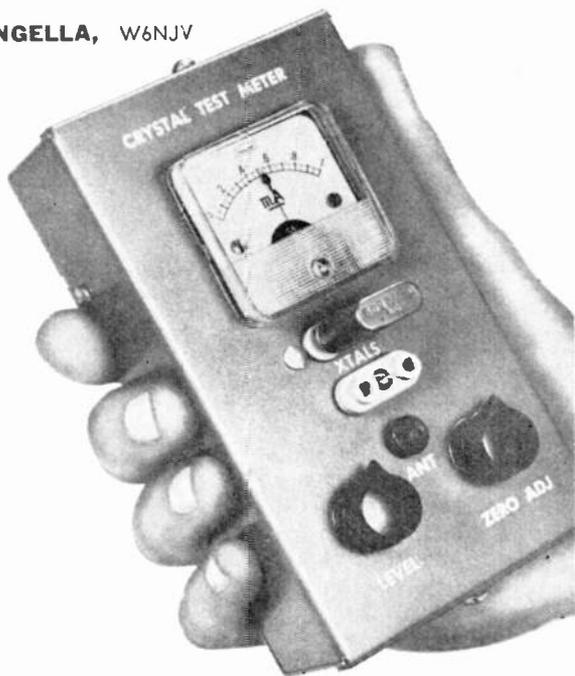
detected by diode *D1* and amplified by transistor *Q2*. Meter *M1*, in *Q2*'s collector circuit, then shows a reading which indicates the relative activity of the crystal.
