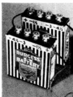
screw-type terminals eliminate the need for battery holders or soldering. The batteries (Burgess 5360 or equivalent) measure about 2 1/2" x 2 1/2" x 2 1/2" and are readily available—at a cost of about 88 cents each—from most electronic supply houses. There are three voltages per battery—1.5, 3, and 4.5 volts—and with two batteries, additional voltages of 6, 7.5, and 9 volts are possible.
