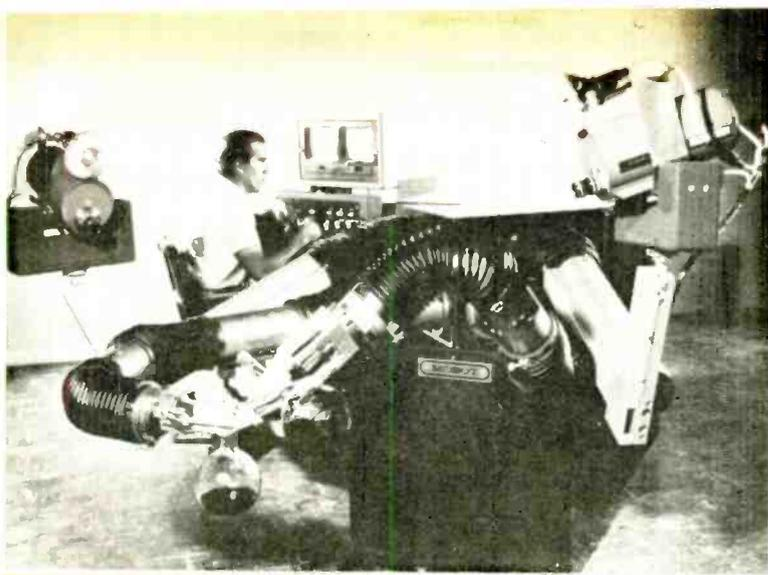
**MOBOT MIXER** pours chemicals from one flask to another under command of operator at control console. A vehicle which can move by remote control, the "Mobot" has a delicate touch, handles dangerous jobs at a distance from the operator.
