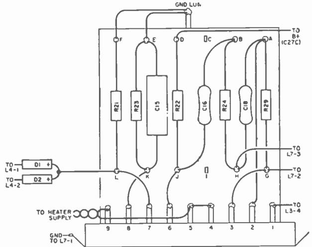
Fig. 8. Mounting turret detail at tube V3.
