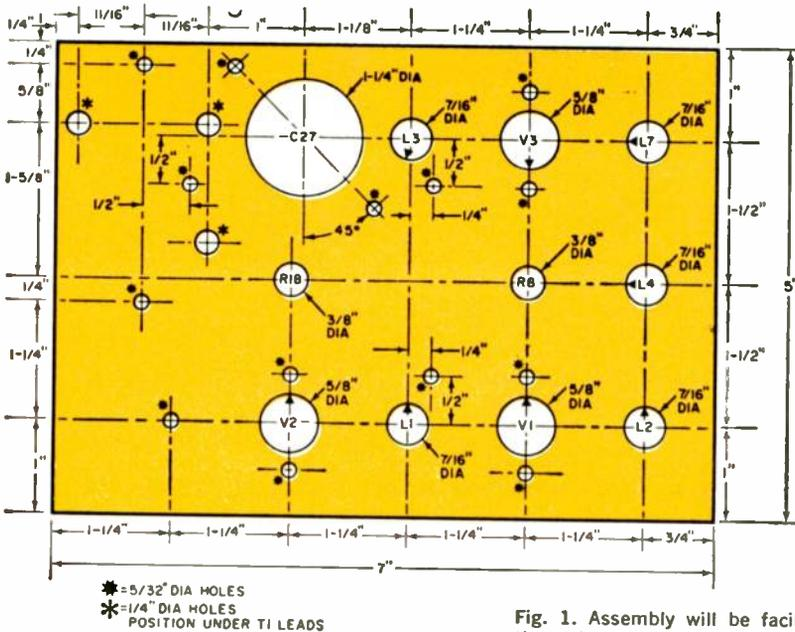
Fig. 1. Assembly will be facilitated by duplicating the author's chassis dimensions. The two end panels are shown at top of page and a top view of the chassis is directly above. Note the small orientation diamonds in the chassis top view. These are important since they position the coils and sockets.
