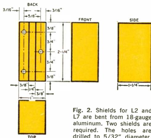
Fig. 2. Shields for L2 and L7 are bent from 18-gauge aluminum. Two shields are required. The holes are drilled to  $\frac{5}{32}$ " diameter.
