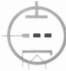
Thus, early r.f. amplifiers tended to be quite unstable, and a variety of schemes were developed to neutralize the effects of grid/plate capacitance. In general, these consisted of introducing enough inverse (or negative) feedback from the plate tuned circuit into the grid circuit to counteract the direct feedback inside the tube and prevent unwanted oscillation.
