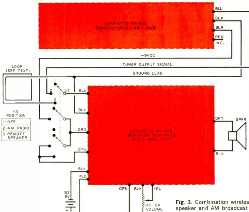
Fig. 3. Combination wireless remote speaker and AM broadcast receiver.
