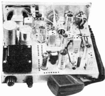
The wide-open interior of the C-22 is obvious from these photos. Note that the power supply is in a shielded section. The power supply in the higher priced (\$69.95) unit, incidentally, operates from both 117 volts, a.c., and 12 volts, d.c. Crystal access is provided by a "door" in the bottom plate of the chassis wrap-around.
