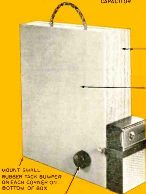
LOOP ANTENNA IS 20 TURNS OF #26 ENAMELLED
