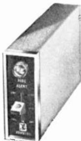
Selective calling system; may be attached to most CB transceivers; self-contained power supply; each unit is both tone generator and monitor with resonant-reed relay; indicator call light stays on after proper incoming tone signal is received; 37 possible tones available; either 117- and 12-volt, or 117- and 6-volt models.
