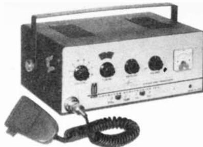
receiver; universal power supply (117- and 12-volt); 9-tube performance double-conversion superhet (1 r.f. stage, 1650-kc. conversion, 455-kc. conversion and i.f. stage); crystal-controlled second oscillator; gated-audio noise-limiting squelch system; S-meter; ceramic mike; pi-network output; no relays—electronic switching; 12 3/16 x 5 1/8 x 9 7/16; 13 lb.
