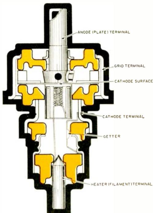
High transconductance, close element spacing, and very low lead inductance are the design factors responsible for the good performance of the light-house tube at frequencies up to 3000 mc.
