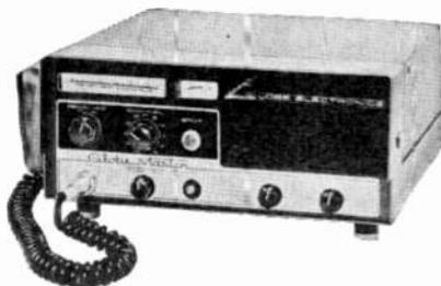
11-channel, crystal-controlled transmit and receive plus tunable receiver; "spotting" switch; universal power supply (either 117- and 12-volt, or 117- and 6-volt available at the same price); 14-tube performance double-conversion superhet; series noise limiter; adjustable squelch; ceramic mike; speech clipping and filtering for effective modulation; pi-network output; S-meter; 11½ x 4½ x 10; 16 lb.
