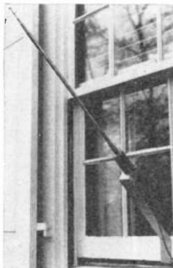
The antenna operates on six different bands—2, 6, 11, 10, 15, and 20 meters—by virtue of a shorting bar for 2 and 6 meters, and small interchangeable coils for the other bands. Rated at 175 watts PEP and 100 watts for AM, the antenna extends to 60 inches. Included in the package are 10 feet of RG-58A/U transmission line,
