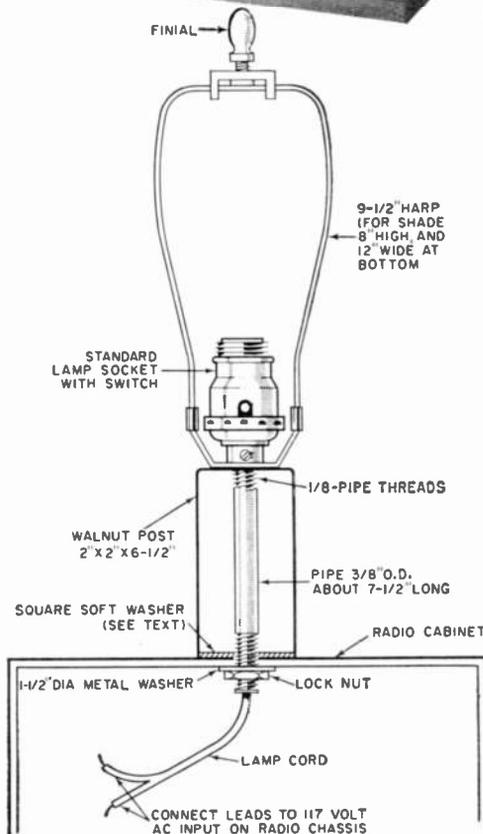
and already threaded—is available from practically any electrical supply house, and at a very reasonable price.) Then I cut a square of "Non-Skid" (an "under-the-rug" rubbery material) for use as a "washer" between the bottom of the post and the top of the plastic radio cabinet.
