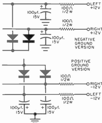
engine is running. A remedy is to add two RC filters to the device to filter out such "hash" as shown in the diagram.
