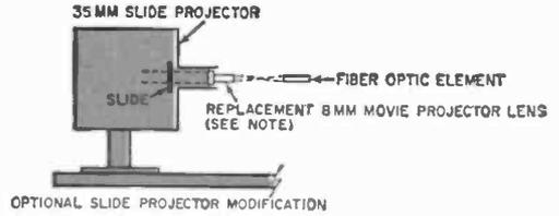
Fig. 2. Two methods can be used to modify a slide projector for the experiment. Use a mailing tube as in Fig. 1 below, or mount a replacement 8-mm. lens in the slide projector barrel as shown above.
