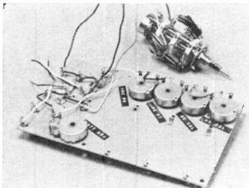
In wiring kit, the transistor mounting board comes first, then the Range and Battery Off switches.
