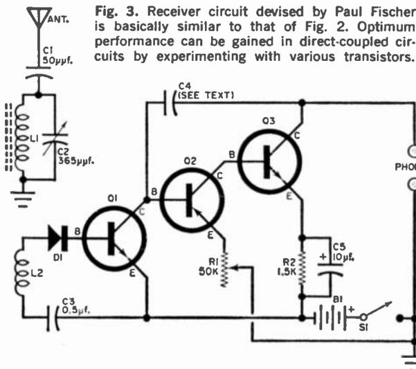
Fig. 3. Receiver circuit devised by Paul Fischer is basically similar to that of Fig. 2. Optimum performance can be gained in direct-coupled circuits by experimenting with various transistors.
