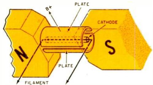
For efficient magnetron operation, a definite relationship between plate voltage and magnetic field strength in the interaction space must always be maintained.
