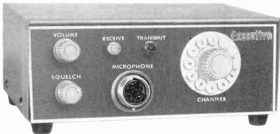
A brand new compact control unit that permits the installation of transceivers in the automobile trunk or other out-of-the-way space. Unit mounts under auto dashboard and gives you complete remote control of transceiver.
