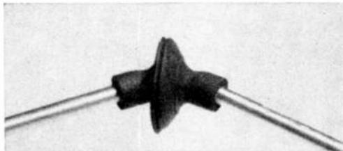
the two suction cups tightly together. Even shafts that are badly misaligned can be coupled with these quick universal joints.
