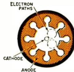
The multi-cavity magnetron has advantages that are important in practical radar applications.
