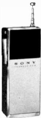
completely free, since the set is keyed with a fingertip cable release. The chassis is out of the way, too, suspended in a shoulder case and belted around the waist. Battery operated and with a range of up to 6 miles, the CB-106 includes chassis, headset-microphone, microphone cable release, shoulder case, batteries.
