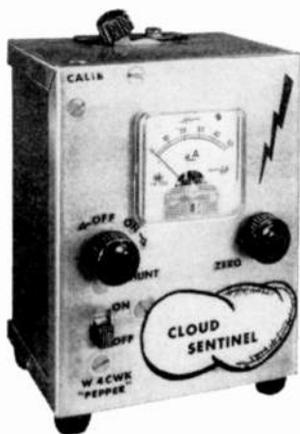
Completed Cloud Sentinel is shown above, the parts layout at the right. Parts values and arrangement are not at all critical; principal requirement is sensitive meter. At far right is a photo of antenna used by the author (see text). Use #14 bare copper wire for spikes, insulated wire for the lead-in taped to mast.
