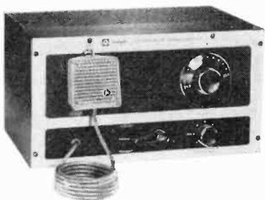
The evolution of CB transceivers is shown by two Knight-Kits (Allied Radio) introduced in 1960 and 1963. Top: the newest kit has double-conversion receiver, multiple channels, maximum utility power supply. Bottom: the older kit, with poor selectivity receiver and only one crystal-controlled channel.
