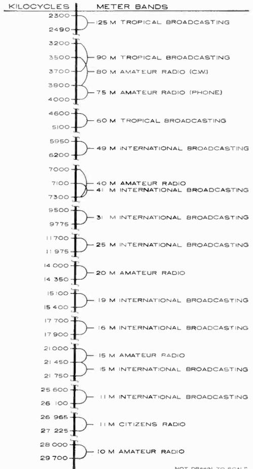
Frequency and wavelength subdivisions in the short-wave bands. On the right-hand side of the vertical bar in each case is the "colloquial" name used in referring to a particular band. On the left-hand side are the upper and lower frequency limitations for each band, which have been set either by international treaty or through accepted usage. These subdivisions apply mainly to frequency allocations and assignments in North and South America.
