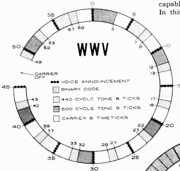
Twenty-four hours a day, radio station WWV, located outside of Washington, D.C., transmits signals on 2.5, 5.0, 10.0, 15.0, 20.0, and 25.0 mc. The accuracy of any of these radiated frequencies is within one part in 10 billion! The wheel at left shows what happens during one hour of transmitting time. Note that different tones are alternated and that the carrier goes off the air after the voice announcement just before 45 minutes past the hour.
