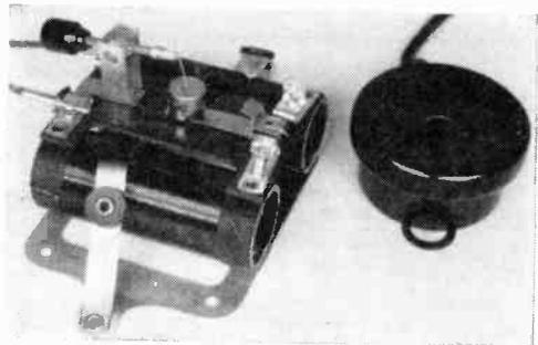
For low-cost operation, you can’t beat the galena crystal set of the 1920’s. This popular version with two sliders on the tuning coils could receive AM broadcasting stations 10 miles away—if it was connected to a long-wire antenna and a “water-pipe” ground. The single earphone is a low-resistance type that was widely used by telephone companies.
