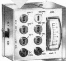
Measures DC voltages from 0 to 500 volts, AC voltages from 0 to 250 volts, DC milliamperes from 0 to 100 milliamperes. Accuracy within  $\pm 10$  percent. Dimensions: 3" x 3" x 2"
