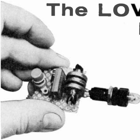
EVER have a problem providing a pilot light for a new transistorized battery-operated gizmo? The first solution that comes to mind is the old standby, a #47 pilot lamp. However, when you realize that a #47 draws 900 mw., the unit shown here, with a drain of only 30 mw., begins to "shine" by comparison.
