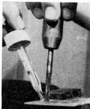
The carbon tet can be stored in an old medicine dropper bottle which will also serve as a convenient dispenser. However, make sure that the room is well-ventilated while you're using the carbon tet. —Robert K. Dye
