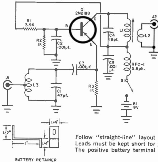
Follow "straight-line" layout shown here. Leads must be kept short for good results. The positive battery terminal is grounded.
