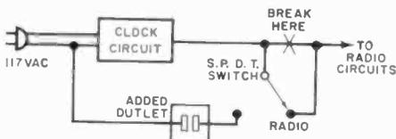
to the diagram. The s.p.d.t. switch can be mounted near the outlet. Locate the wire from the clock switch to the radio circuits and wire the added components as shown.
