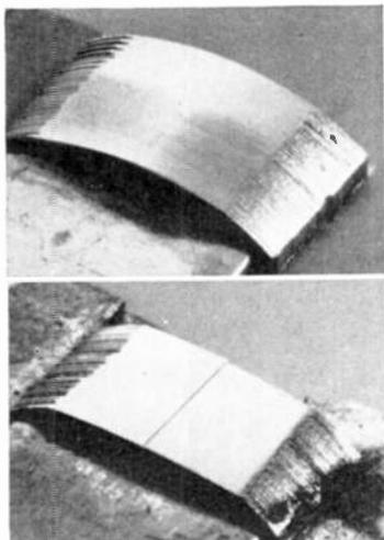
The entire story becomes dramatically clear when we compare heavily worn head (lower) with new one. Note how abrasive tapes have worn down the head, widened recording gap. Uneven wear characteristics are caused by improperly slit tape. Note, too, the accumulation of oxide in the gap and around the head. This head is useless!
