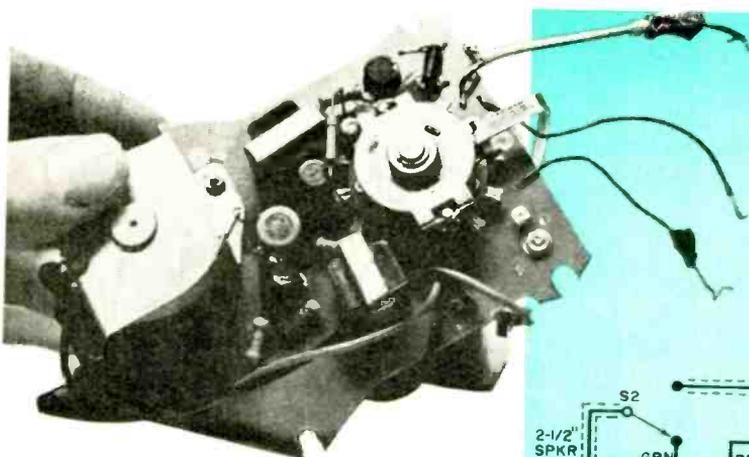
The Min-Corder comes assembled and ready to put into the cabinet. It uses a continuous loop of tape with oxide on both sides.
