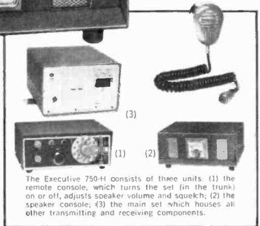
The Executive 750-H consists of three units: (1) the remote console, which turns the set (in the trunk) on or off, adjusts speaker volume and squelch; (2) the speaker console; (3) the main set which houses all other transmitting and receiving components.
