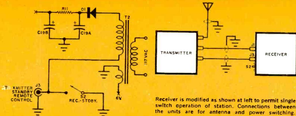
Receiver is modified as shown at left to permit single switch operation of station. Connections between the units are for antenna and power switching.
