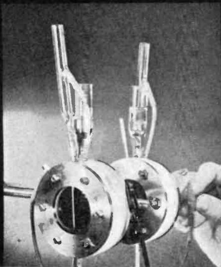
This experimental high-temperature fuel cell uses a solid zirconia electrolyte (white cylinder). The dark cylinder is a graphite electrode. Cell uses natural gas and oxygen to generate electricity.
