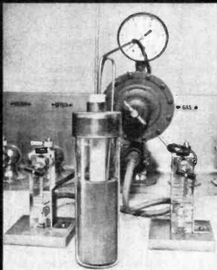
Below is a cutaway mock-up of one of the fuel cell canisters installed in Gemini. Fuel cell modules — the first may be in orbit when you read this — produce drinking water for astronauts as well as up to two kilowatts of electrical power.
