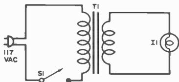
Simple circuit above is easily wired. Solder all connections and use tape or wire nuts over *T1*'s wires to insulate them.
