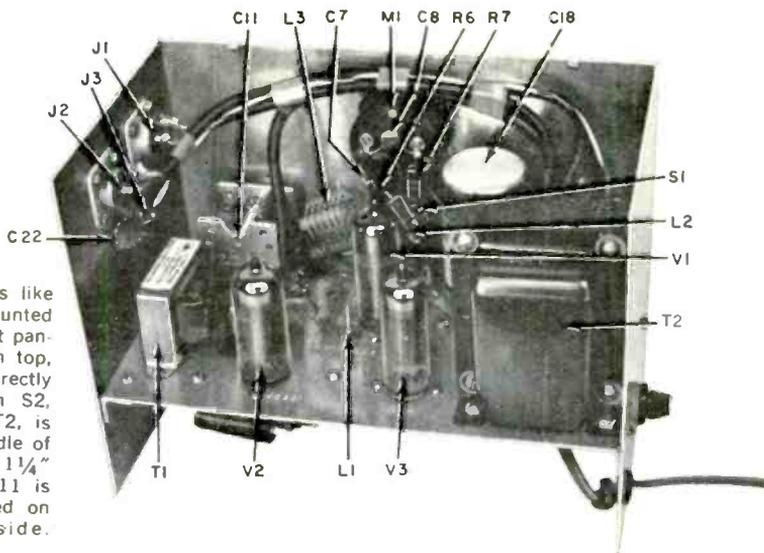
Top of rig looks like this, with M1 mounted at center of front panel and  $\frac{1}{2}$ " from top, S1 and C10 directly below it. Switch S2, hidden behind T2, is mounted in middle of panel and about  $1\frac{1}{4}$ " in from side; C11 is similarly mounted on the opposite side.
