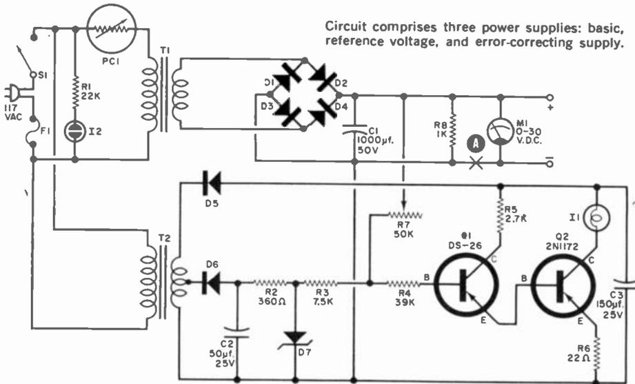
Circuit comprises three power supplies: basic, reference voltage, and error-correcting supply.
