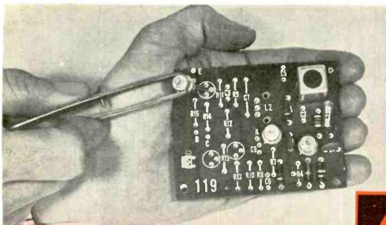
The printed circuit board needs to have the holes drilled in it for parts mounting. Reverse side is silk-screened for identification. Use care in mounting the transistors to avoid heat damage.
