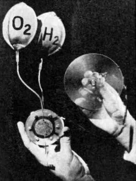
A hydrogen-oxygen fuel cell, circa 1959 shows immense progress that has been made in a few years. Object at right is a G.E. cell is a rotor with a propeller.
