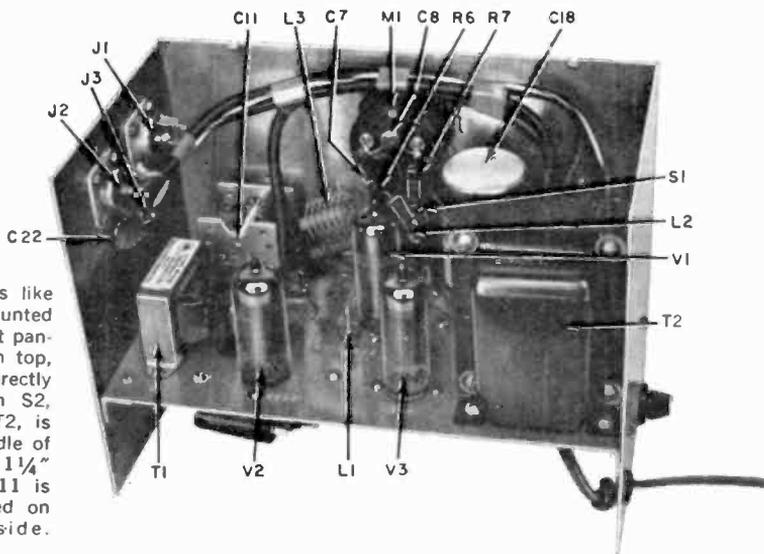
Top of rig looks like this, with M1 mounted at center of front panel and 1/2" from top, S1 and C10 directly below it. Switch S2, hidden behind T2, is mounted in middle of panel and about 1 1/4" in from side; C11 is similarly mounted on the opposite side.
