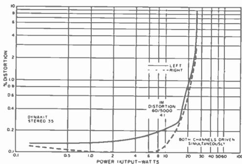
Intermodulation distortion as measured by the Hirsch-Houck Laboratories was below 0.5% for all output levels up to 17.1B watts output per channel.
