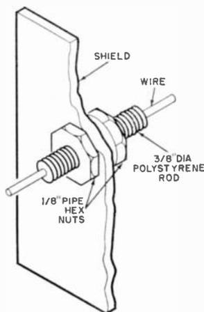
mount the bushing with a nut on each side of the shield, and simply thread your wire through it. That's all there is to it.
