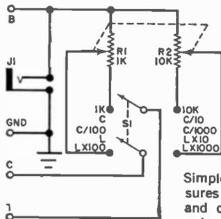
Simple instrument measures values of coils and capacitors. Adjust pots to match voltage across unknown parts.
