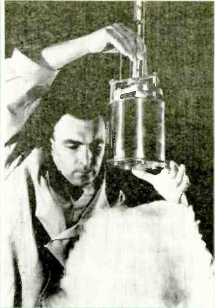
This device, the world's most powerful superconductive magnet at 107,000 gauss, is lowered into vapor-shrouded bottle of liquid helium. Despite the intense field it generates, it requires only an initial starting current.
