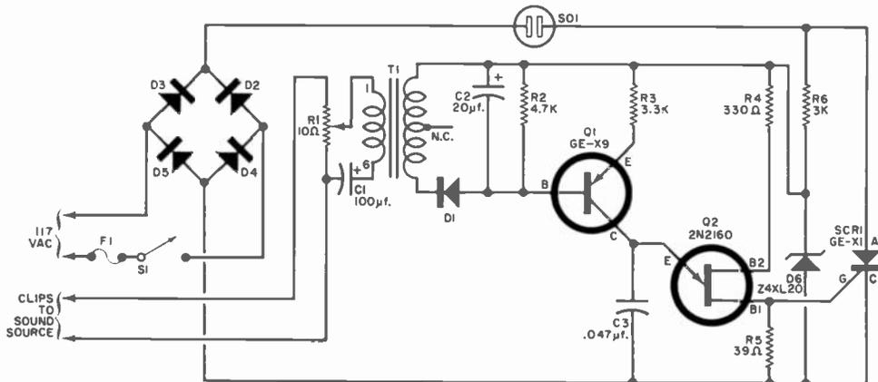
Rhythmicon consists of bridge rectifier, audio pulsing circuit (Q1-Q2), and power control (SCR1)
