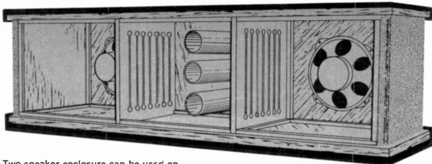
Two-speaker enclosure can be used on its side as above, or on end as seen below. Novel filters (the slotted boards) and ports furnish bass boost.
