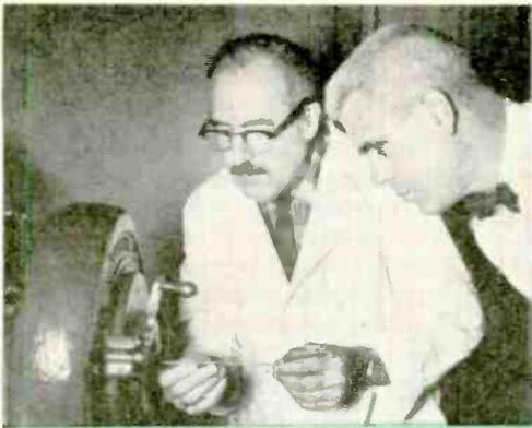
Many superconductive materials, as niobium-tin, can't be bent or shaped—they're just too brittle. Bell Labs solved the problem by enclosing the raw ingredients in a pure niobium tube, drawing tube into a thin wire (see above) and shaping it into a coil, and then putting it into a 1,000° C furnace to fire it.
