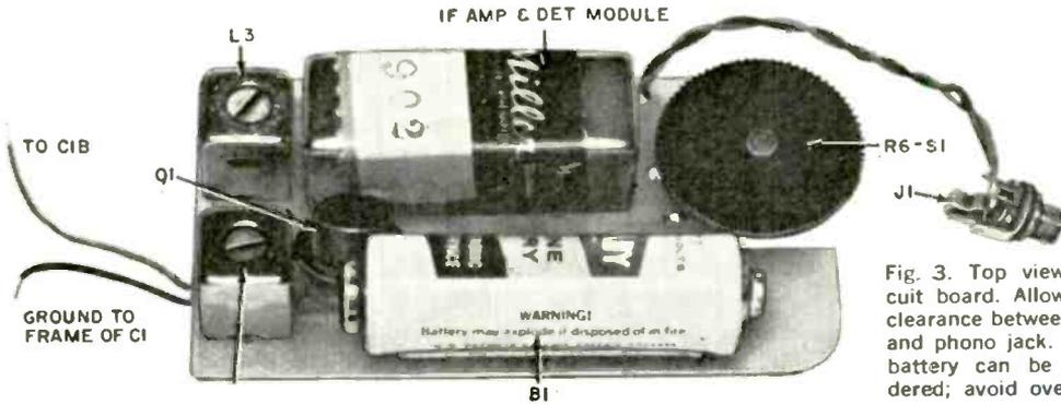
Fig. 3. Top view of circuit board. Allow enough clearance between battery and phono jack. Leads to battery can be spot-soldered; avoid overheating.
