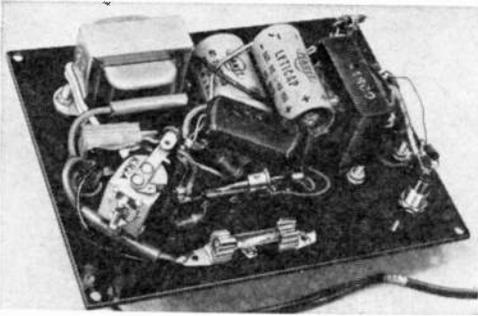
Spring tension on normally-closed relay should provide good contact. Tighten to increase "on" time.
