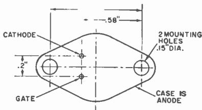
Bottom view of the RCA 2N3228 rectifier. In this speed control circuit, the rectifier is bolted to the heat sink and insulated from the metal box.
