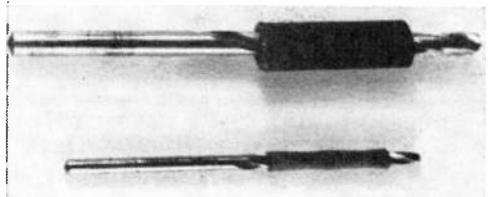
force-fit a small length of spaghetti over the drill bit—the tighter the better—exposing as much of the bit as is needed. Several layers of tape wrapped around the bit at the proper place can serve the same purpose.
