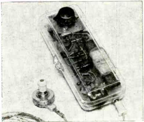
ume of air as a loudspeaker does. Ear-phone impedance should be anywhere from 3000 to 7000 ohms. Do not use a low-impedance phone, as it will load down the output circuit excessively.
