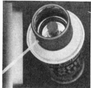
neatly trim out the top of the plastic cover with a small knife. Then drill or punch a hole on the side of the cap for the spray extender tube. When the can is empty, the modified cap can be transferred to a new can.
