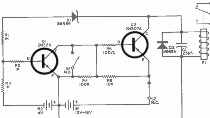
Fig 1. Reader Ronald L. Ives employs transistors to latch relays and other control devices. Circuit stays off until triggered by momentarily closing switch S1. Circuit stays on until switch S2 is temporarily opened or until the power is removed.
