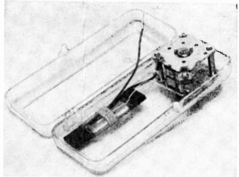
Except for the antenna loopstick, variable capacitor and phono jack, all components including the i.f. module are mounted on a small board, measuring just  $2\frac{7}{8}$ " x  $1\frac{1}{16}$ ", as shown in Fig. 2. This is not a printed circuit. All the components are hand-wired.
