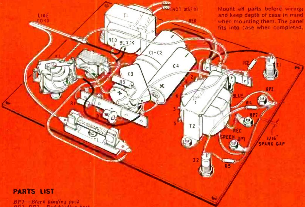
Mount all parts before wiring and keep depth of case in mind when mounting them. The panel fits into case when completed.
