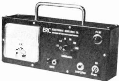
100 kc., and  $\pm 2\%$  from 100 to 200 kc. Input impedance is 100,000 ohms. An output jack, designed for use either with an oscilloscope or earphones, provides a 15-volt, peak-to-peak square wave into a 50,000-ohm load. Price, \$149.50.
