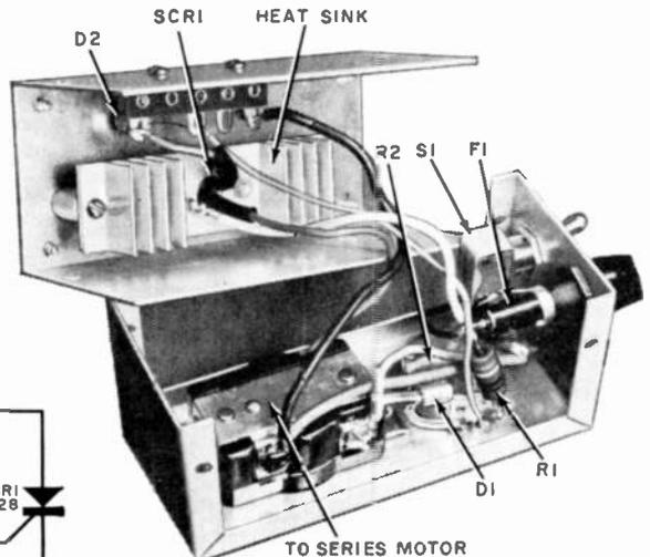
The heat sink in the speed control must be insulated from the aluminum box; use H. H. Smith Type 2645 ceramic insulators. Position sink so that it will not short out to the metal back of the outlet.
