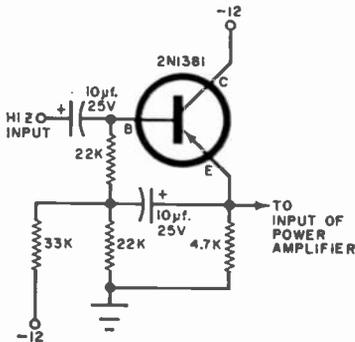
feed the amplifier from a high impedance source. Incidentally, I feel that the regulated d.c. supply is a luxury—any low-impedance 12-volt power supply with a current capacity of 1 to 2 amps will suffice to power the amplifier.
