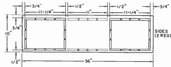
Construction of enclosure is detailed at left. All panels can be made from  $\frac{1}{2}$ " plywood, with  $\frac{1}{2}$ "-square stock making up the cleats. Cut all pieces exactly to size; place cleats as shown for easy assembly.
