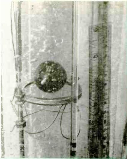
Although lead ball appears to be floating, it is actually riding on a cushion of magnetic force set up by the loop of wire below it in liquid helium. This opposition to any magnetic field is known as diamagnetism.
