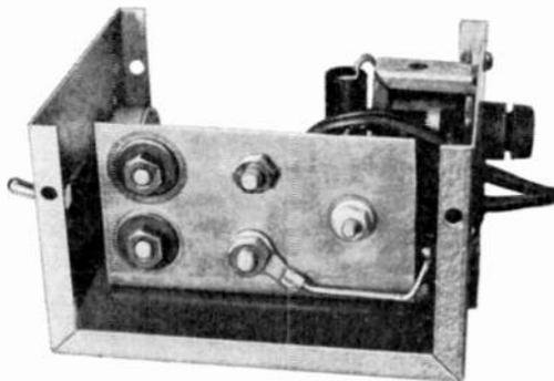
and the positive terminal of C1 to the transformer terminals that give the highest impedance—with the unit used by the author, terminals 1 and 6. Connect the push-pull plate side as shown in the schematic; the center tap is not used and can be shorted.
