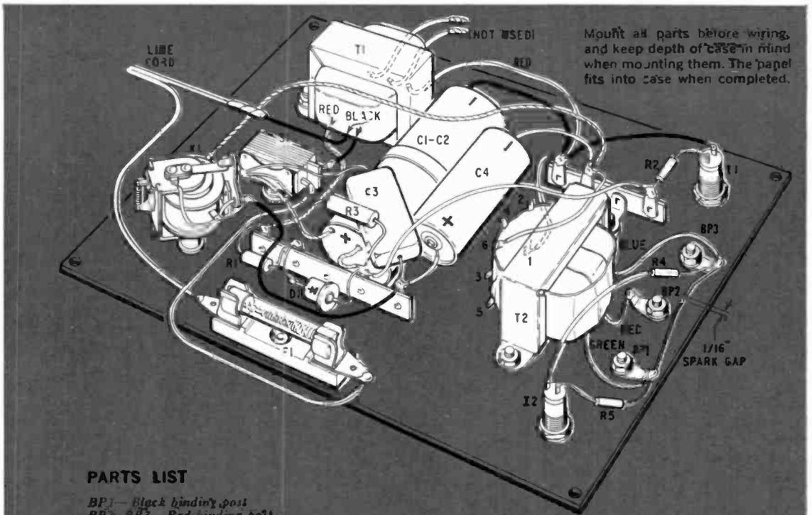
Mount all parts before wiring, and keep depth of case in mind when mounting them. The panel fits into case when completed.
