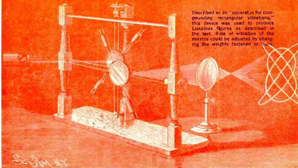
Described as an "apparatus for compounding rectangular vibrations," this device was used to produce Lissajous figures as described in the text. Rate of vibration of the mirrors could be adjusted by changing the weights fastened to them.
