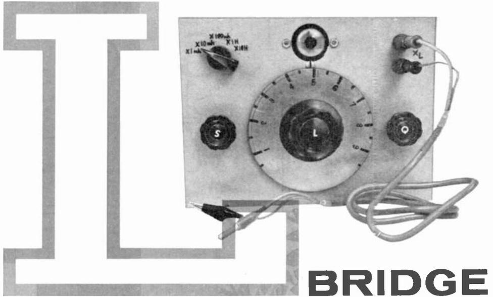
***Build this multi-range inductance tester to find unknown values of r.f. i.f., audio and filter coils and chokes***
