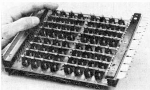
Electromagnetically operated reed switches replace conventional relays in the "No. 1 Electronic Switching System." These switches respond to commands from the central control and connect telephone subscribers to trunk lines.
