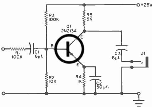
Harold Reed's impedance-matcher enables use of low-impedance headphones in high-impedance audio circuits without excessive loading. A potentiometer in place of *R5* could serve as a volume control.
