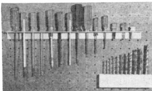
by hacksawing two slots about  $\frac{1}{4}$ " apart approximately 2" in from each end and bend to shape. These newly formed hooks should be spaced to line up with the peg-board holes. For an easy fit, use a file or grindstone to round off the edges and reduce the diameter of the hooks if necessary. A scrap block of wood can also be utilized as a tool holder, as shown in the photo.
