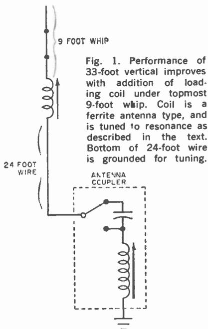
Fig. 1. Performance of 33-foot vertical improves with addition of loading coil under topmost 9-foot whip. Coil is a ferrite antenna type, and is tuned to resonance as described in the text. Bottom of 24-foot wire is grounded for tuning.
