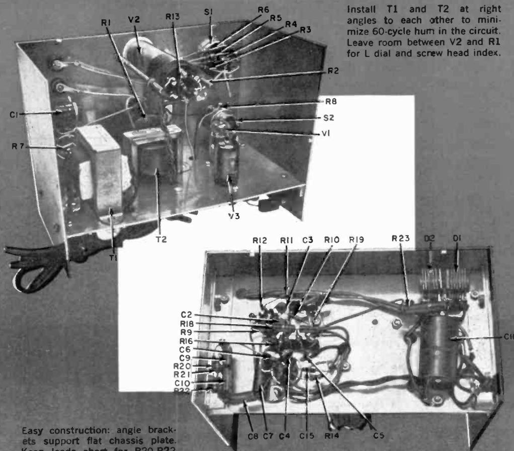
Easy construction: angle brackets support flat chassis plate. Keep leads short for R20-R22 and C8-C10, in the oscillator circuit. Other wiring is not critical.
