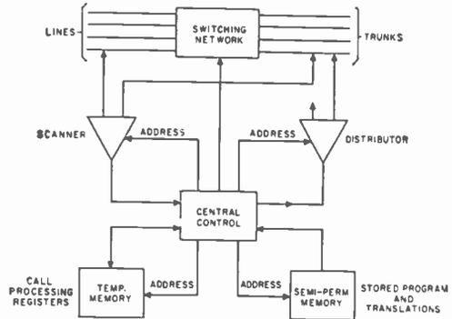
Deceptively simple block diagram outlines the basic plan of the No. 1 ESS. Lines go to phone subscribers and trunks connect to other exchanges. Central control tells ("address") the scanner and distributor how rapidly to monitor incoming and outgoing calls. Description of the memory banks appears in text.
