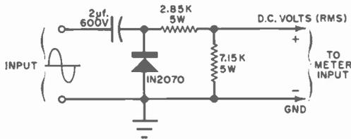
Fig. 4. Divider in demodulator probe delivers about 70% of peak voltage to meter circuit to enable direct readout of r.m.s. voltages.
