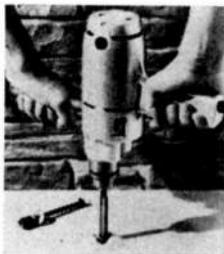
ping one switch turns off the universal motor, while flipping the second switch reverses the drill. The "All Drill" can also be used with almost any attachment. Price, \$44.95.
