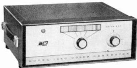
and to align the color demodulators. Suitable for operation on channels 3, 4 or 5, it connects directly to the TV antenna terminals. Its r.f. output is more than 5000  $\mu\text{V}$ . The unit is power-transformer-operated and line-isolated to prevent shock hazards. Price, \$134.95.
