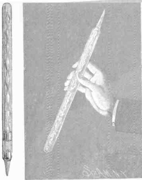
The self-exciting Geissler tube used static electricity to produce momentary flashes of light. One version of the device, which was evacuated and partially filled with mercury, found application as a sea-going marker buoy.
