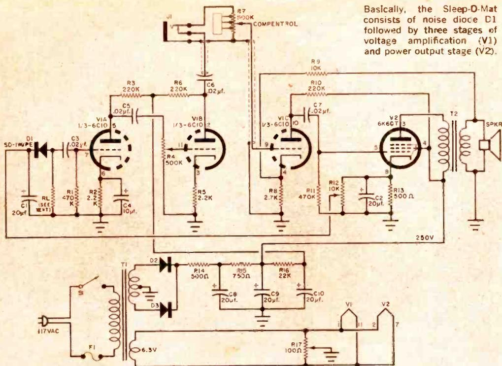
Basically, the Sleep-O-Mat consists of noise diode D1 followed by three stages of voltage amplification (V1) and power output stage (V2).
