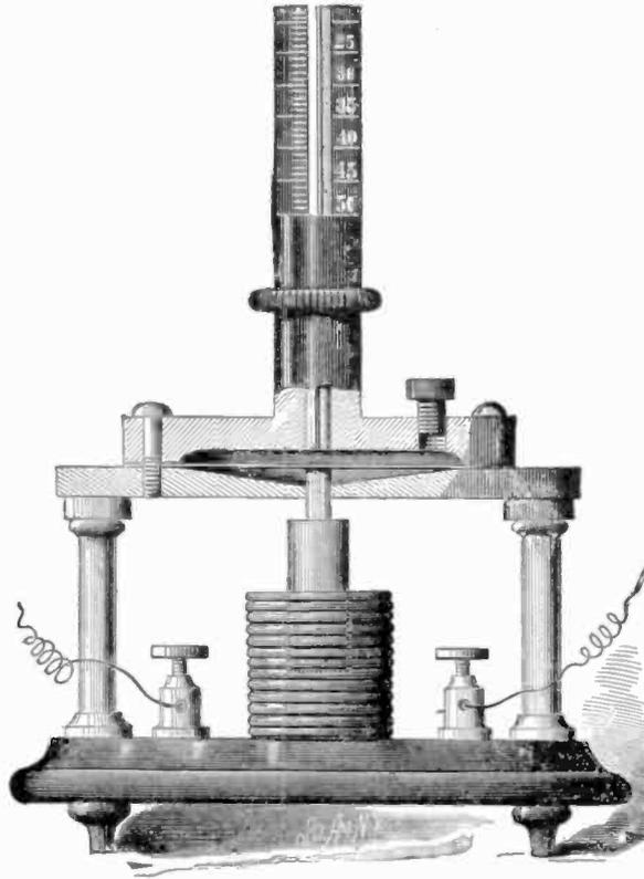
In crude ammeter above, current flowing through coil pulls a movable core down, activating a diaphragm and causing mercury in tube to fall. Device below is expansion voltmeter; it depends on linear expansion of a thin platinum wire when voltage is applied. Wire is coupled to pointer in front of scale.
