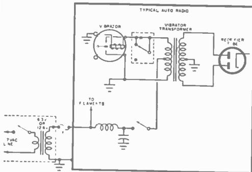
a filament transformer with a voltage equal to the radio's original working voltage—6 or 12 volts—and with a current rating that equals or exceeds the radio's battery drain current (usually 6 or 7 amperes for a 6-volt set, half that for a 12-volt set). Connect
