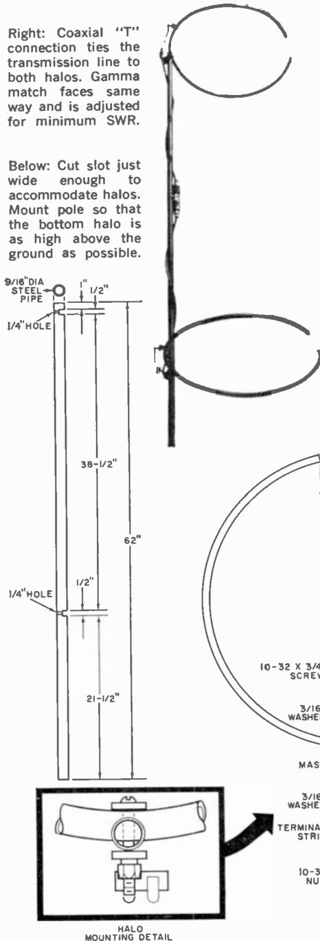
**H**ALO ANTENNAS are like  $\frac{1}{2}$ -wavelength dipoles in many ways. They are cut to the same size, they are horizontally polarized, and they can be stacked for additional gain. However, the bidirectional characteristic of the dipole changes to an omnidirectional pattern when the dipole is curved to form a halo.
