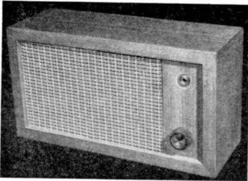
Small speaker system forms housing for Sleep-O-Mat; loudness control *R7* and phono jack *J1* are mounted on front. Long narrow chassis fits in back of speakers (photo below). Tubes *V1* and *V2* are at left, power and output transformers at right. Chassis size depends on the enclosure selected for the unit.
