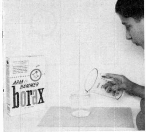
The first step in making a chemical rectifier is to dissolve Borax in water—peanut butter jar is used.
