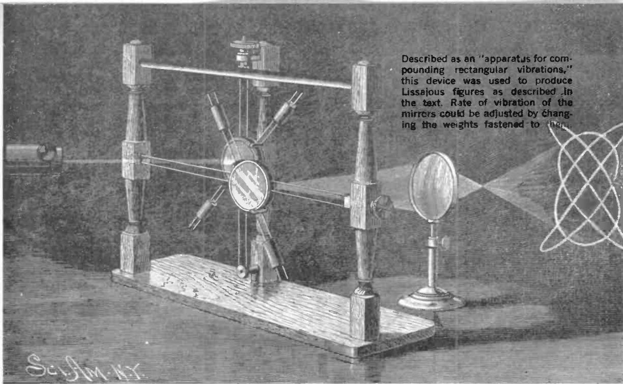
Described as an "apparatus for compounding rectangular vibrations," this device was used to produce Lissajous figures as described in the text. Rate of vibration of the mirrors could be adjusted by changing the weights fastened to them.
