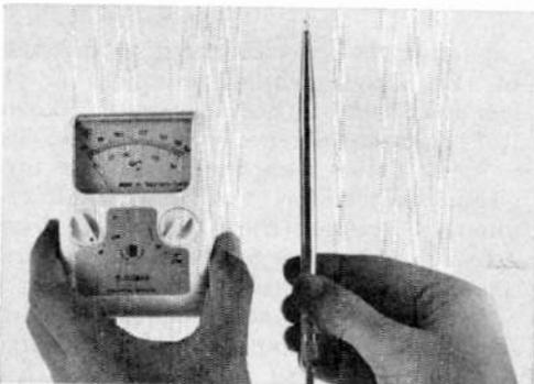
**A** NEW application has been found for the temperature-sensitive thermistor, a semiconductor. Braun Electronic, a West German firm, has put it to work in a medical thermometer that accurately gauges a patient's temperature in seconds. Named "Tastomed," the device has a probe which is held under the patient's tongue, and a meter calibrated in Centigrade and Fahrenheit. U.S. representatives: Electro-Physical Instruments of Ogdensburg, N.Y.
