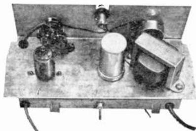
Chassis shown is made from one piece of sheet metal. Separate pan and front piece could be employed. Tabs on apron act as backstops.
