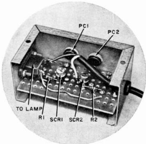
The two SCR's can be connected directly to the board and soldered into the circuit, or plugged into appropriate sockets. Avoid overheating the SCR's when soldering.
