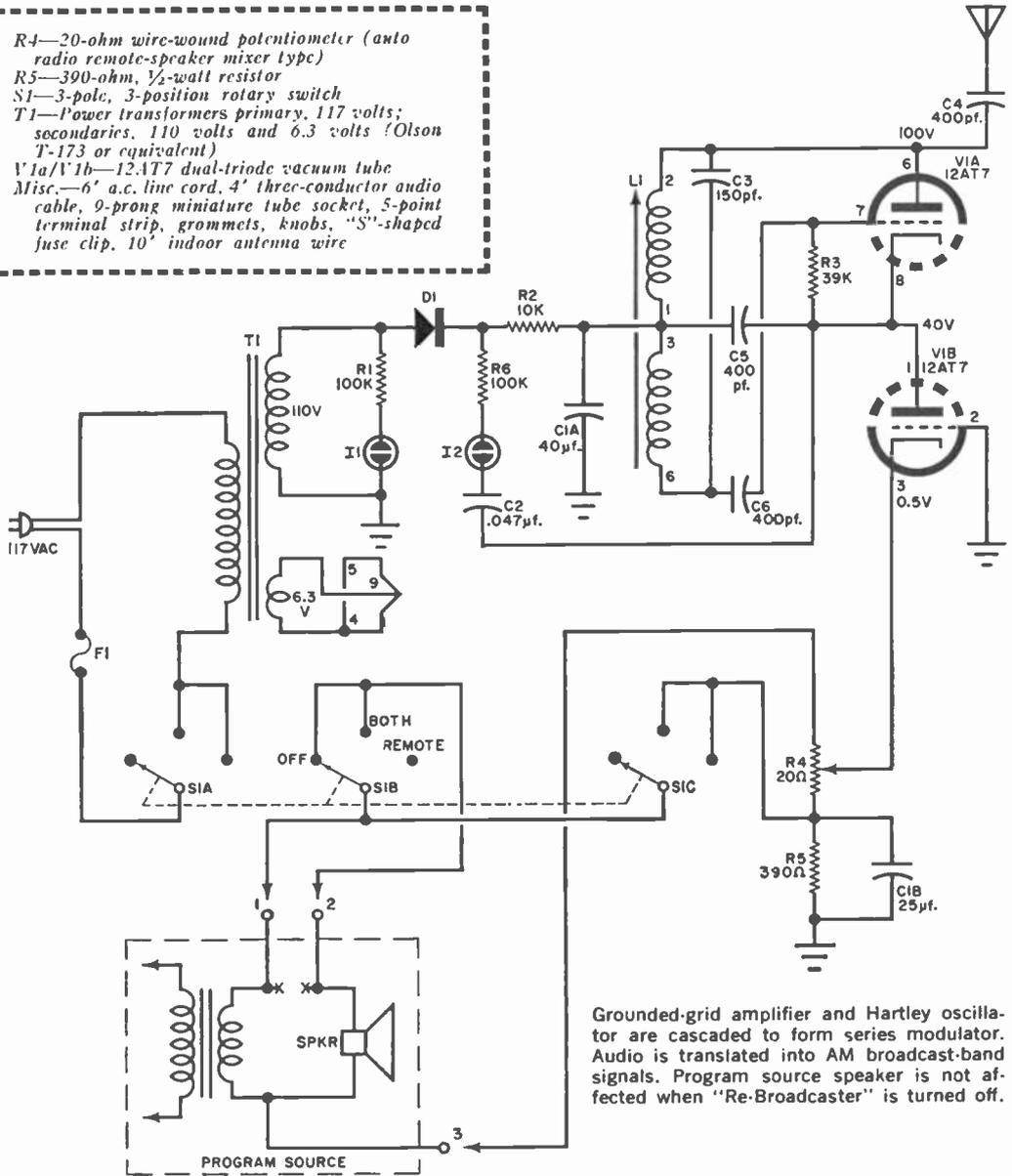
Grounded-grid amplifier and Hartley oscillator are cascaded to form series modulator. Audio is translated into AM broadcast-band signals. Program source speaker is not affected when "Re-Broadcaster" is turned off.
