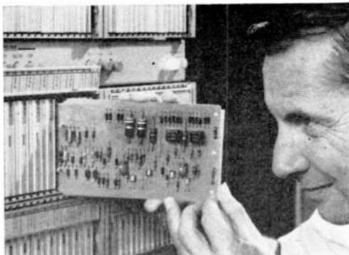
Heart of new telephone switching system is the "central control." Thousands of readily replaceable circuit boards have been specially developed to speed maintenance.
