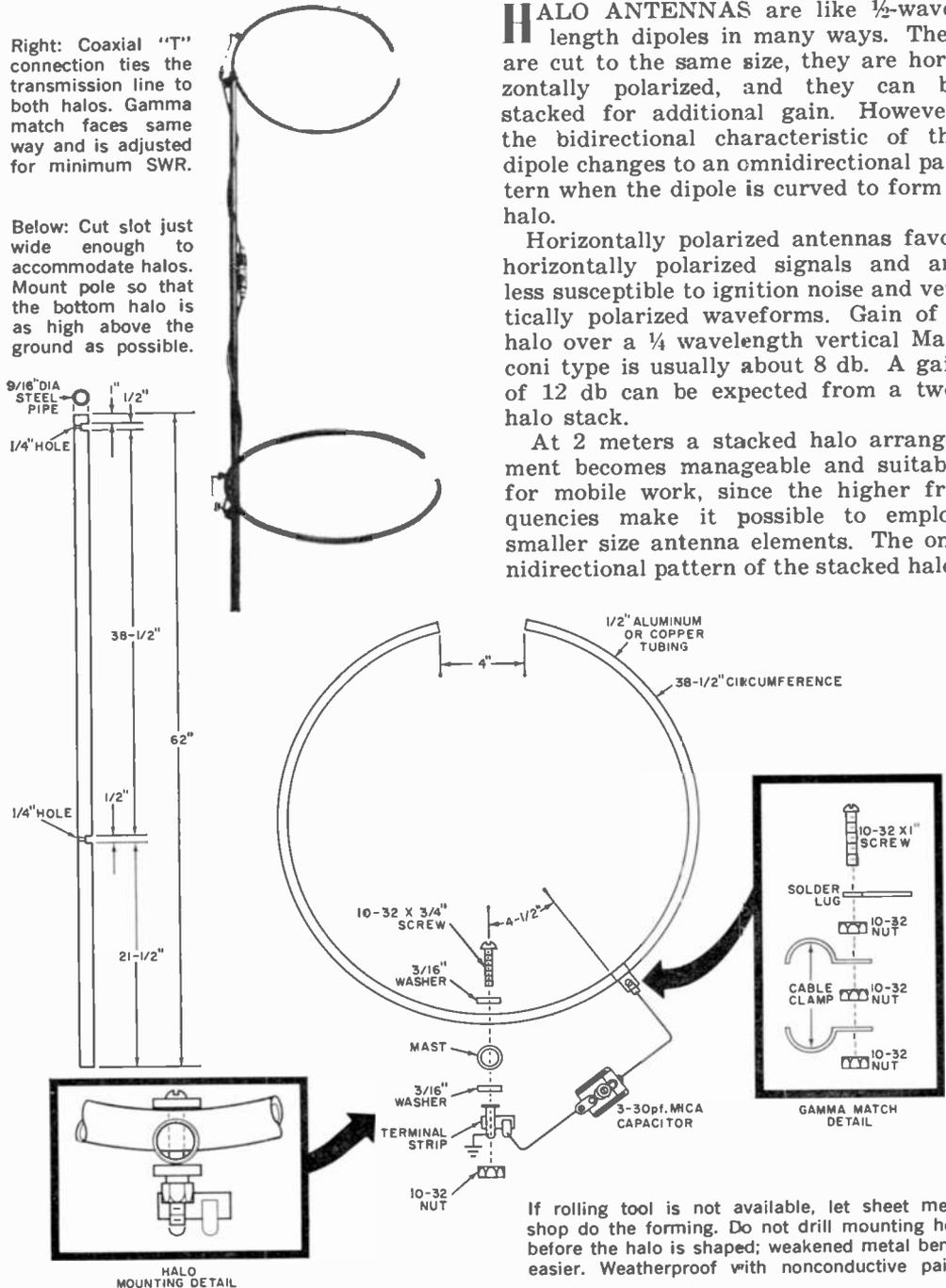
**H**ALO ANTENNAS are like  $\frac{1}{2}$ -wavelength dipoles in many ways. They are cut to the same size, they are horizontally polarized, and they can be stacked for additional gain. However, the bidirectional characteristic of the dipole changes to an omnidirectional pattern when the dipole is curved to form a halo.
