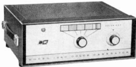
and to align the color demodulators. Suitable for operation on channels 3, 4 or 5, it connects directly to the TV antenna terminals. Its r.f. output is more than 5000  $\mu$ v. The unit is power-transformer-operated and line-isolated to prevent shock hazards. Price, \$134.95.
