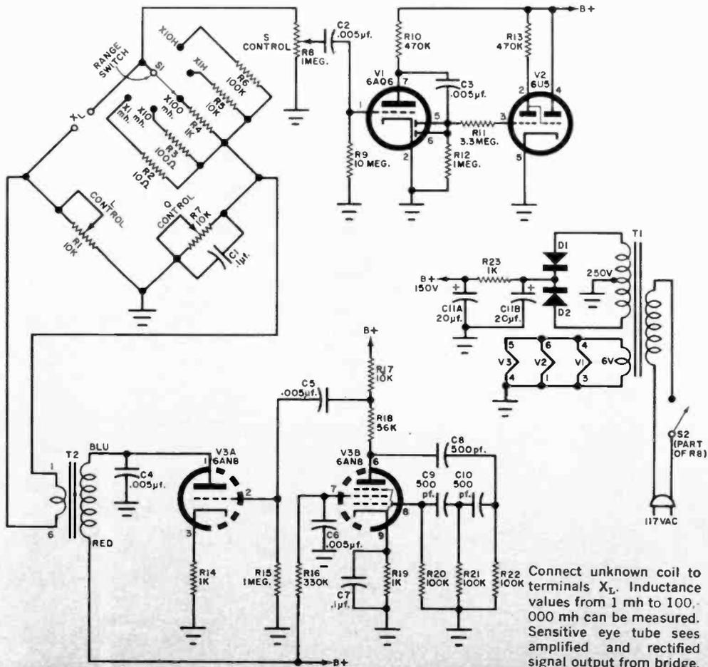
Connect unknown coil to terminals  $X_L$ . Inductance values from 1 mh to 100,000 mh can be measured. Sensitive eye tube sees amplified and rectified signal output from bridge.
