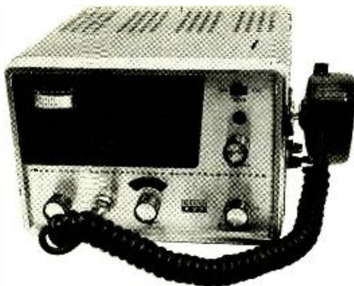
Above: an external view of the 777, which measures  $6" \times 8\frac{1}{2}" \times 10"$ . Below: top-of-chassis arrangement; factory-assembled transmitter is on left subchassis.
