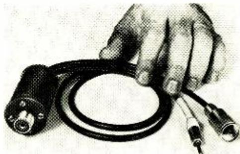
To use a CB antenna for AM broadcast-band radio reception, a coupler must be installed (it takes only two minutes) to keep the signals separate. The coupler shown here is manufactured by B & K/Mark (division of Dynascan Corp.) as model number CBC-1.
