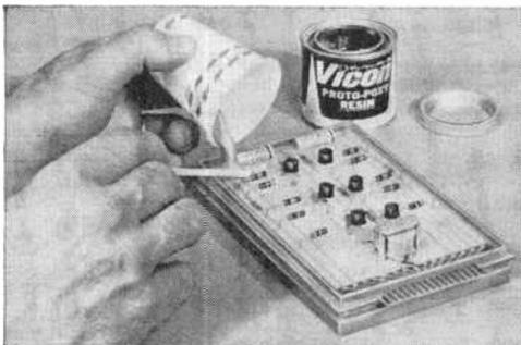
Fig. 15. This "Proto-Board" circuit can be fitted with a frame as shown and covered with a special epoxy resin compound.
