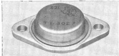
without any heat sink whatever, it could run at a 2-watt continuous power level.
