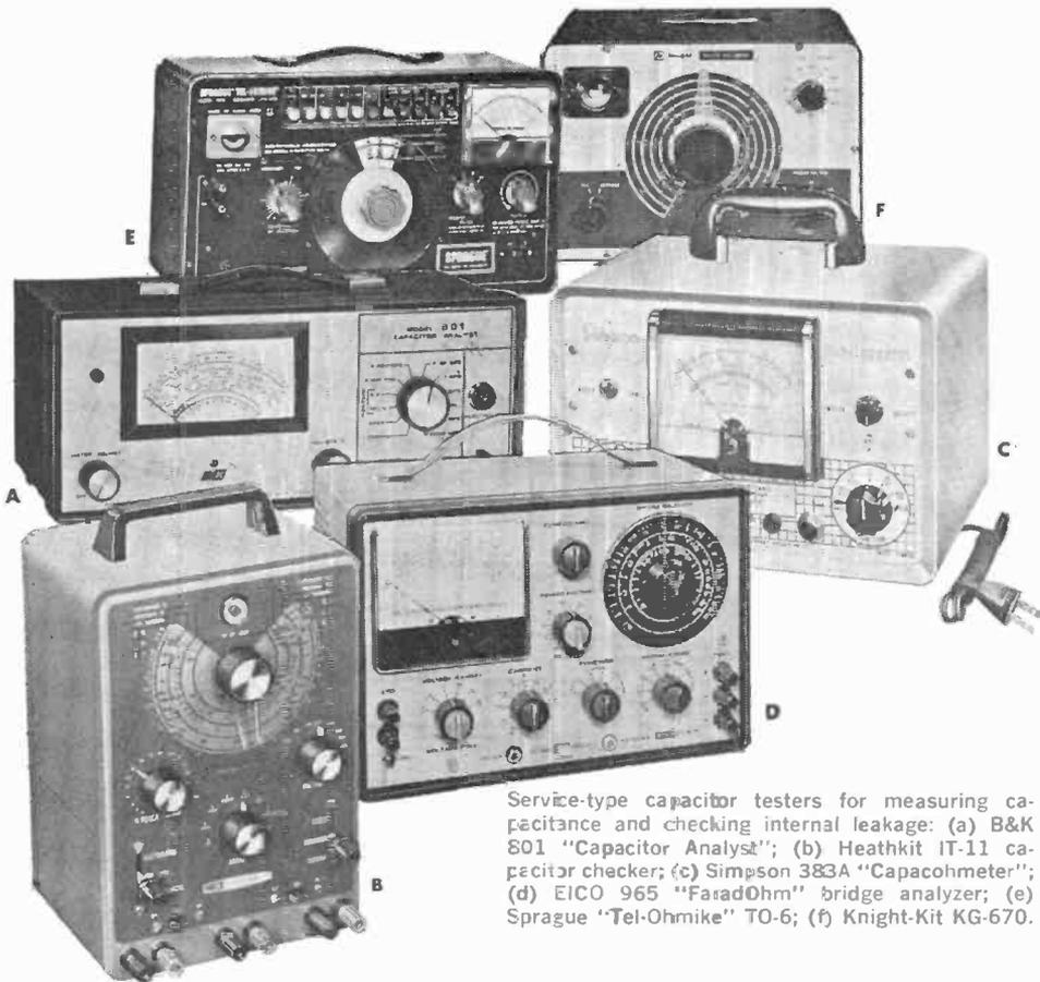
Service-type capacitor testers for measuring capacitance and checking internal leakage: (a) B&K 801 "Capacitor Analyst"; (b) Heathkit IT-11 capacitor checker; (c) Simpson 383A "Capacohmeter"; (d) EICO 965 "FaradOhm" bridge analyzer; (e) Sprague "Tel-Ohmike" TO-6; (f) Knight-Kit KG-670.
