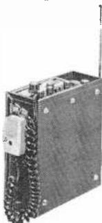
This 40" telescoping portable antenna is ideal for field operation.
