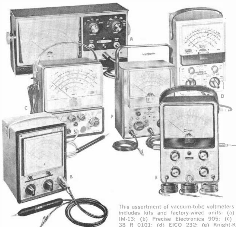
This assortment of vacuum-tube voltmeters (VTVM's) includes kits and factory-wired units: (a) Heathkit IM-13; (b) Precise Electronics 905; (c) Lafayette 38 R 0101; (d) EICO 232; (e) Knight-Kit (Allied Radio) KG-620; (f) RCA "VoltOhmyst" WV-77E.
