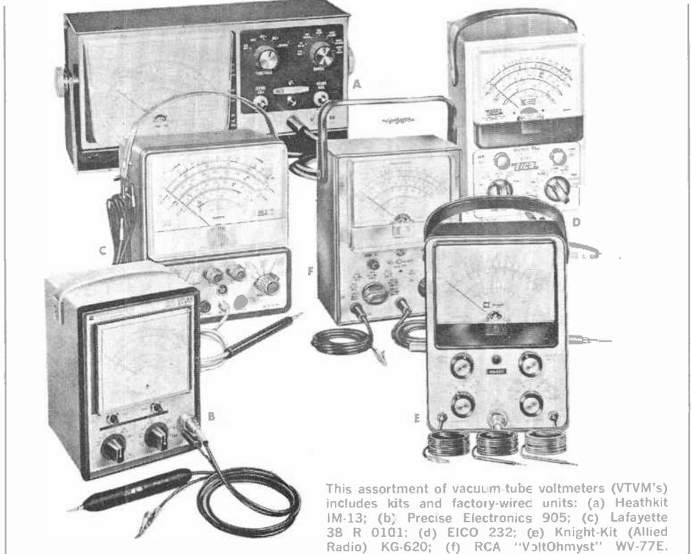
This assortment of vacuum-tube voltmeters (VTVM's) includes kits and factory-wired units: (a) Heathkit IM-13; (b) Precise Electronics 905; (c) Lafayette 38 R 0101; (d) EICO 232; (e) Knight-Kit (Allied Radio) KG-620; (f) RCA "VoltOhmyst" WV-77E.
