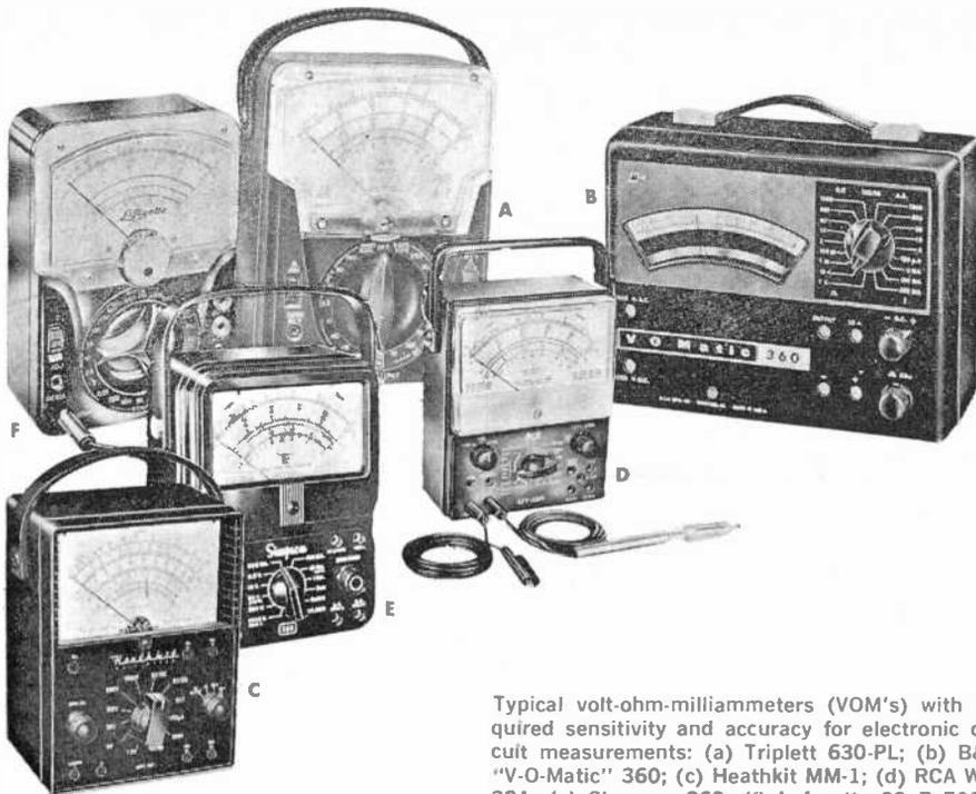
Typical volt-ohm-milliammeters (VOM's) with required sensitivity and accuracy for electronic circuit measurements: (a) Triplet 630-PL; (b) B&K "V-O-Matic" 360; (c) Heathkit MM-1; (d) RCA WV-38A; (e) Simpson 260; (f) Lafayette 99 R 5004.
