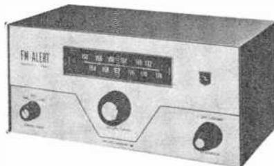
dial, it comes in two models—one covering 152-175 mc., the other 30-50 mc. The "FM Alert" utilizes a quadrature detector and high-gain i.f. to provide clean, quiet reception over a wide range of signal strengths and modulation levels. Sensitivity is  $3\mu\text{v}$ . or less for squelch control and 10 db S/N. A separate matching speaker can be used either at the receiver or at a remote location.
