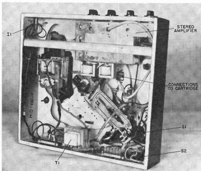
Solid-state stereo amplifier runs cool and is compact enough to fit into record changer base. Parts location is not critical, but adequate clearance for the changer mechanism must be provided. It's a good idea to run the changer through a cycle by hand in order to check clearance requirements.
