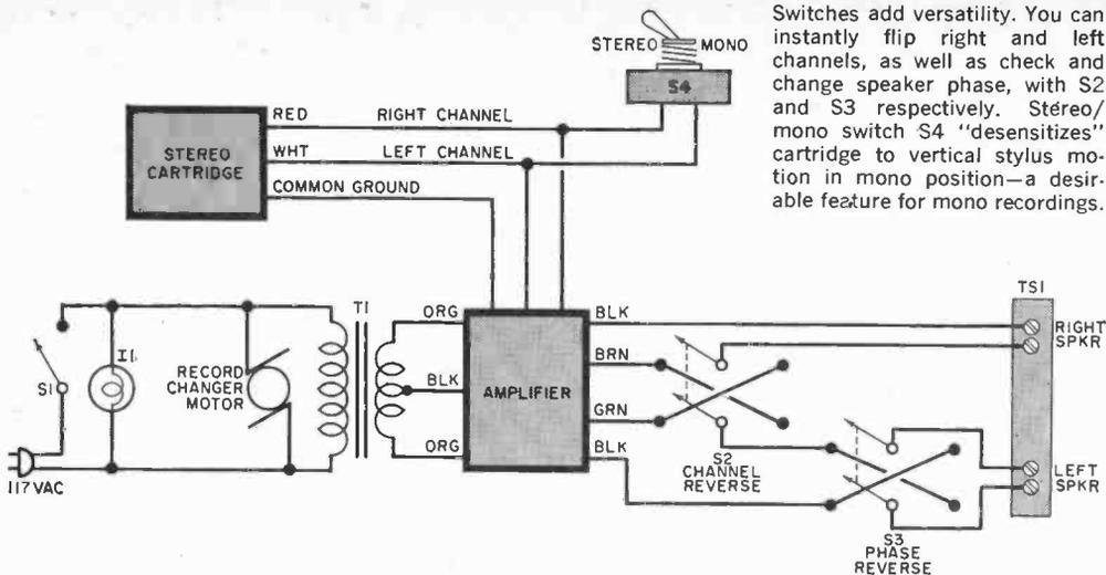
Switches add versatility. You can instantly flip right and left channels, as well as check and change speaker phase, with S2 and S3 respectively. Stereo/mono switch S4 "desensitizes" cartridge to vertical stylus motion in mono position—a desirable feature for mono recordings.
