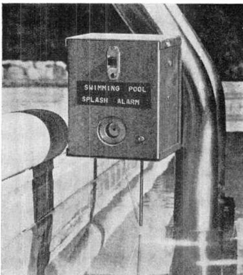
When installing the alarm, bend the probes close together and make tests to determine optimum separation. Best results will be obtained by installing the probes at the pool, with the alarm being remotely located at a convenient listening post.
