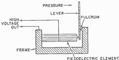
Fig. 1. Clevite Corporation's Spark Pump Igniter develops 20,000-volt sparks which can be used to ignite gasoline engines and gas-fired appliances.
