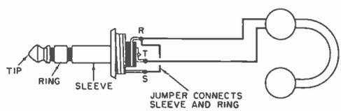
for use with a 2-conductor mono headset is to jump the plug's sleeve (S) and ring (R) connectors as shown. Solder the headset leads to the ring and lug tips (T). —Carl Dunant
