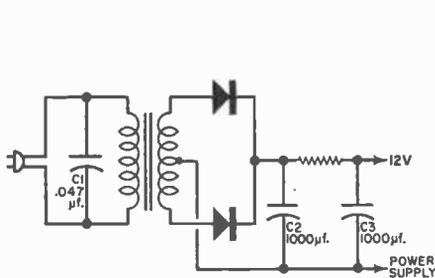
Large capacitors (C2, C3) are needed to smooth out ripple voltage from rectifiers—values ranging from 20  $\mu\text{f.}$  and up are typical. Electrolytic type capacitors, because of their relatively small size and low cost per microfarad are used here. Capacitor C1 is not always used, but it does reduce r.f. and other hash on the power line; its value, not critical, is usually quite small.
