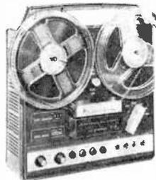
preset button. Frequency response is  $\pm 3 \text{ db}$ , 40-15,000 hertz at  $7\frac{1}{2} \text{ in/s}$ ;  $\pm 3 \text{ db}$ , 40-10,000 hertz at  $3\frac{3}{4} \text{ in/s}$ . The RK-815 is mounted in a textured solid vinyl case.
