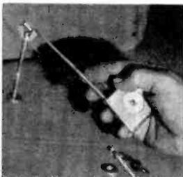
masking tape—sticky side out—around the magnet. The flexibility and slimness of the steel tape enables the magnet to be positioned in extremely close quarters to pick up the fallen object.
