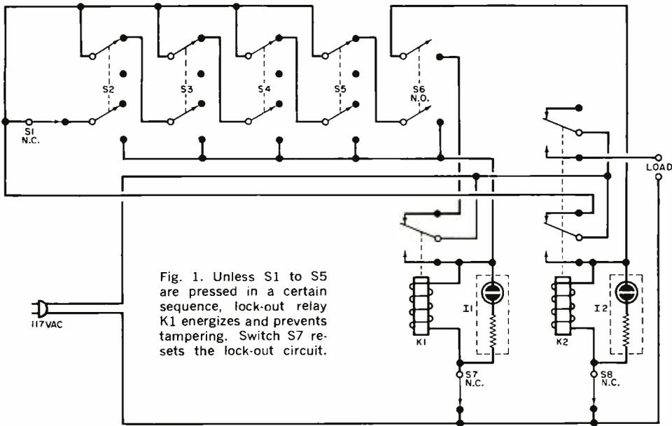
main depressed until the entire six-switch sequence is complete. A lock picker would naturally assume that all he has to do is press a button, release it, and go on to press another. Not so. If he presses any of the remaining five buttons without holding the first one down, the lock-out circuit will come into play as if he had selected the wrong one on the first try—even if the second push
