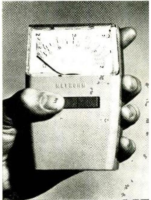
Fig. 3. Newly developed, this transistorized insulation tester by Edgcombe Peebles Ltd. (Surrey, England), can also double as a low-resistance continuity tester, or as a general-purpose voltmeter.
