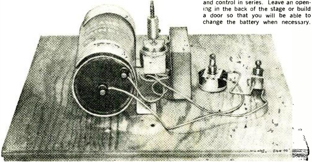
Connect the battery, motor, switch, and control in series. Leave an opening in the back of the stage or build a door so that you will be able to change the battery when necessary.
