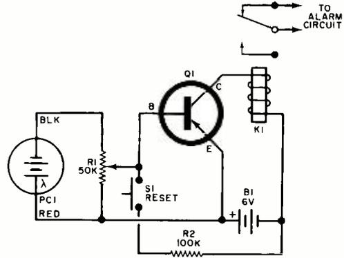
Fig. 1. In this intruder alarm circuit submitted by reader Eugene Richardson, relay *K1* is released to activate the alarm when an intruder interrupts the light beam focused on *PC1*. The alarm stays on until reset switch *S1* is pressed to turn it off.
