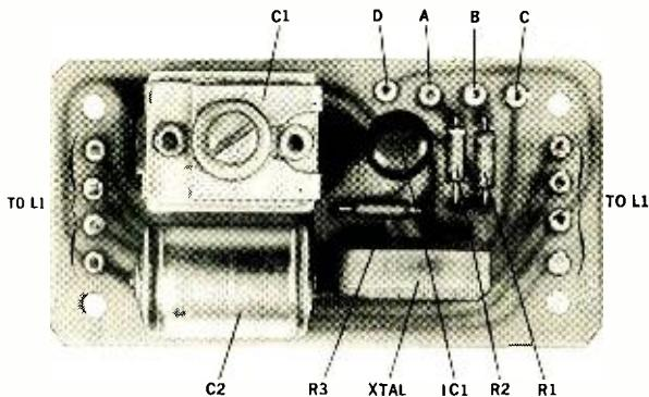
Fig. 11. Components are mounted on transmitter board. Note that pin numbers on IC1 run counterclockwise when you're looking at the top of the component.
