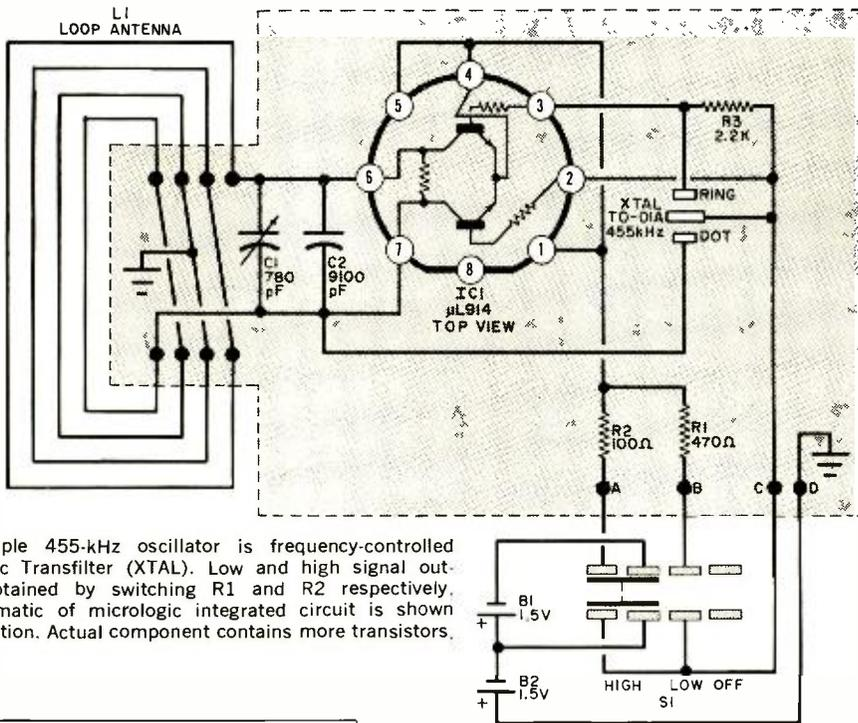
Fig. 1. Simple 455-kHz oscillator is frequency-controlled by a ceramic Transfilter (XTAL). Low and high signal outputs are obtained by switching R1 and R2 respectively. Partial schematic of micrologic integrated circuit is shown for simplification. Actual component contains more transistors.
