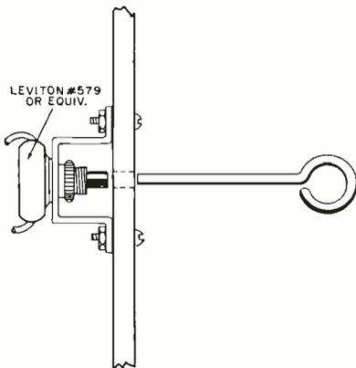
connect the power, insert a metal or plastic rod in the hole and press. To restore the power, press again. The rod is the key to your lock, so bend one end of it into a closed loop and carry it around on your key chain.
