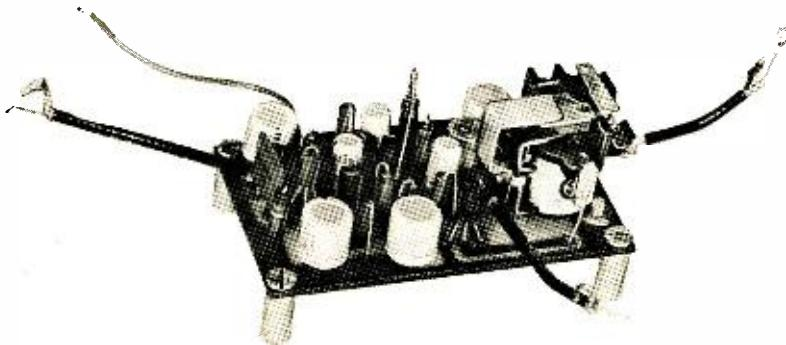
Fig. 5. Completed board assembly. Note use of shielded cable for input and output connections. Stand-offs are used to mount the board in the cabinet and to provide clearance. Components are stood on end.
