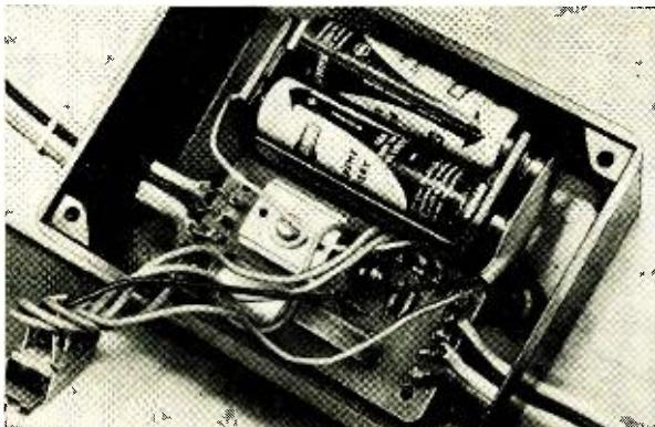
10. Mount the components as shown in Figs. 11 and 13. Do not substitute capacitors; those called for have the proper "Q" and tolerance. The transformers and chokes are held in place by their leads. After the initial checkout, you can further secure them with a dab of coil dope.
