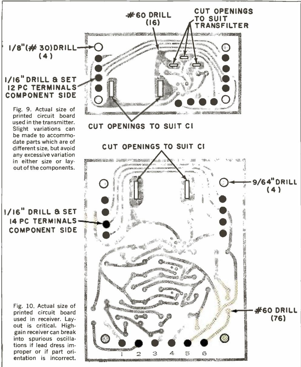
Fig. 9. Actual size of printed circuit board used in the transmitter. Slight variations can be made to accommodate parts which are of different size, but avoid any excessive variation in either size or layout of the components.
