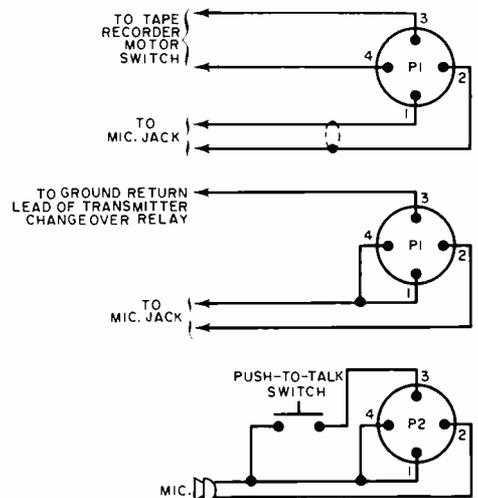
Fig. 2. Inputs *J1* and *J2* are in parallel, and can be used interchangeably, but the plugs must be wired in accordance with their specific function. Plug *P1*, top, serves as an output connector from the Trans-Vox, and is designed for a tape recorder. Plug *P1*, center, is for connection to a transmitter. Input plug *P2* can be wired as shown; if your microphone does not have a push-to-talk switch on it, simply omit the connections to pins 3 and 4 on *P2*.
