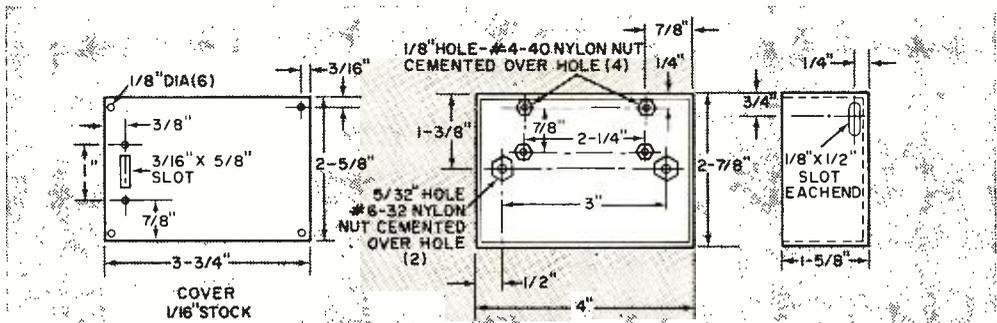
Fig. 7. Use a small plastic box to house the transmitter. Do not employ any more metal hardware than is absolutely necessary. A metal case will distort field pattern uniformity.
