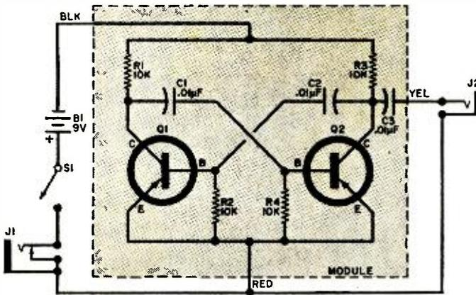
Parts inside the preassembled module are arranged to form a multivibrator oscillator circuit. Oscillator frequency is determined by C1, C2, R2 and R4.
