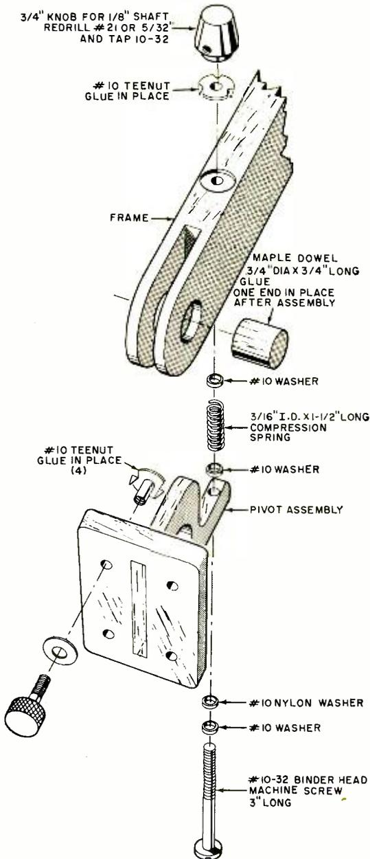
8, but do this carefully to avoid damage. A rotary file will save you time on the two big holes in the receiver. Glue nylon nuts over the holes in the case, as indicated, and keep the threads and the hole clear. Insert a metal screw while the gluing job is in progress, and then
