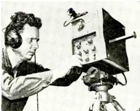
**WHO GOES THERE?**—The AN/PPS-6 one-man portable radar set built by the General Instrument Corp. detects a moving vehicle at distances up to 2 miles, a walking man up to 1 mile in pitch darkness.
