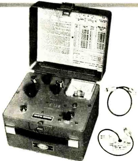
■ *Panel Controls* — Channel selector, 24 positions • "Hi-Lo" frequency adjust • RF level control • Modulation set • Power • Meter calibration adjust • Function selector, 7 positions • Modulation • RF • Deviation • Calibration • Battery Test "A" • Battery Test "B" • Battery Test "C".
