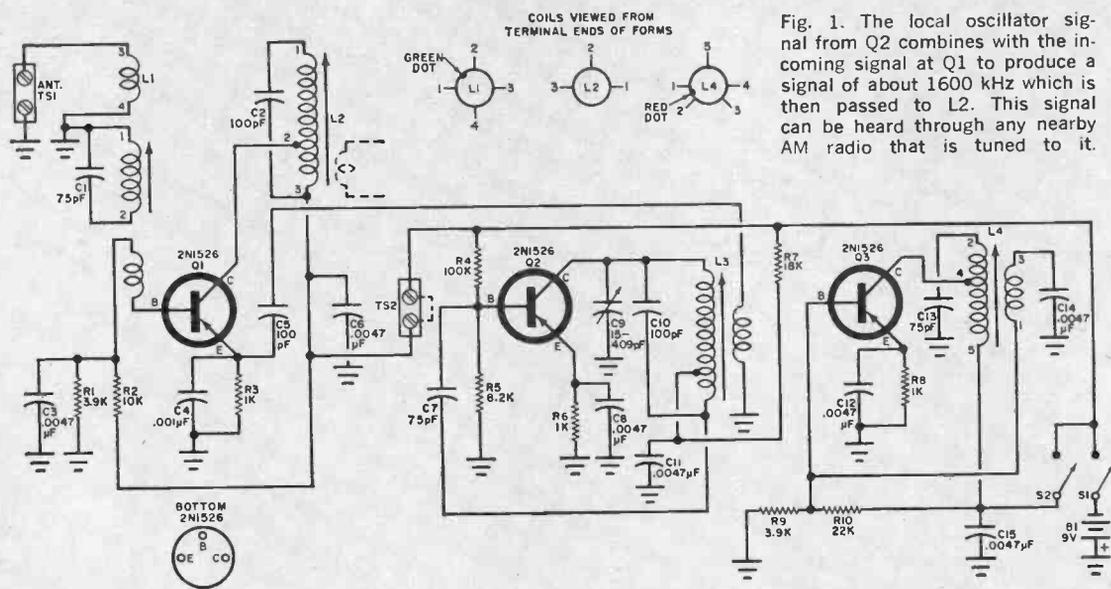
Fig. 1. The local oscillator signal from  $Q2$  combines with the incoming signal at  $Q1$  to produce a signal of about 1600 kHz which is then passed to  $L2$ . This signal can be heard through any nearby AM radio that is tuned to it.
