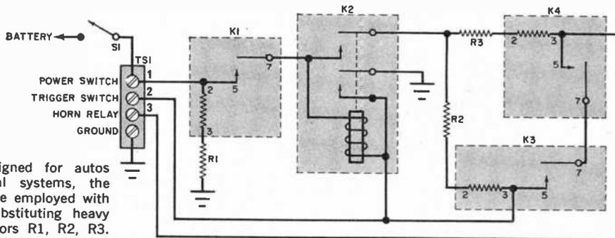
Fig. 1. Although designed for autos with 12-volt electrical systems, the "Auto Sentinel" can be employed with 6-volt systems by substituting heavy jumper wire for resistors R1, R2, R3.
