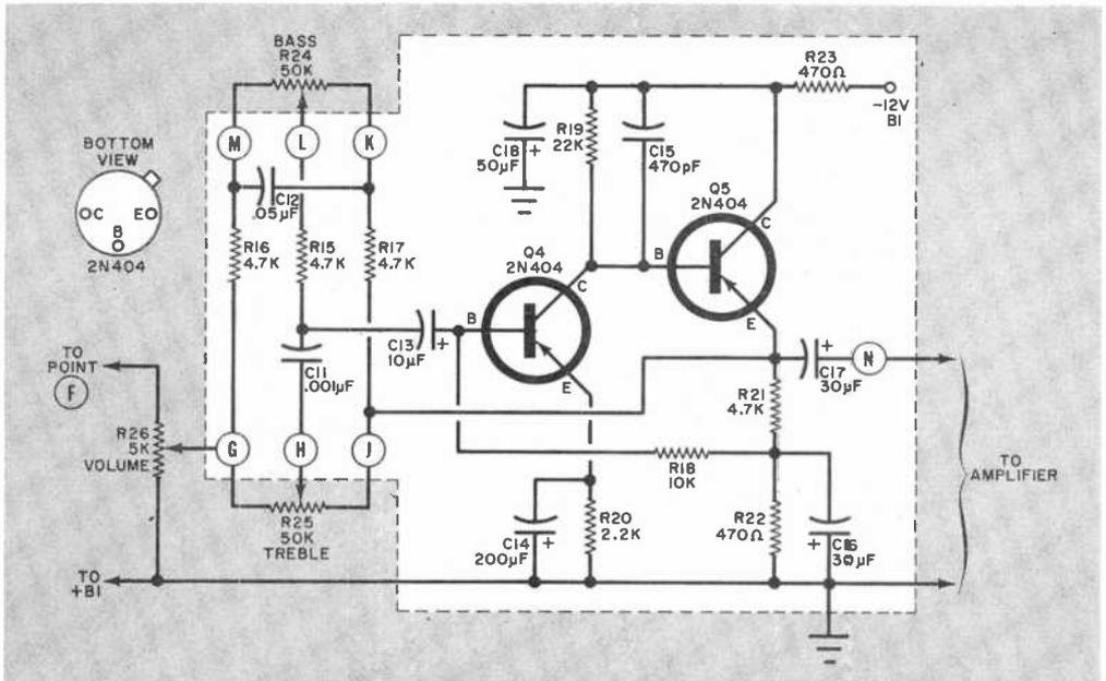
Fig. 2. Circuitry important to the tone controls of the stereo preamp is etched in two printed circuit boards. As in the diagram on the facing page, points G,H,J,K,L,M, and N are connections to jacks, switches, and front panel controls.
