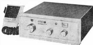
precision series-mode fundamental crystals results in superior transmit and receive stability (crystals are supplied for 23 channels). Sensitivity is less than 0.5  $\mu$ V for 10 dB S/N ratio, squelch adjustable to 1  $\mu$ V. The unit operates from a 12-volt d.c. negative-or-positive-ground supply, or from 117 volts a.c. with an optional power supply. Special feature: a flick of a switch converts the NOVA-23 to a 3.5-watt p.a. system.
