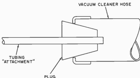
through the center of the plug just large enough to allow the tubing to fit snugly. Push the tubing into the hole, and apply a daub of cement to hold it in place. Then push the plug into the end of the vacuum cleaner hose. You can use the adapter either to blow or draw air.
