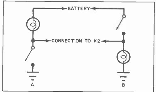
Fig. 4. If a mercury switch is used for the trunk light and it is wired as shown in B, rewire it to conform to the configuration shown in A at left.
