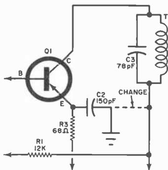
best way to do this is to use the hole in the chassis formerly used to ground *C4*. It may be necessary to add a short extension lead to *C2*. When you make this modest circuit change, your squeal should vanish.
