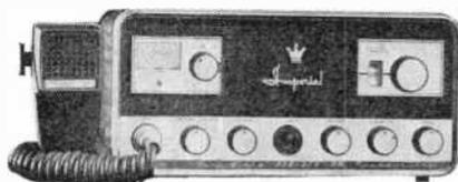
three different modes in each of the 23 CB channels, and it can transmit on two modes within each channel. A simple front panel control enables you to select the upper sideband, lower sideband, or AM function on the receiver. For transmitting, you can use the double sideband with reduced carrier facility for conventional AM signals, or transmit on both sidebands simultaneously without carrier. The Imperial operates on 117 volts a.c., or 12 volts d.c.
