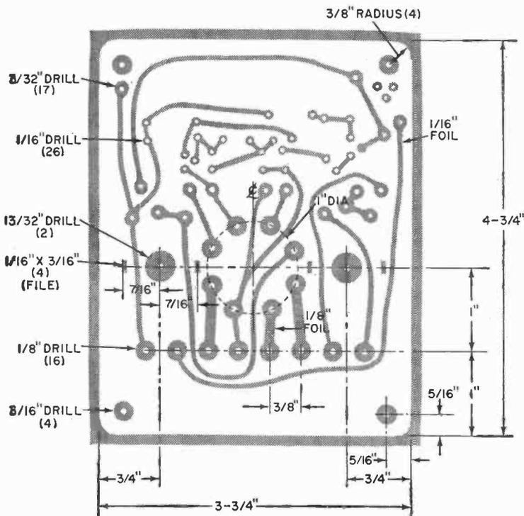
Fig. 2. A printed circuit board can be etched following the outlines shown in this drawing. Use of this outline should be predicated on the physical size of capacitor C1, location of the terminals for the octal socket to hold K1, and whether or not the builder uses twist-tab potentiometers for R11 and R12. Point-to-point wiring can be used in place of a printed circuit without encountering any problems.
