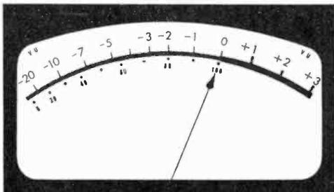
the difference between the vu and the dBm and states that the two should not be used interchangeably. It's true, too, that a vu meter must have a certain specified ballistic characteristic to read out average levels in a waveform, and to keep it from responding to signal peaks. Your letter-head logo seemed so apropos to this discussion that we have reproduced it here.
