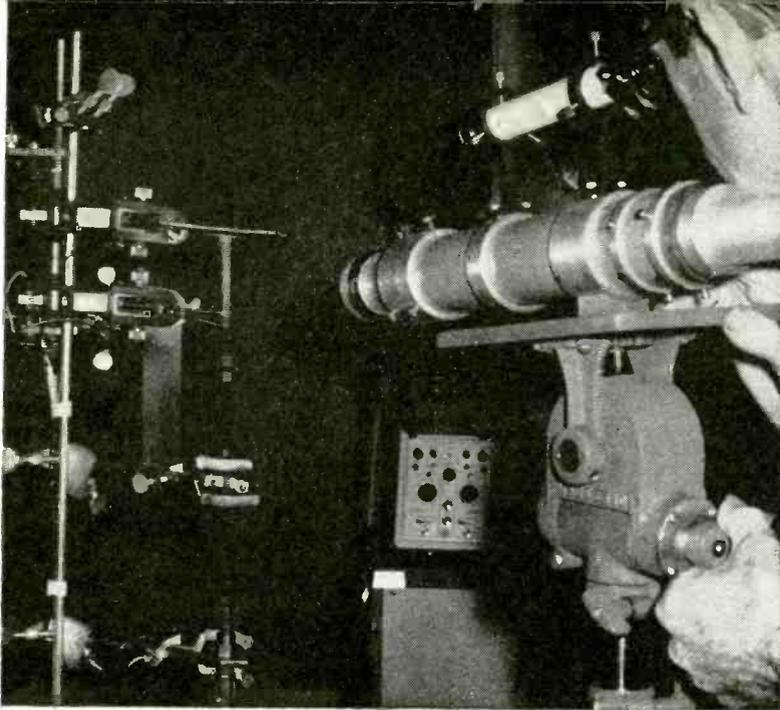
Because the welding torch flame is too small to support the low audio frequencies, a photomultiplier system "picks them out" and supplies them to a separate amplifier system. Overall frequency response is from a few cycles to well over 100 kHz at high sound level.
