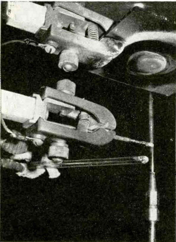
Electrical signals are fed in via two insulated alligator clamps while glass rod "seeds" the flame.
