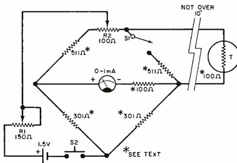
$\pm 1\%$  at  $25^\circ\text{C}$  can be used. All resistors are precision units (IRC 1% metal film) which can be obtained from most supply houses; they cost less than a dollar each.
