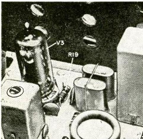
Resistor R19 is directly adjacent to tube V3, the first i.f. amplifier. After the overall conversion is completed, the GR-54 becomes a really "hot" set.
