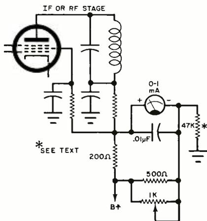
stages, or use a second or third i.f. stage. The pot zeros the meter with no signal.
