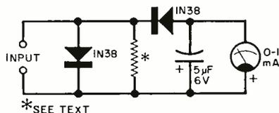
stant signal (not null), the meter needle will remain steady, its deflection being proportional to the amount of signal available. The resistor across the plug should match the output impedance of the headphone jack, which can be 2000, 4000, or 8000 ohms.
