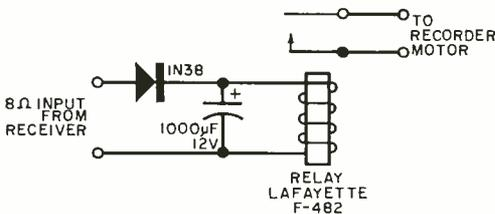
one second after the speech ceases. The relay contacts are connected to the recorder motor circuit. Adjust the a.f. output of the receiver (on signal) so that the relay will close and turn on the recorder motor. If you experience too short a delay, increase the size of the capacitor to 2000  $\mu$ F.
