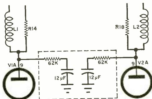
and a.c. signals, and a pronounced sloping of low-frequency square waves. The compensation network shown here will compensate for low-frequency losses in the Model 460. For best results, you might have to allow a slight variation in the value of the resistors for individual tubes. The easiest way to install the capacitors is to connect one lead of each to a ground lug held by terminal board TB-16, and the other lead directly to pin 9 on the respective tube sockets. —Donald Stauffer
