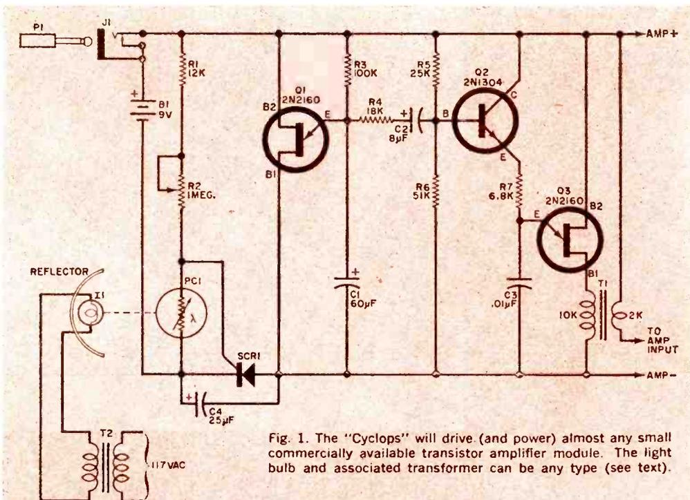
Fig. 1. The "Cyclops" will drive (and power) almost any small commercially available transistor amplifier module. The light bulb and associated transformer can be any type (see text).
