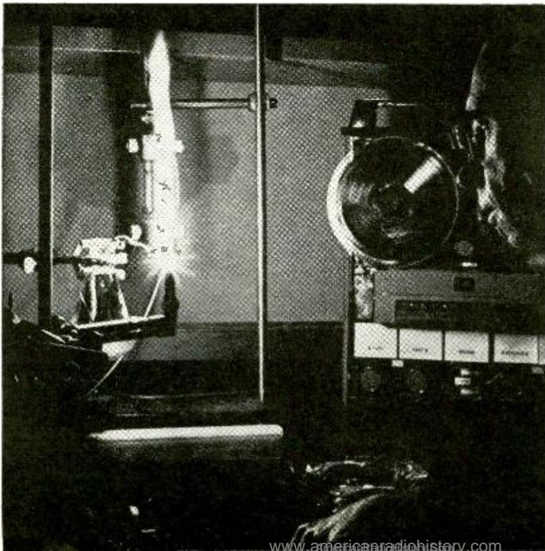
sizable pluses of the flame speaker. Its frequency response range is three to four times that of any known mechanical speaker—and future tests, far beyond the audio spectrum, may well show even higher response. Where, for example, even the best and costliest of diaphragm-type speakers can reproduce, at their highest range, only about 30,000 Hz (at best, about 12,000 Hz above what even the most acute human ear can hear), the flame speaker has shown it can reproduce *at least* 100,000 Hz.
