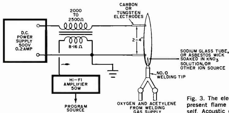
Fig. 3. The electrical arrangement of the present flame amplifier is simplicity itself. Acoustic output is omnidirectional.
