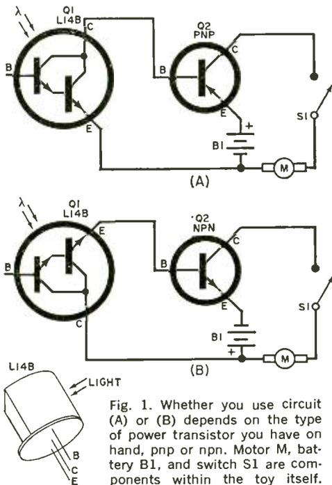
Fig. 1. Whether you use circuit (A) or (B) depends on the type of power transistor you have on hand, pnp or npn. Motor M, battery B1, and switch S1 are components within the toy itself.
