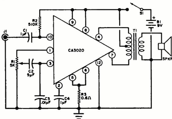
Fig. 2. This 500-mW audio amplifier is one of many circuits that can be made with RCA's QK2200 kit.
