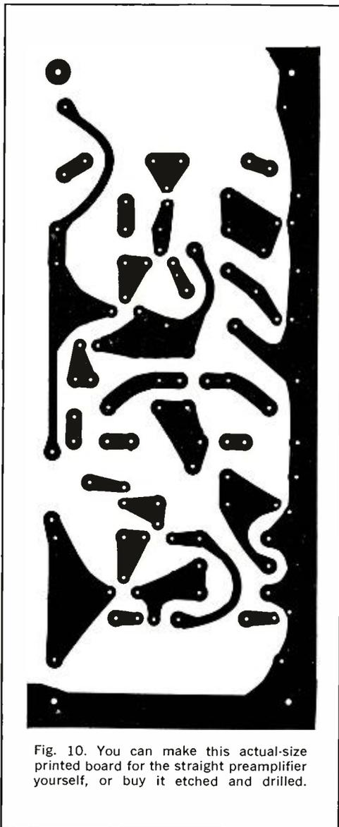
Fig. 10. You can make this actual-size printed board for the straight preamplifier yourself, or buy it etched and drilled.
