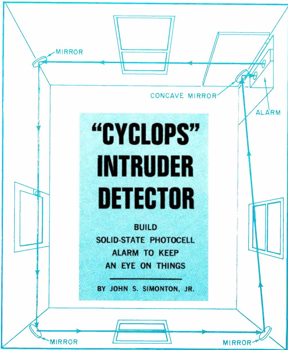
**H**ERE IS a little unit that is about as useful as another pair of eyes when you want to protect an area from intruders. If anyone, or anything, crosses an invisible line formed by a beam of light, an alarm sounds and does not turn off even though the intruder backs away from the line. The only way to shut off the “Cyclops Intruder Detector” is to use a special “key” that will be in your possession.
