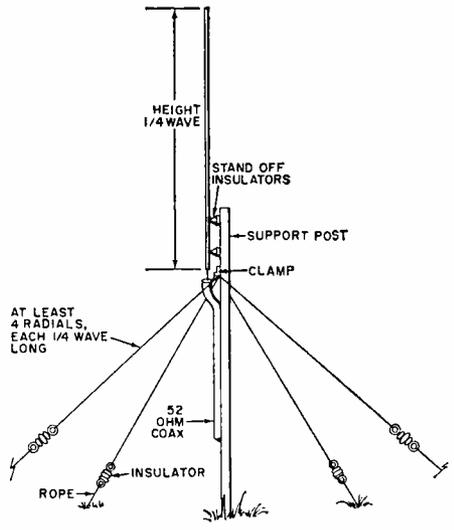
**T**HE ground-plane antenna at left is a logical choice where space is at a premium and if you want to work DX. It has a low radiation angle, can be mounted in the air or on the ground, and can be fed with coax. Its disadvantages are the need for a good radial system and the fact that it is generally a single-band affair with a tendency to cause TVI and broadcast interference.
