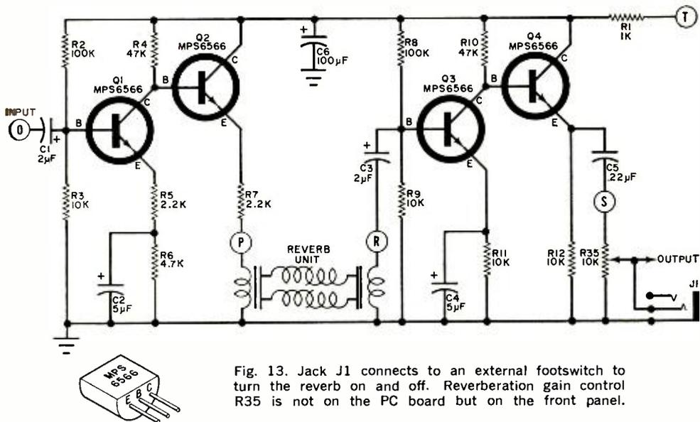
Fig. 13. Jack J1 connects to an external footswitch to turn the reverb on and off. Reverberation gain control R35 is not on the PC board but on the front panel.
