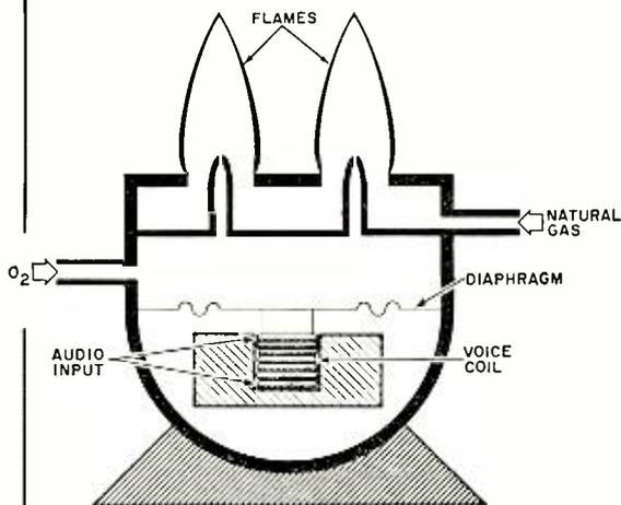
Fig. 2. Variation of mechanical flame modulator provided a louder sound and better audio quality.
