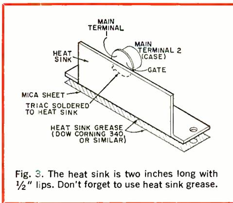
Fig. 3. The heat sink is two inches long with 1/2" lips. Don't forget to use heat sink grease.
