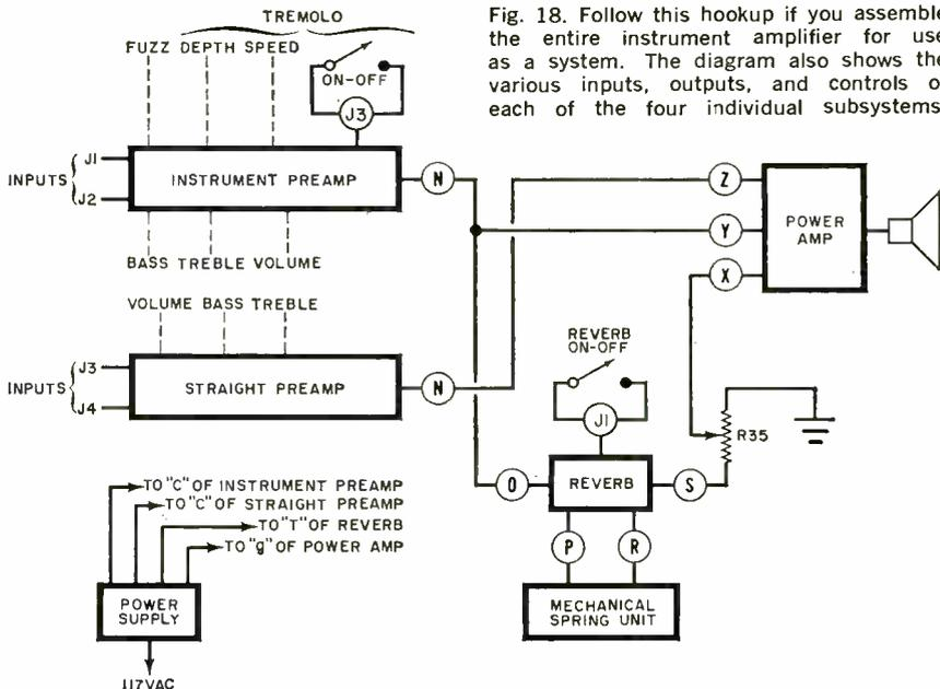
Fig. 18. Follow this hookup if you assemble the entire instrument amplifier for use as a system. The diagram also shows the various inputs, outputs, and controls of each of the four individual subsystems.
