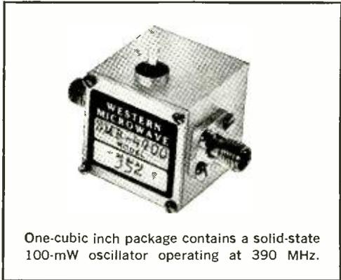
One-cubic inch package contains a solid-state 100-mW oscillator operating at 390 MHz.
