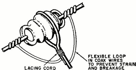
**T**O prevent the transmission line from breaking away from the antenna elements, it should be secured to the center insulator as shown here. Place the transmission line into one of the insulator's depressions, bend the line over double, and tie it securely in place with lacing cord.
