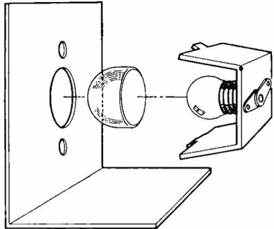
ceiver. Remove the #47 lamps, and replace them with #51 lamps. Then place colored dome-type lenses (for example, red for main tuning and green for bandspread) over the lamps, and replace the lamp holder on its bracket. —Gary Hummell
