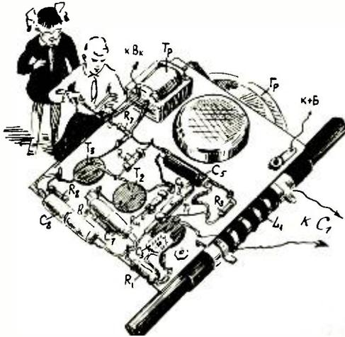
How-to articles, such as the one titled "Your First Transistor Receiver," featured in the Soviet magazine *RADIO*, are often lavishly illustrated with construction and component-orientation and placement drawings like this one.
