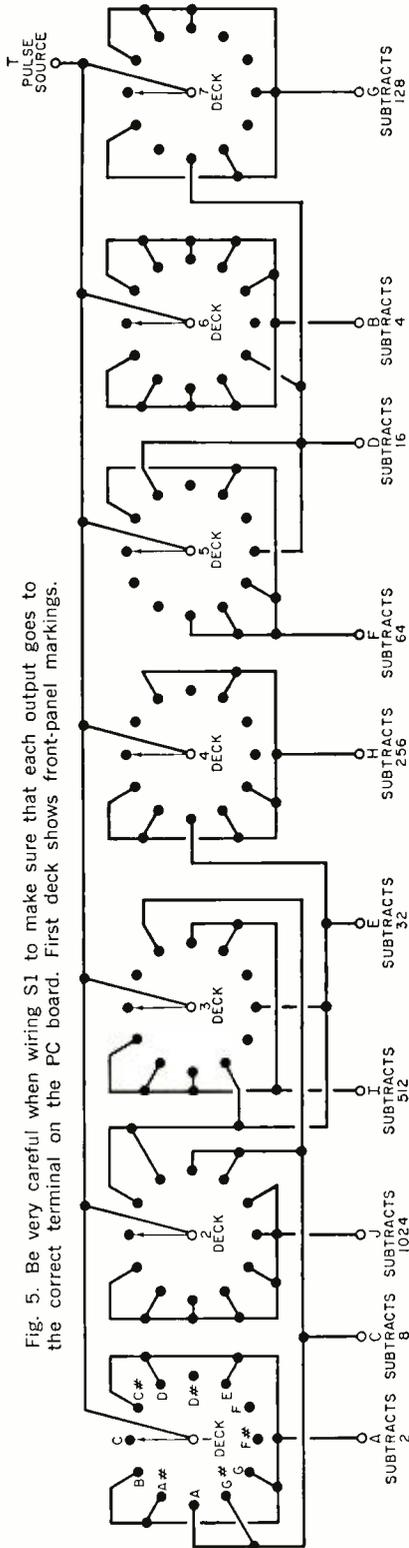
Fig. 5. Be very careful when wiring S1 to make sure that each output goes to the correct terminal on the PC board. First deck shows front-panel markings.
