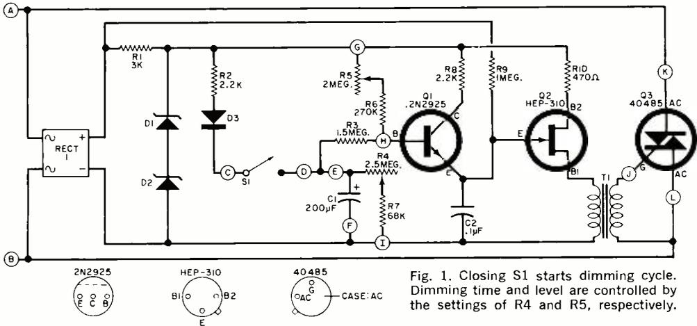
Fig. 1. Closing S1 starts dimming cycle. Dimming time and level are controlled by the settings of R4 and R5, respectively.
