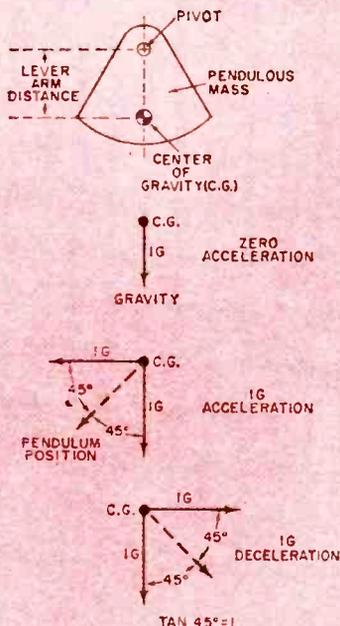
All forces acting on the pendulum mass act on its center of gravity, which is eccentric with respect to its pivot point. The lever arm is the distance from the pivot point to the center of gravity and transmits the force acting on the center of gravity to the pivot in a rotational manner.
