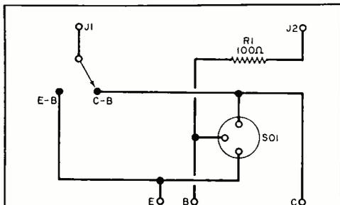
Containing only a resistor and a mounting socket, the circuit can be used to test pnp or npn transistors, in or out of use.
