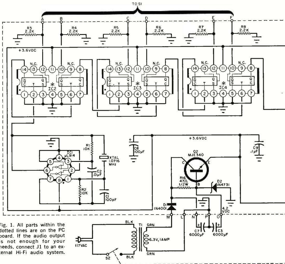
Fig. 1. All parts within the dotted lines are on the PC board. If the audio output is not enough for your needs, connect J1 to an external Hi-Fi audio system.
