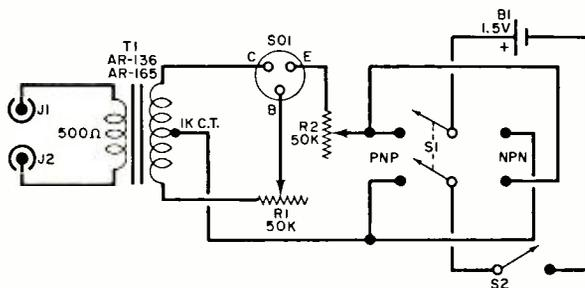
St., Arleta, Calif. 91311. Although it does not permit quantitative measurements, it can be used to find out if a transistor provides modest gain and will reject open, shorted, excessively leaky, and very low-gain units. The instrument could be quite valuable for quick checks of bargain or low-cost "surprise package" transistor purchases.
